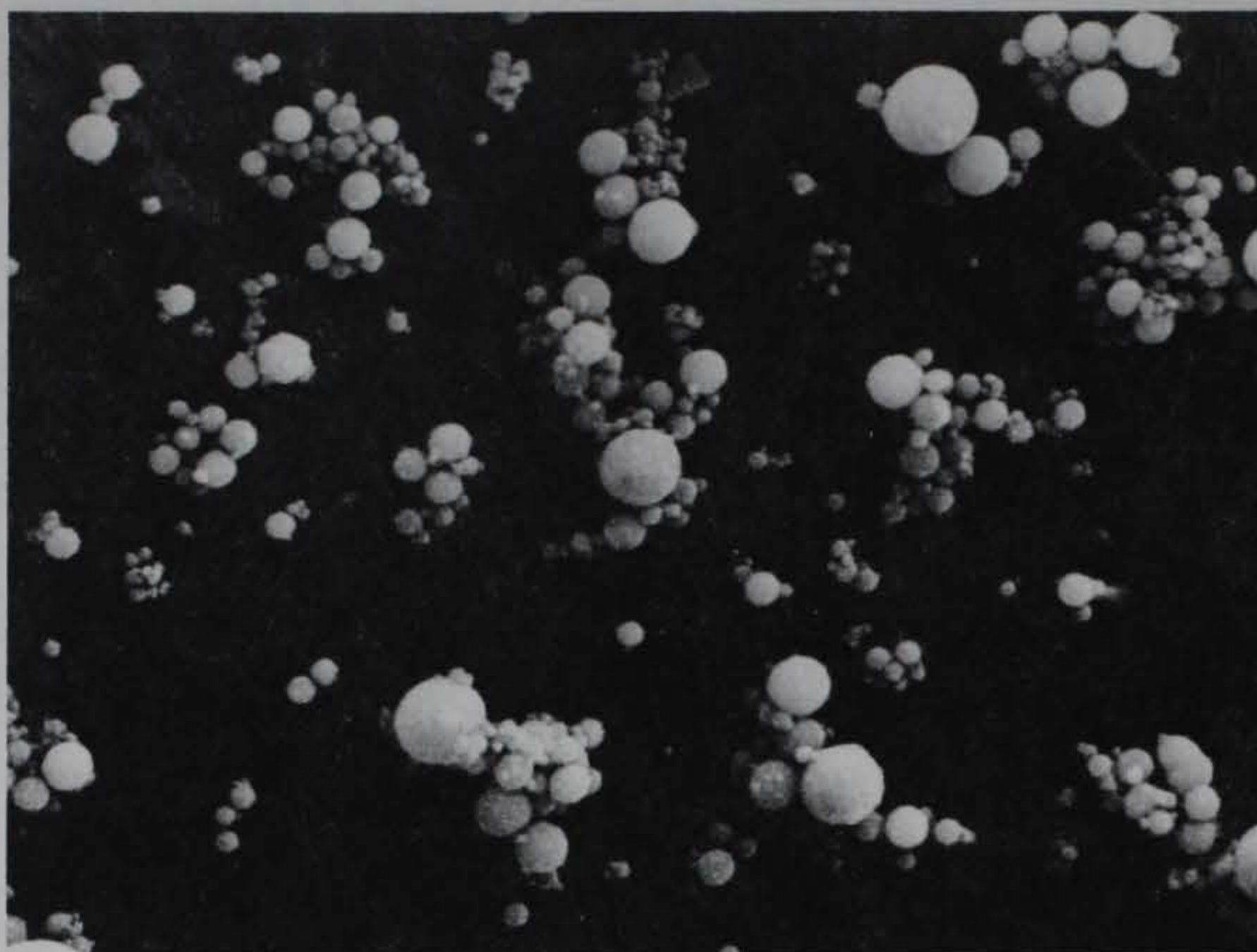
a. Fly ash AD-513, showing spherical shapes, X 2000, No. 042677-3. Largest sphere is about 5 \mu\text{m} in diameter.
