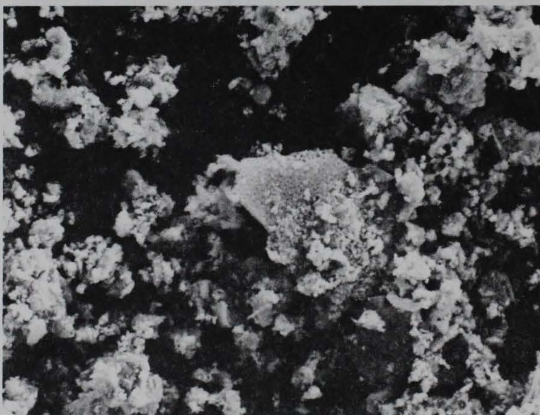
b. Natural pozzolan AD-518, X 1000. No. 102076-15. Nonspherical shapes. Largest particle is about 35 \mu\text{m} .
