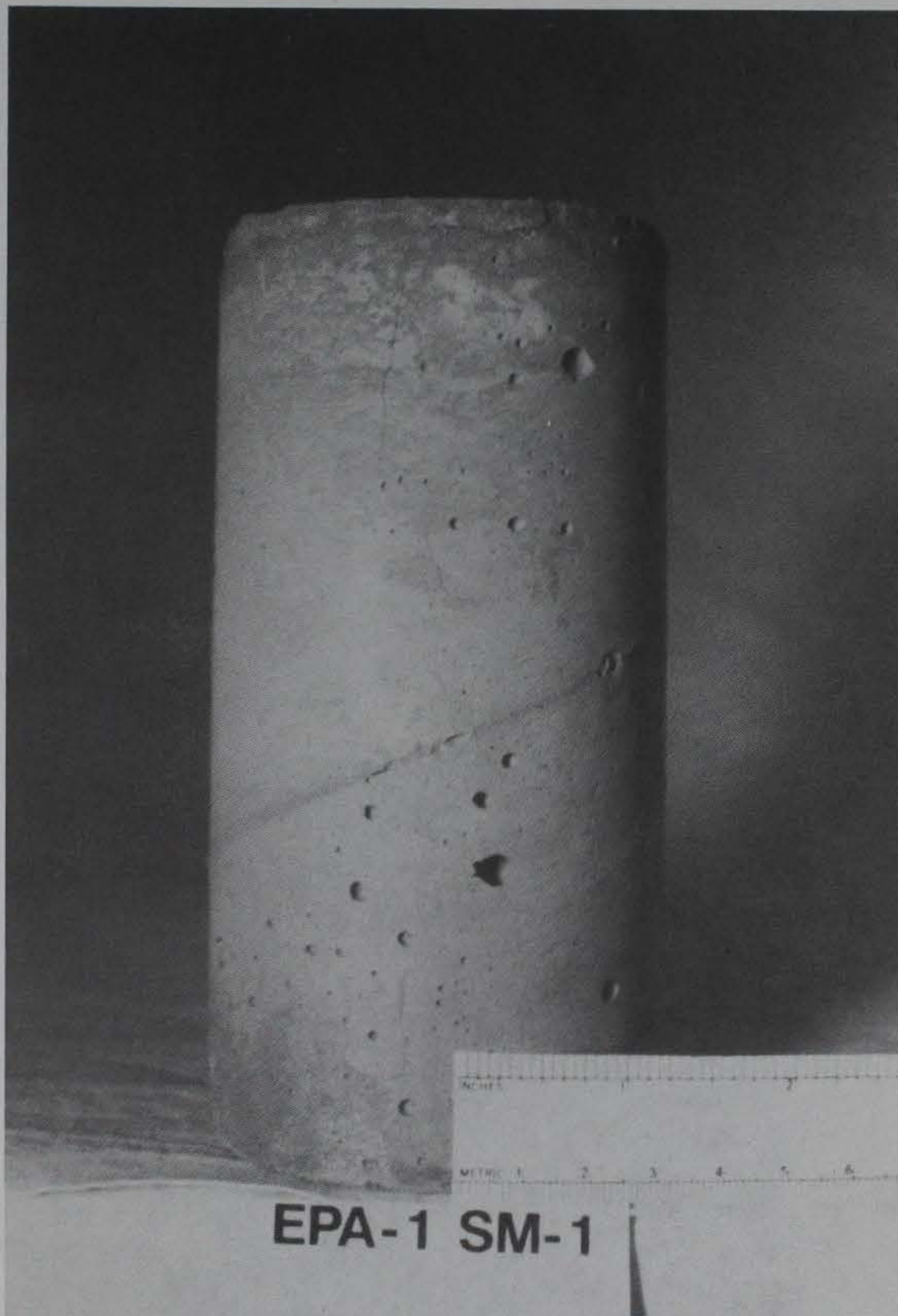
Figure 1. Cylinder of solidified filter cake. Diagonal line on circumference shows location of seam in cardboard sample mold; surface voids represent air trapped during casting
