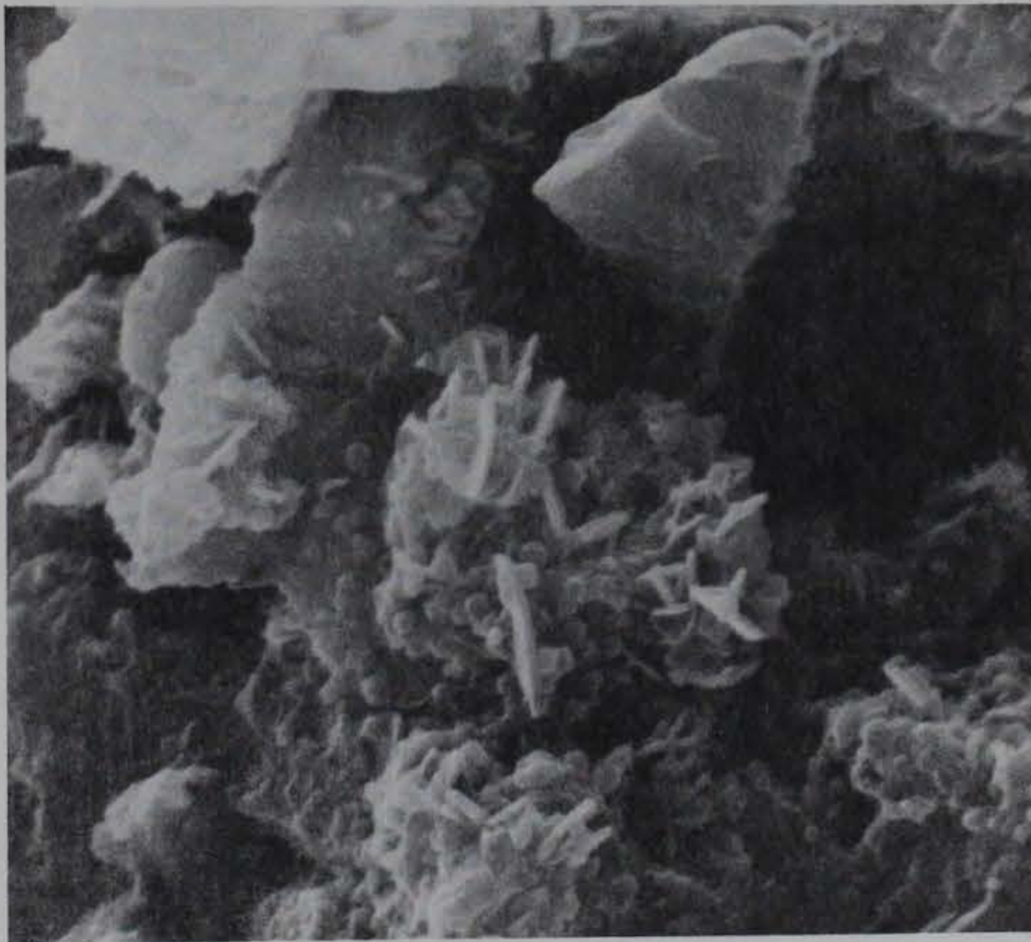
Figure 19. Type I cement, hydrated at 0.5 W/C. Specimen aged 3 days. Shown is a small cluster of hydration products from the center of Figure 18 being engulfed by calcium hydroxide. The small hexagonal platelets may be a hexagonal tetracalcium aluminate hydrate such as tetracalcium aluminate monosulfate hydrate which has formed at the expense of ettringite. The platelets range from 0.20 to 0.25 \mu\text{m} in diameter (10,000X)
