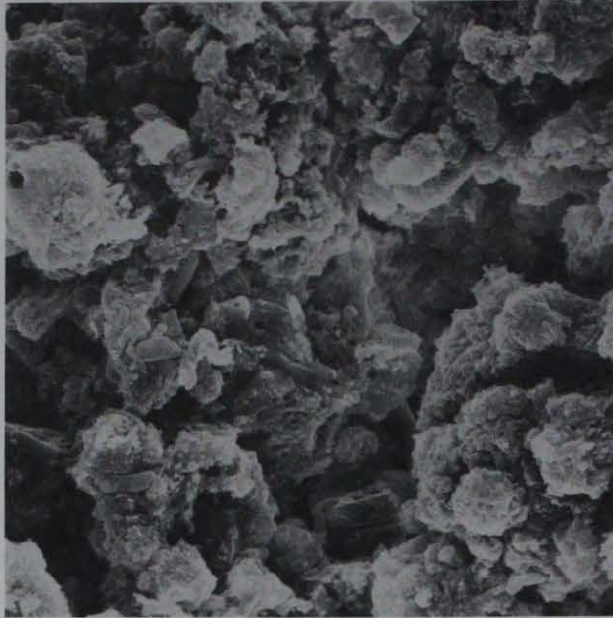
Figure 10. Ettringite-forming material, hydrated at 0.5 W/C. Specimen aged 3 days. This area shows the increased development of gypsum (?) and the presence of a few larger prisms of ettringite which developed normal to the grain surfaces (2000X)
