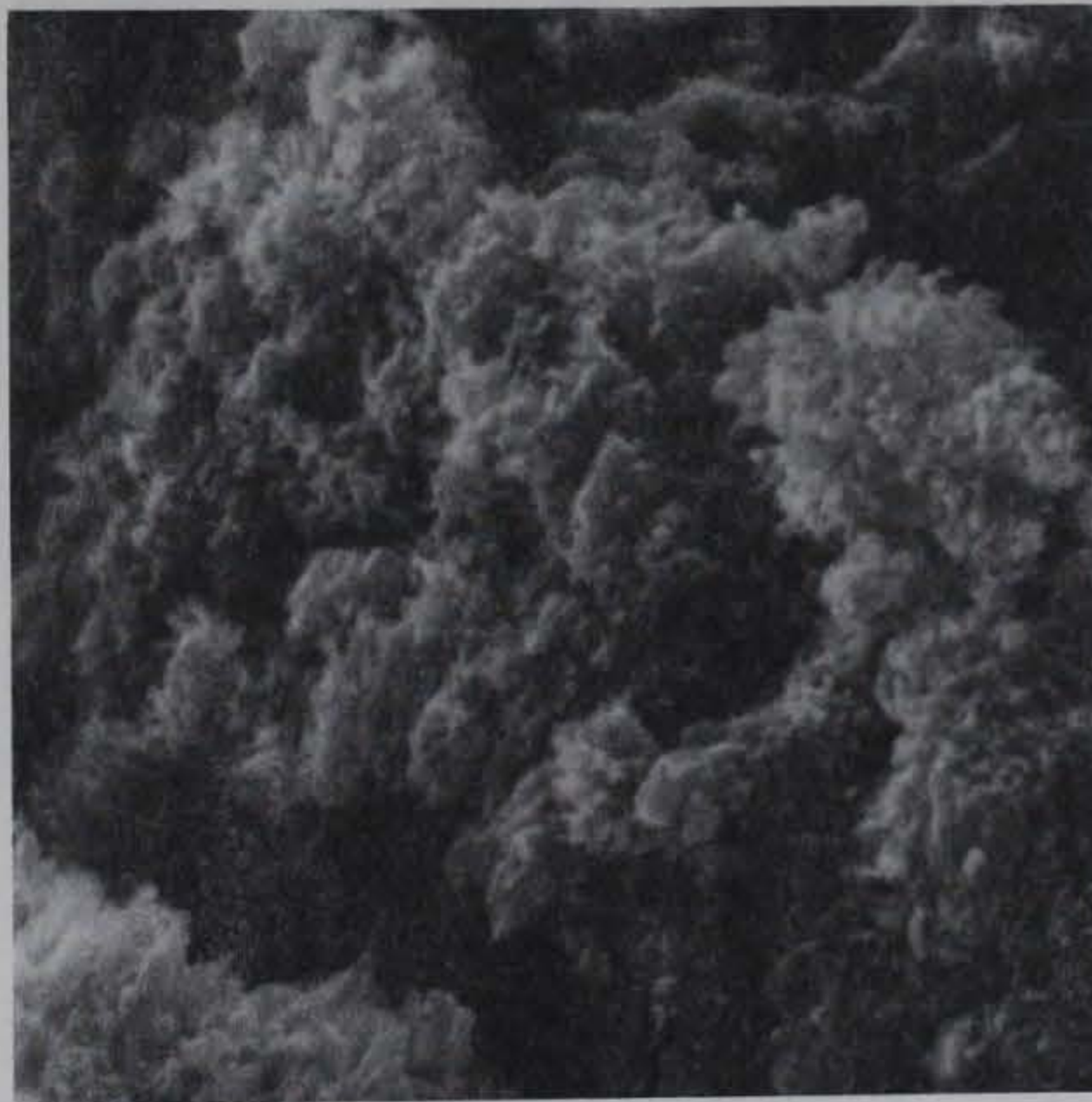
Figure 33. Type K cement, hydrated at 0.5 W/C. Specimen aged 3 days. Center of Figure 32 showing limited development of hydration products (10,000X)
