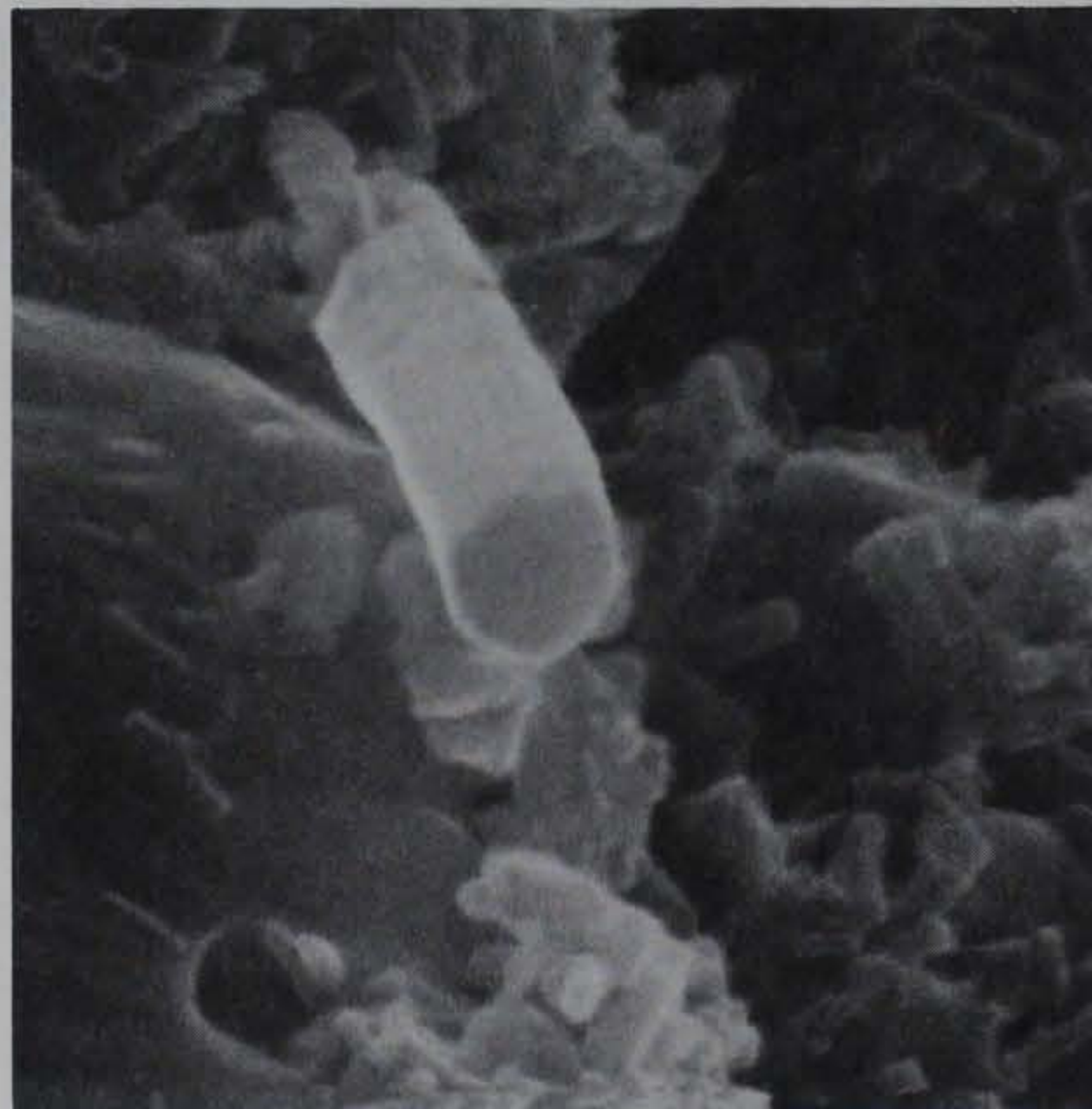
Figure 11. Ettringite-forming material, hydrated at 0.5 W/C. Specimen aged 3 days. This is the center part of Figure 10. In the center of this figure is a rod of ettringite with a hexagonal cross section. This rod, 1 \mu\text{m} in length, developed normal to the grain surface, while the majority of the smaller rods developed parallel to the grain surface and were typically 0.4 \mu\text{m} in length (20,000X)
