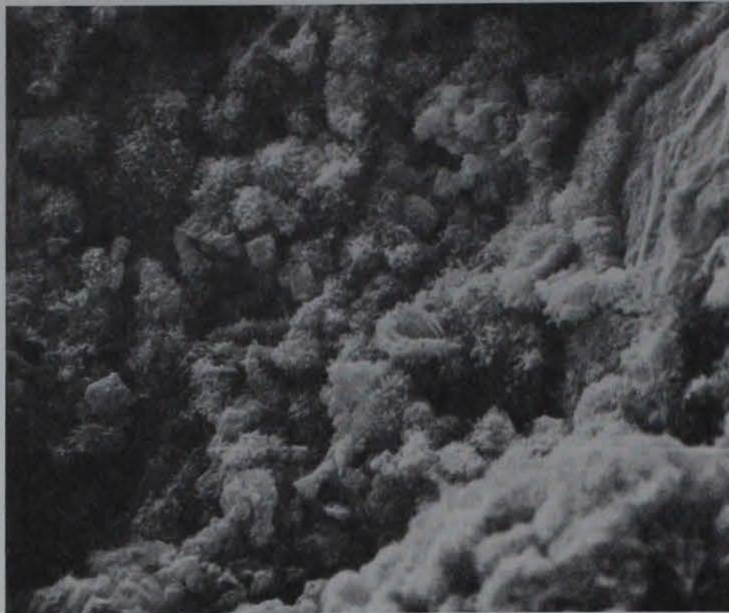
Figure 23. Type V cement, hydrated at 0.5 W/C. Specimen aged 1 day. Area shows development of calcium silicate hydrate and some ettringite crystals on the surface of the grain forming a porous interlocked coating (2000X)
