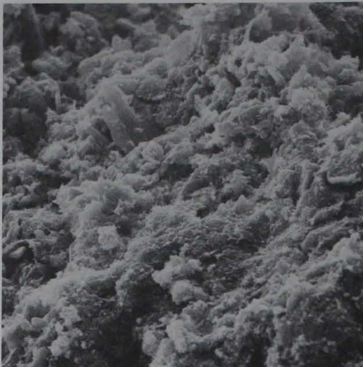
Figure 13. Ettringite-forming material, hydrated at 0.5 W/C. Specimen aged 7 days. The specimen has developed a more massive texture by this age (2000X)
