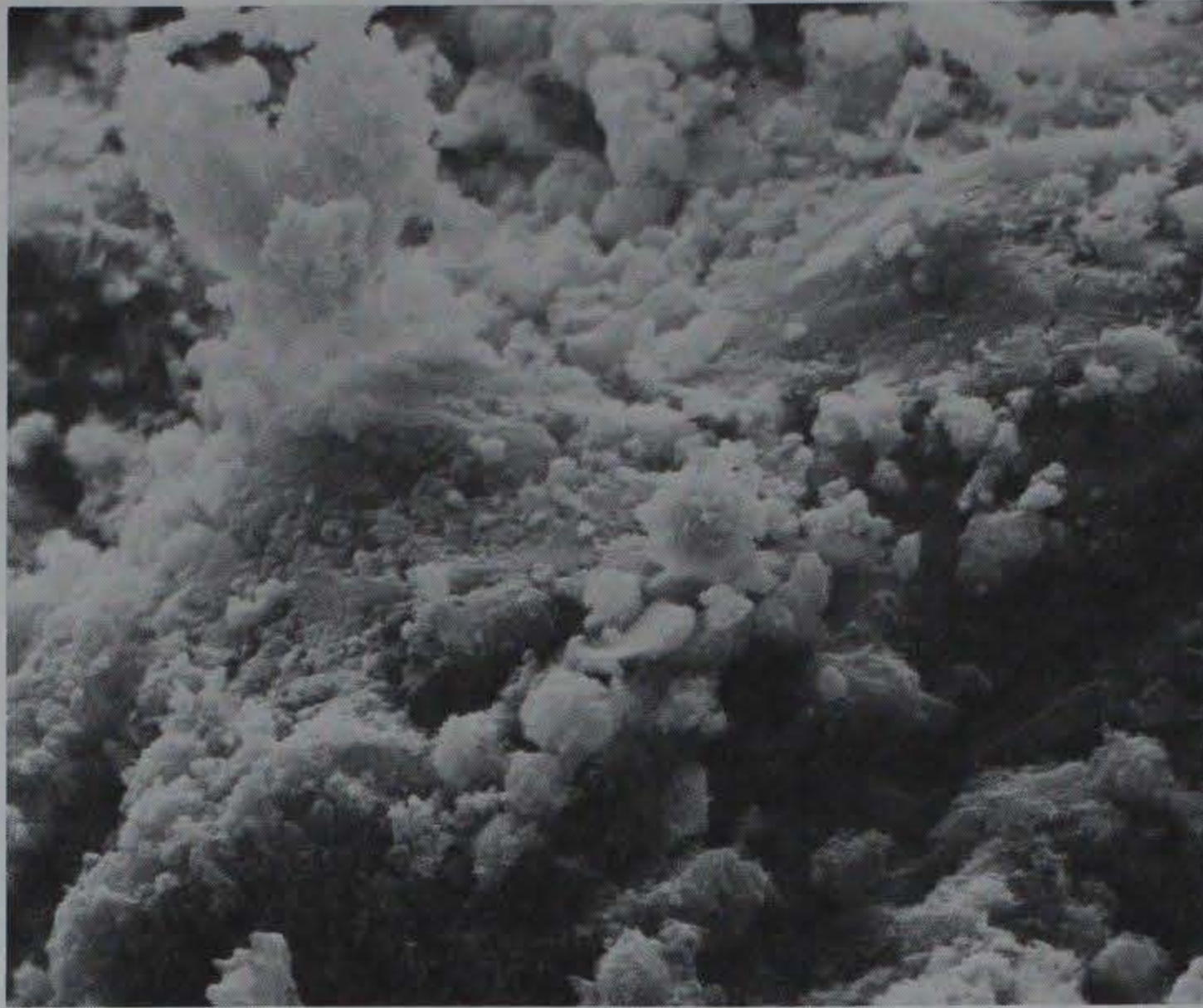
Figure 26. Type V cement, hydrated at 0.5 W/C. Specimen aged 3 days. The bulk of this specimen had a massive amorphous texture as shown here (2000X)
