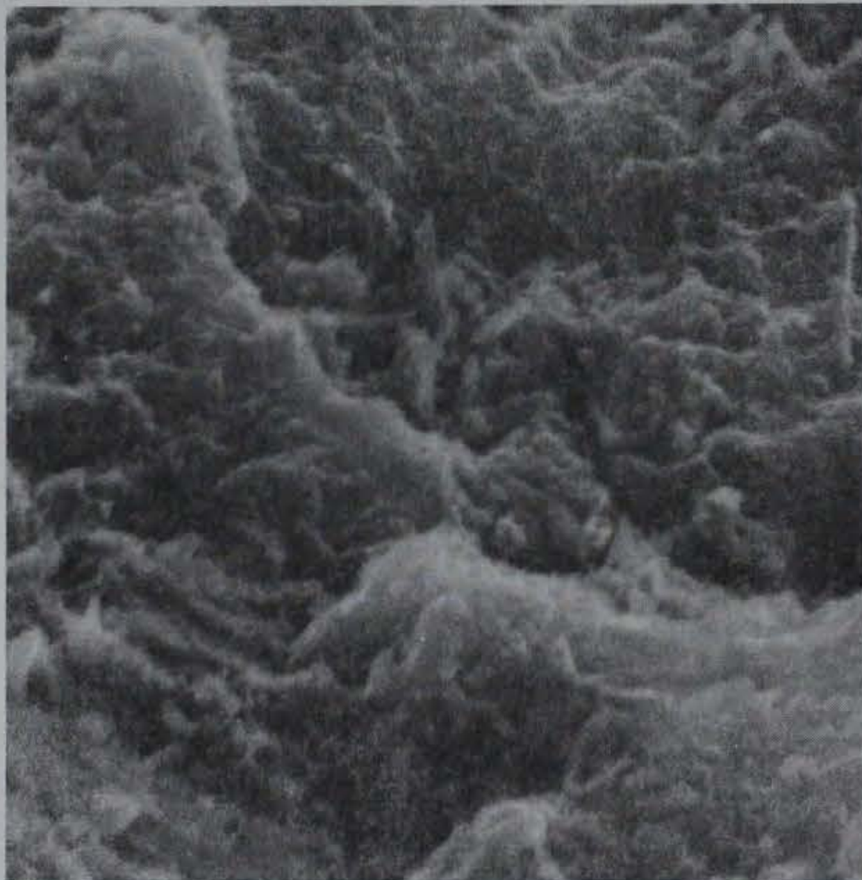
Figure 31. Type V cement, hydrated at 0.5 W/C. Specimen aged 28 days. Center of Figure 30 showing rods of ettringite (?) engulfed by calcium hydroxide (10,000X)
