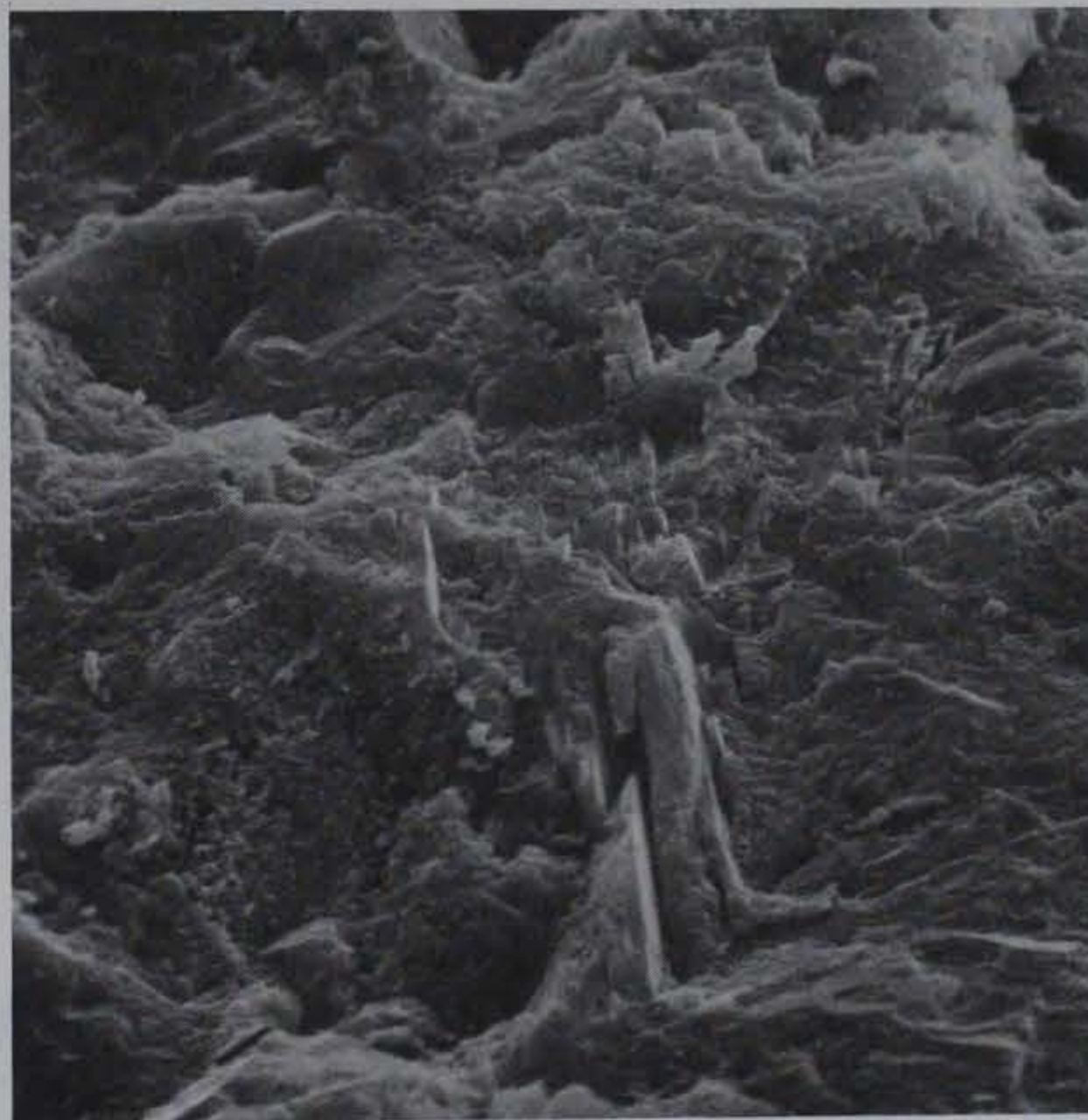
Figure 22. Type I cement, hydrated at 0.5 W/C. Specimen aged 28 days. Enlarged view of center of Figure 21. In the left center is an area of calcium silicate hydrate that has been engulfed by calcium hydroxide (2200X)
