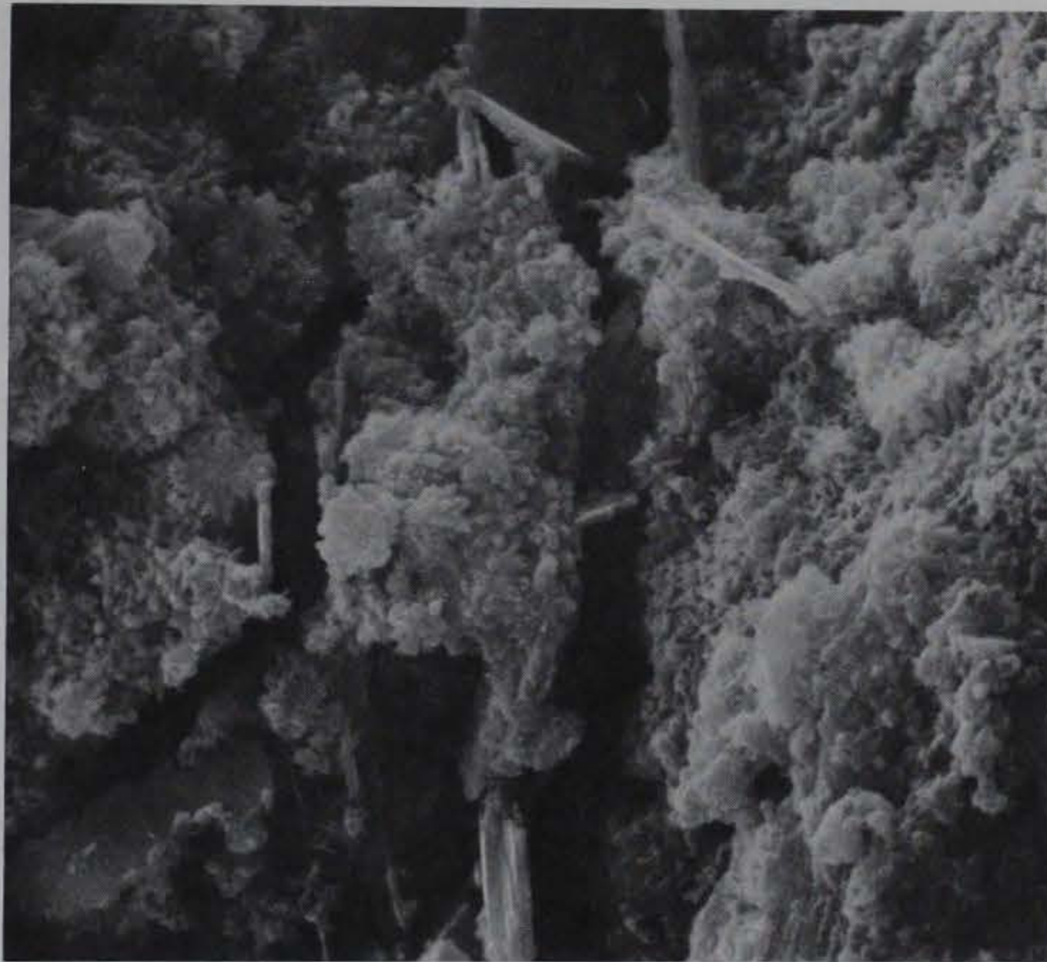
Figure 16. Type I cement, hydrated at 0.5 W/C. Specimen aged 1 day. The area shown is in the center of Figure 15. Much of the surface is coated by small crystals of calcium silicate hydrate. The platy crystals in the cracks indicate that the cracks formed during hydration rather than during specimen preparation. They may be calcium hydroxide or monosulfoaluminate or both (5000X)
