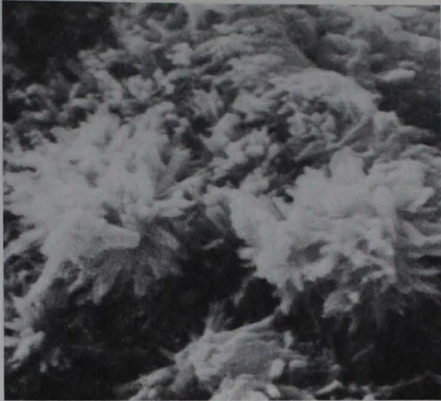
Figure 25. Type V cement, hydrated at 0.5 W/C. Specimen aged 1 day. Center of Figure 24 shows interlocked clusters of fibrous Type I 14 calcium silicate hydrate. The cluster on the right is 2 \mu\text{m} in diameter (20,000X)
