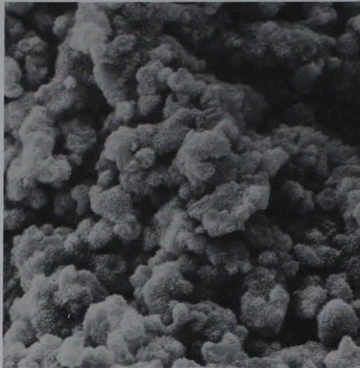
Figure 6. Alite, hydrated at 0.5 W/C. Specimen aged 7 days. This specimen shows a slight reduction in pore space as the clusters of calcium silicate hydrate have grown closer together. Also, calcium hydroxide grains are becoming more apparent at this age (2000X)
