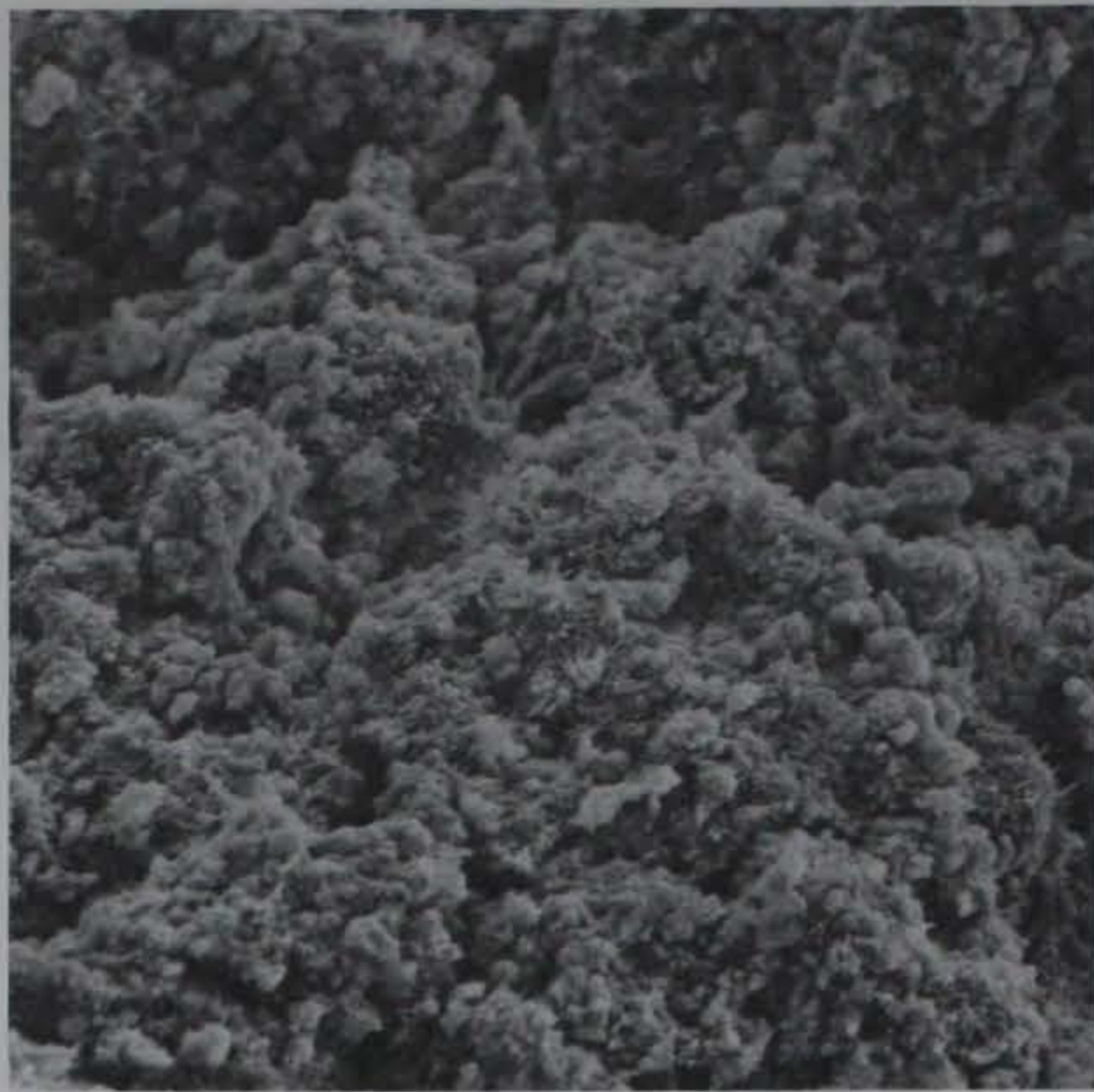
Figure 34. Type K cement, hydrated at 0.5 W/C. Specimen aged 28 days. Specimen showed little change in available pore space but did show considerable development of ettringite (500X)
