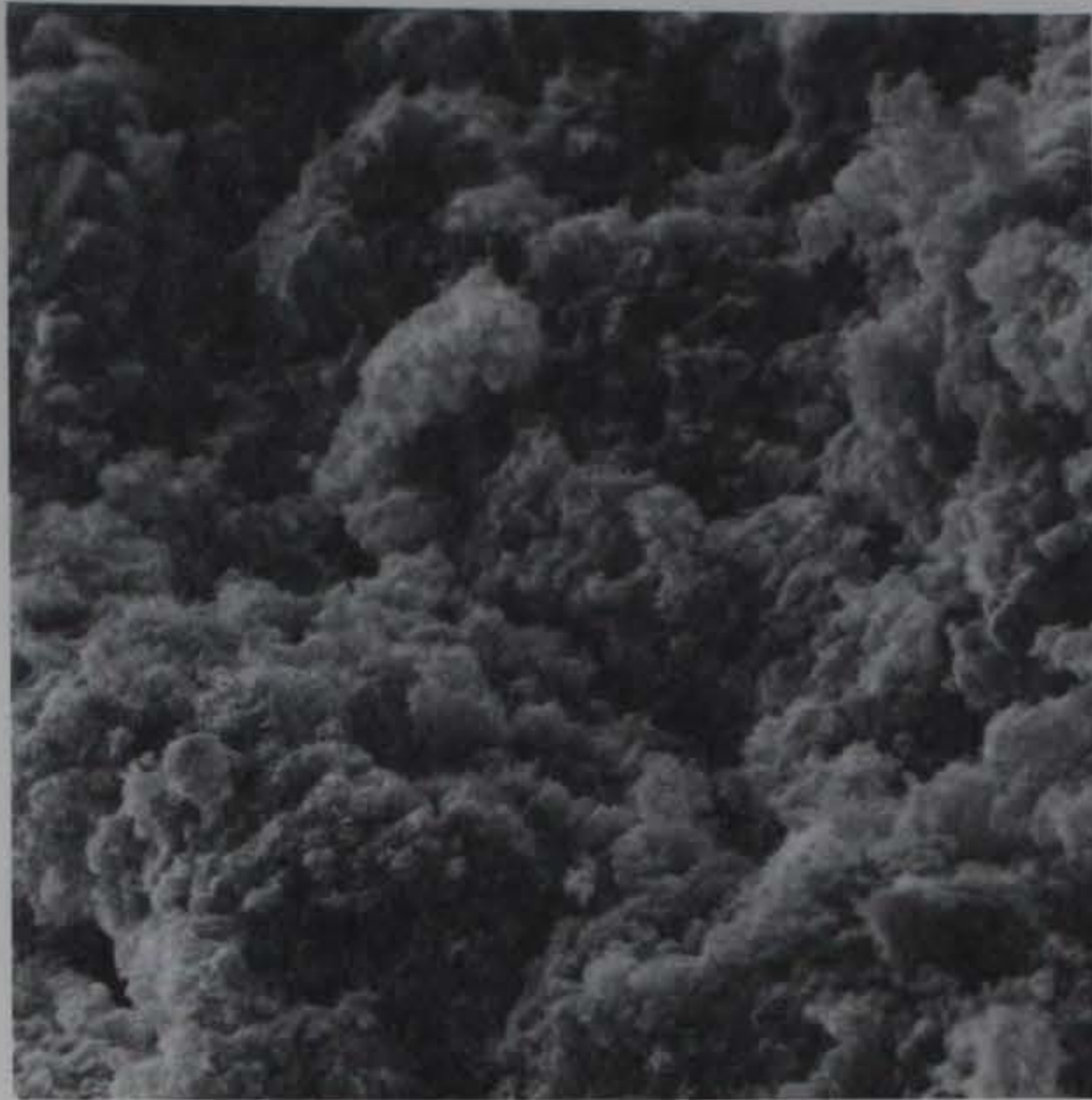
Figure 32. Type K cement, hydrated at 0.5 W/C. Specimen aged 3 days. Specimen showed very little development of hydration product at this age (2000X)
