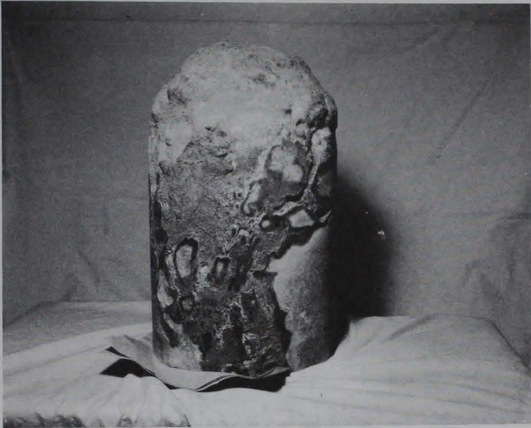
Figure 5. Sample A12 from satellite Hole 4. The sand was mixed into most of it. Note the voids in the sample due to the turbulence during placement. The sample is 1.1 ft long
