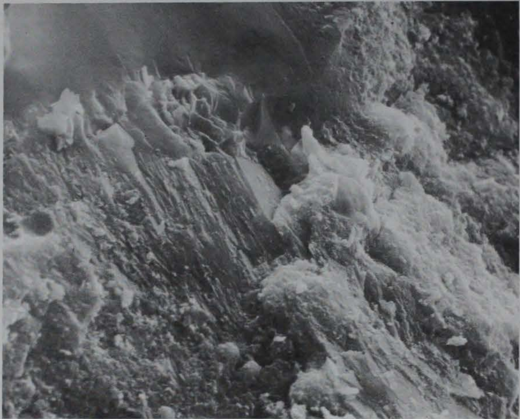
Figure 8. Micrograph 030581-26, X1900. Broken surface of Plug 2 cube CL-30 GRT-158. An unhydrated cement grain is seen in the upper left corner, bordered by calcium hydroxide and calcium silicate hydrate. The specimen was about 1 year old
