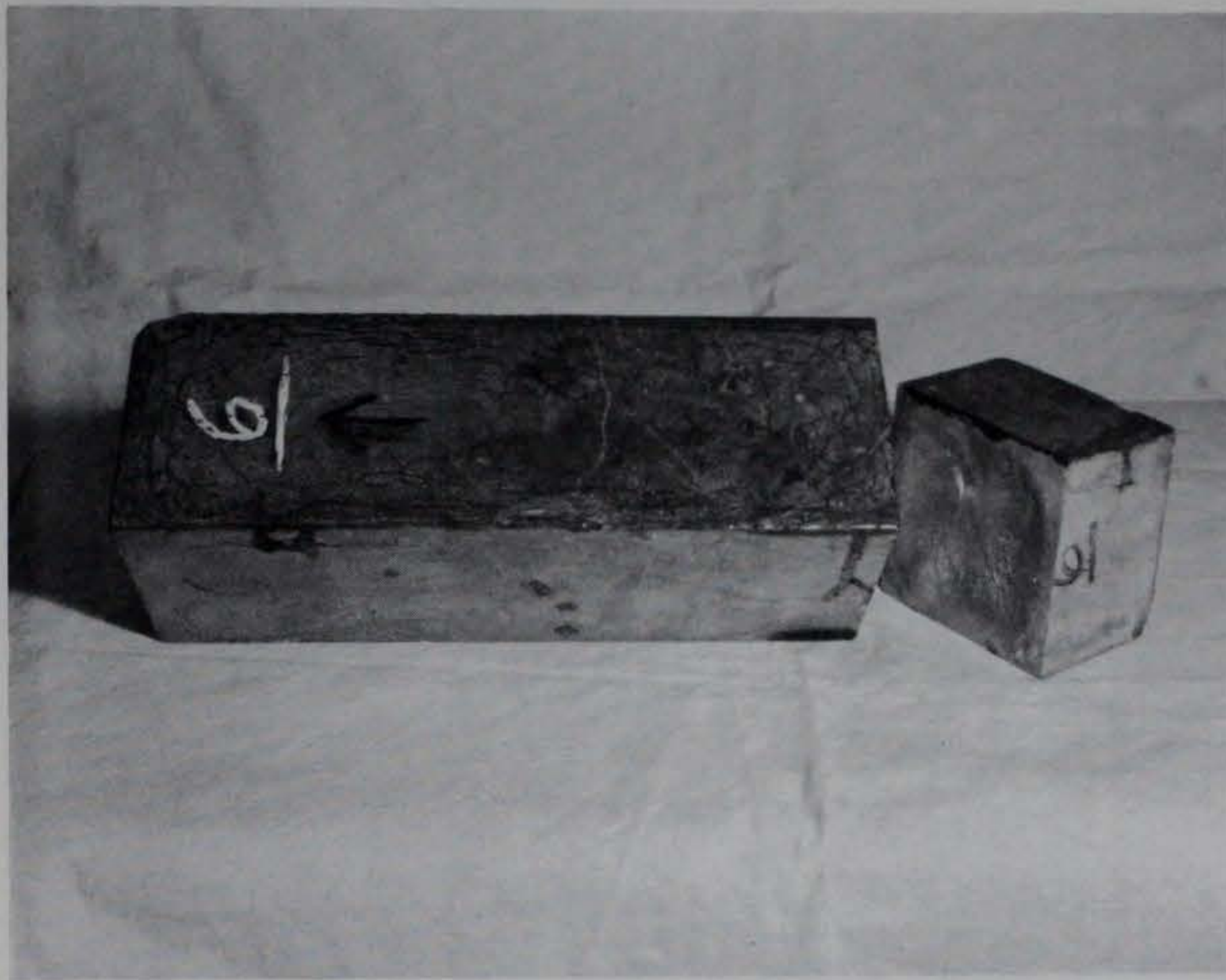
Figure 1. Plug 2 unrestrained prism CL-30 GRT-6 that broke at approximately 1-year age. Note the cracking on the surface and the faint white crack in the center of the top surface, X0.25
