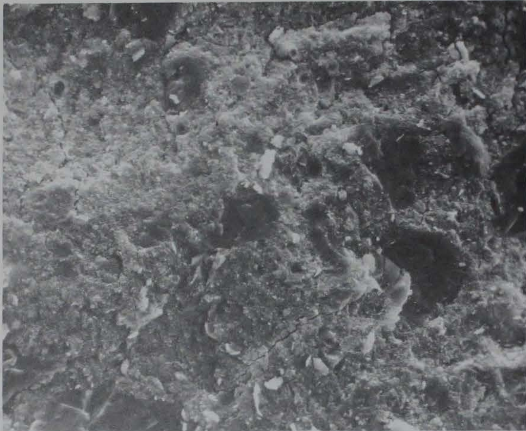
Figure 12. Micrograph 041383-4, X530. Microstructure of Plug 1 grout at 3 years. This sample came from a piece of a cylinder. Three grains of unhydrated cement can be seen in the right central portion of the micrograph. Note the microstructure appears denser than the same grout at 370-days age (Figure 6)
