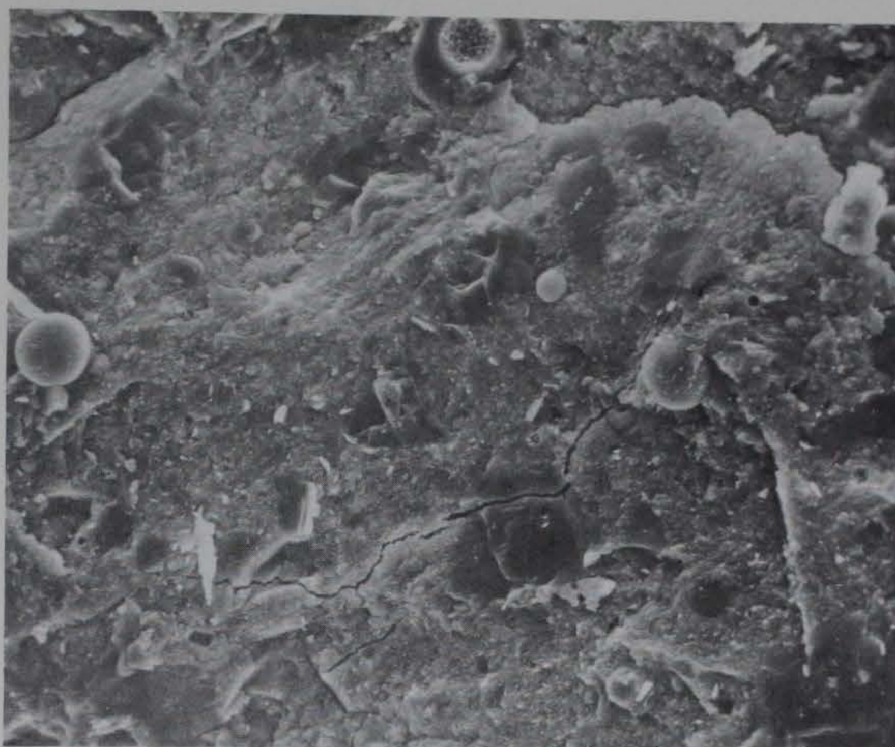
Figure 13. Micrograph 041383-15, X510. Microstructure of Plug 2 grout at 3 years. This sample came from cube CL-30 GRT-158 grout. The surface of this grout looks denser than Plug 1 grout of the same age (Figure 12). Unhydrated portland cement and fly ash spheres can be seen in the micrograph. A broken fly ash sphere is in the upper central portion of the micrograph
