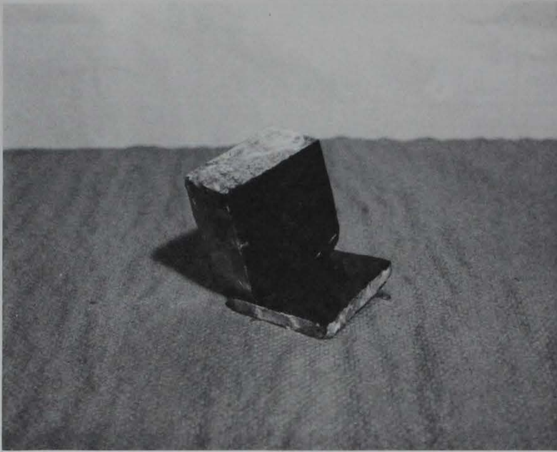
Figure 2. Plug 2 cube CL-30 GRT-158 after it had been sawed to obtain a 370-day-old sample. Notice the white material on the outer surfaces of the cube, X0.38
