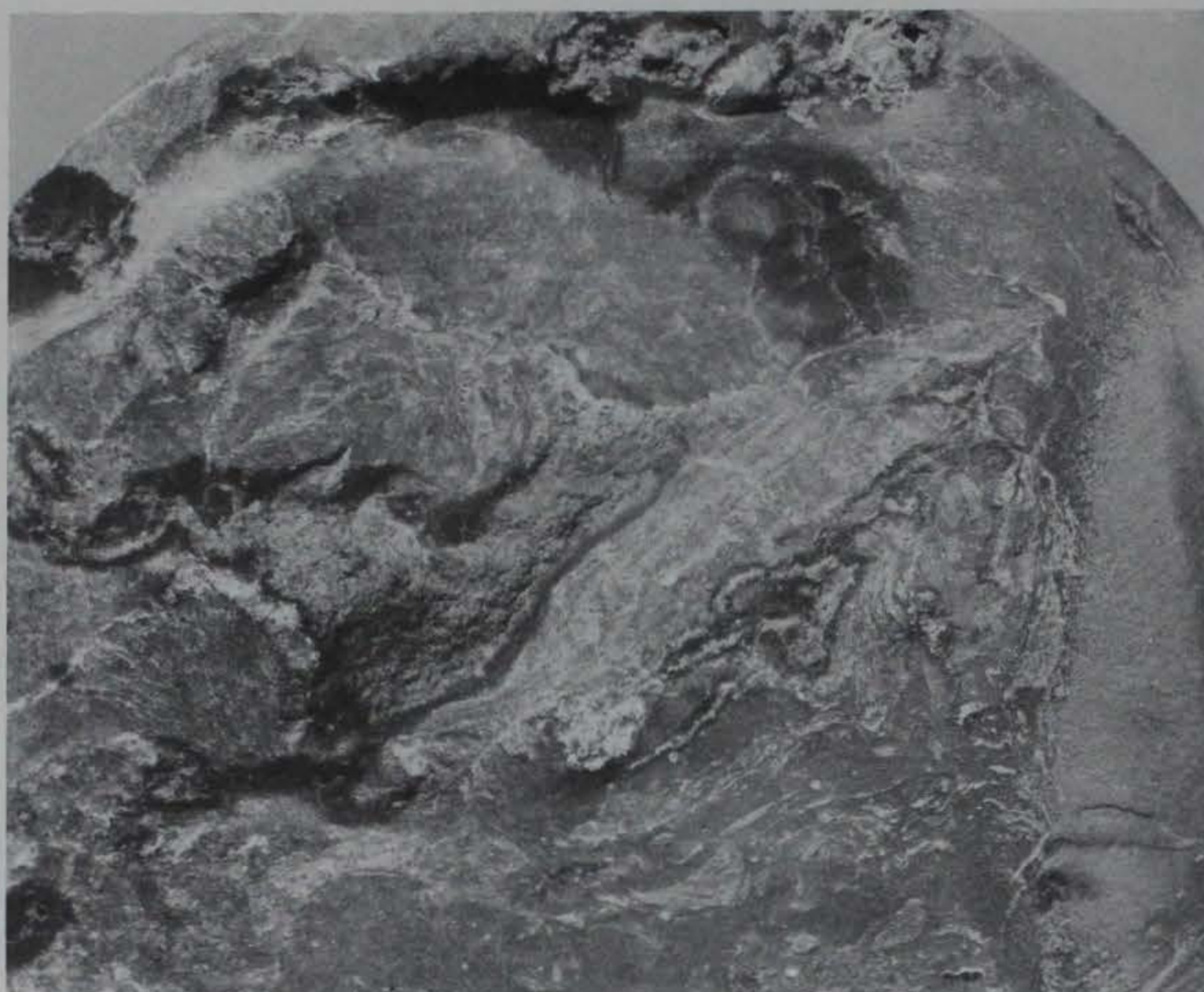
Figure 4. Sample A12 from bottom of satellite Hole 4. Note the sand particles in the center and some on the outer upper perimeter. The lower right corner shows the discoloration found in the sample; is probably carbonation. About natural size
