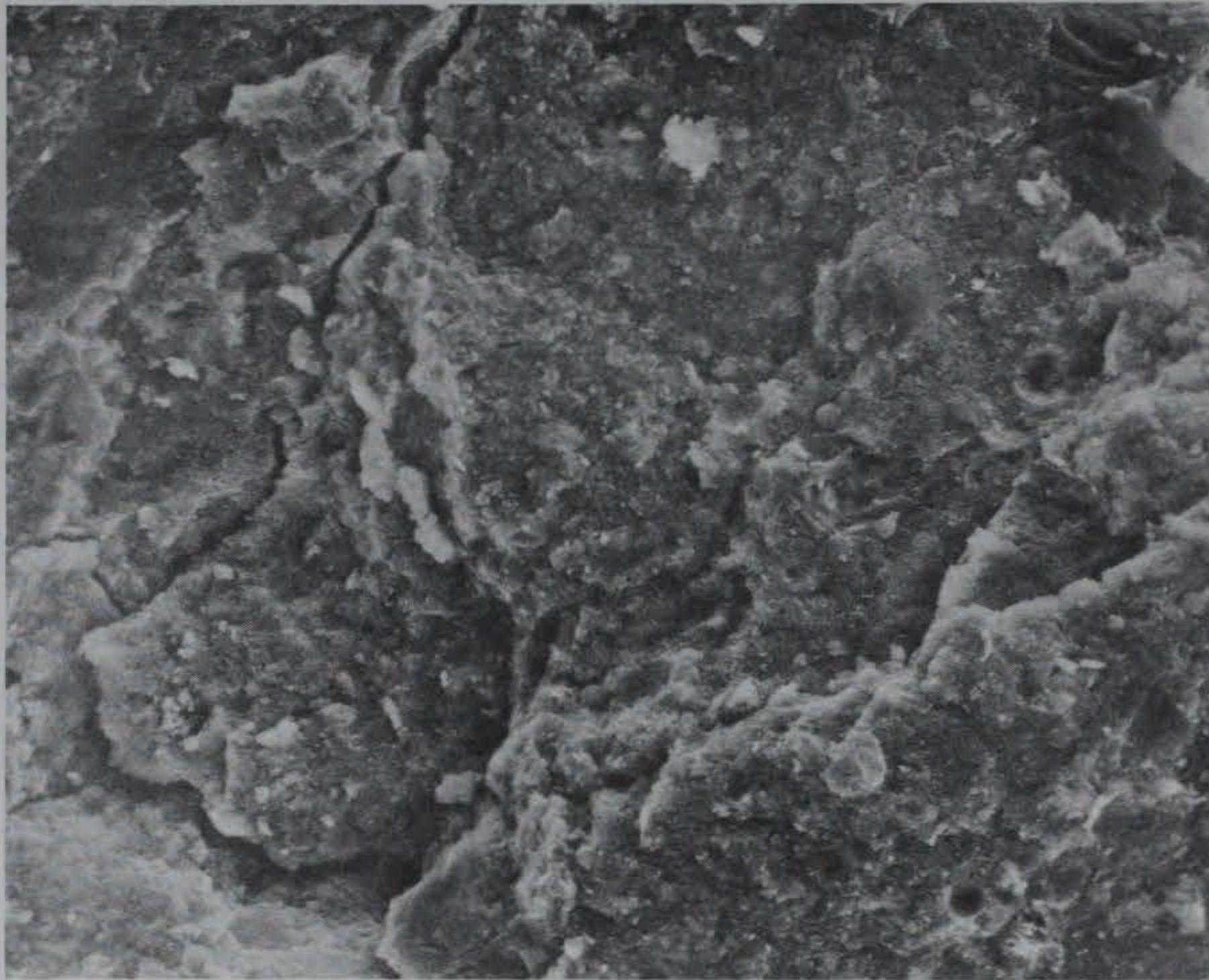
Figure 6. Micrograph 030581-11, X500. Typical morphology of Plug 1 cube A4 showing some fly ash spheres on a broken surface. The age is intended to be equivalent to 370 days
