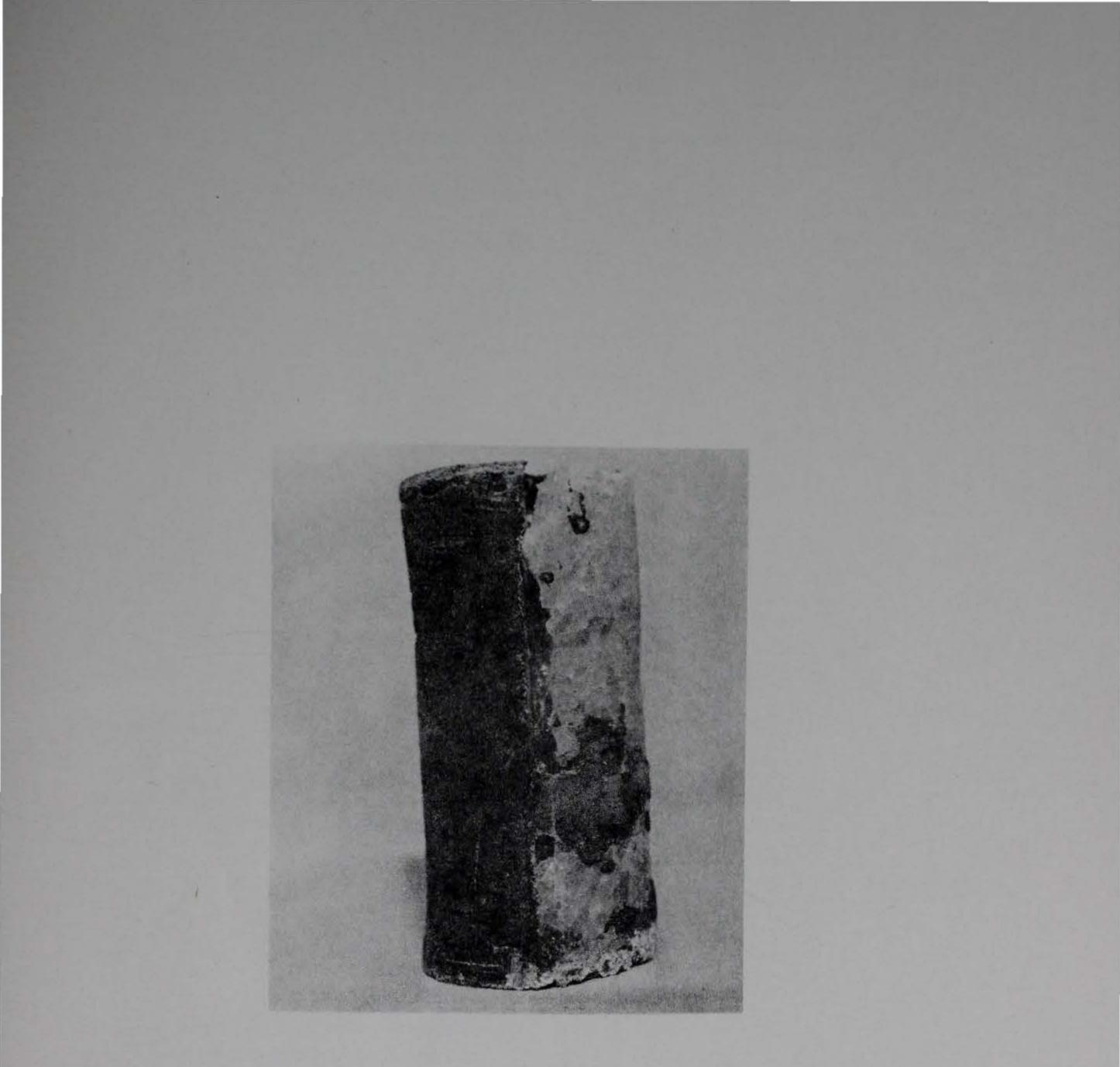
Photograph 1. View of ruined SBH sample made of TT83 grout (left) and rock salt (right) after fresh water reached it. The dissolution of salt along the contact surface is evident.
