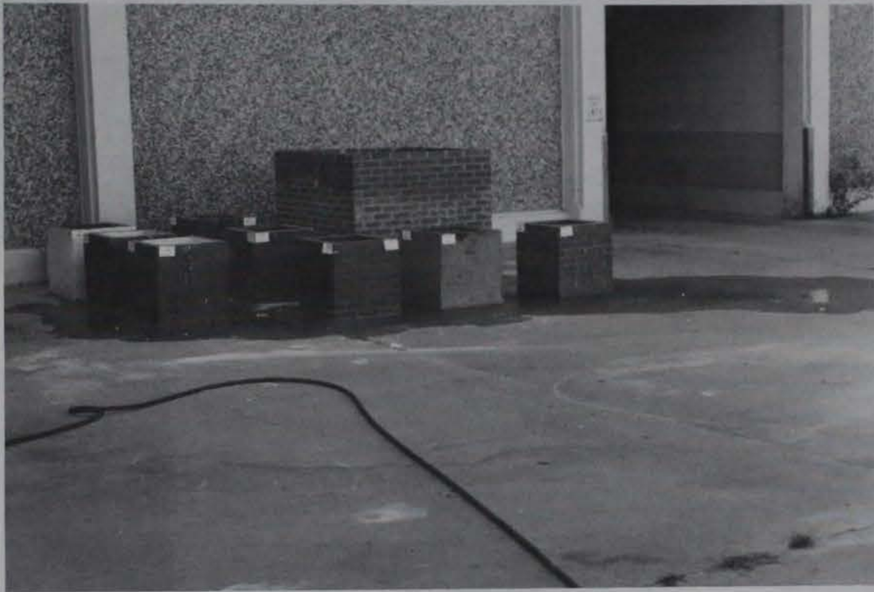
Figure 21. Brick cubes to test sealants and systems for preventing flood damage
