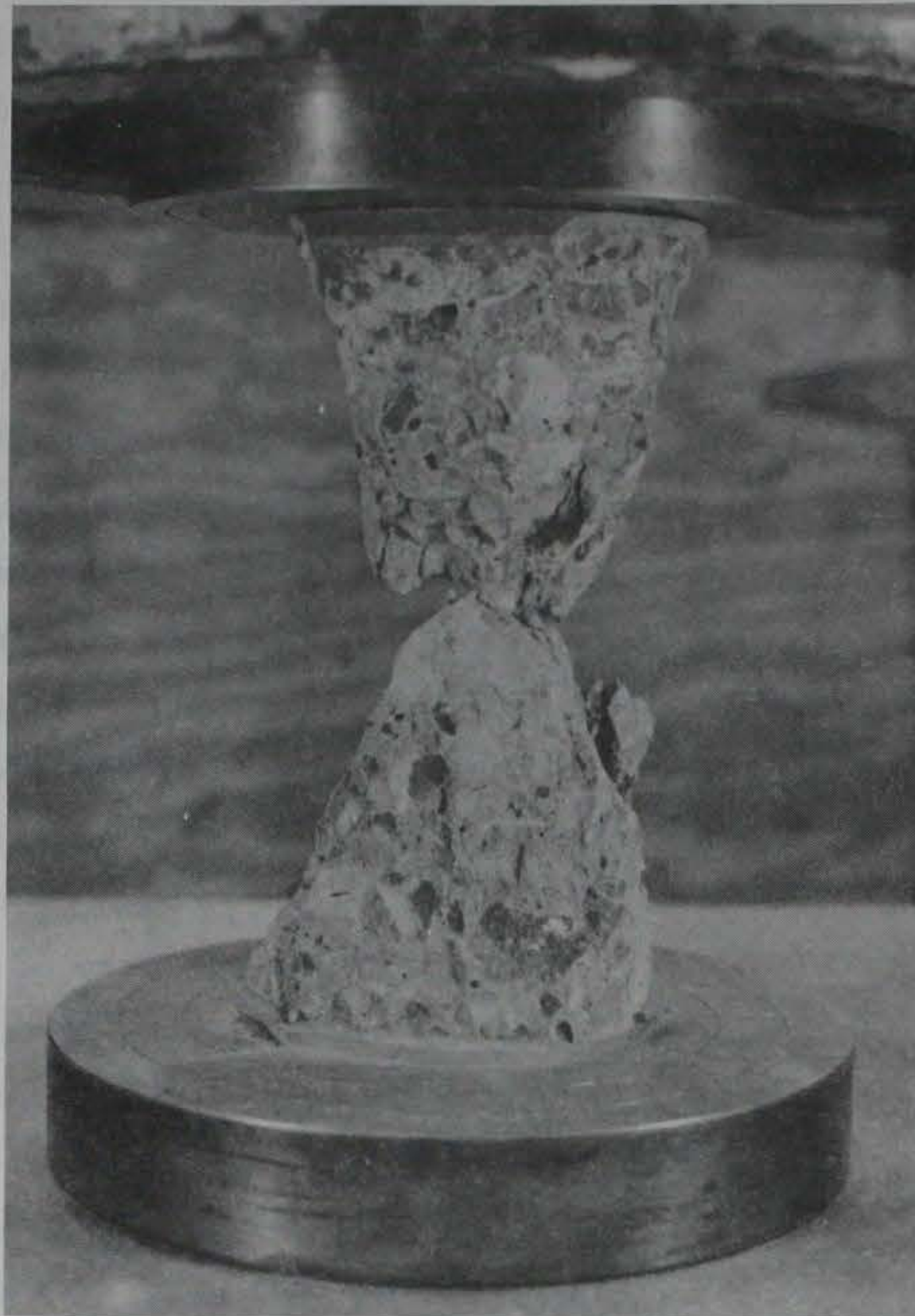
Figure A1. Typical conical fracture expected from the compressive strength test
