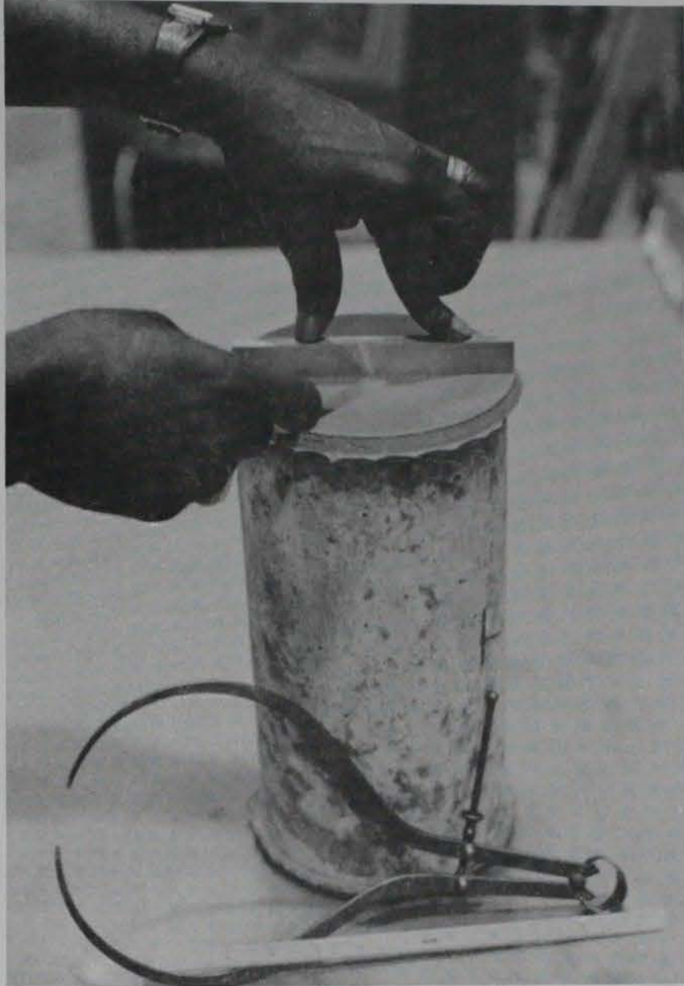
Figure A2. Checking planeness of the capped end of a concrete cylinder before testing
