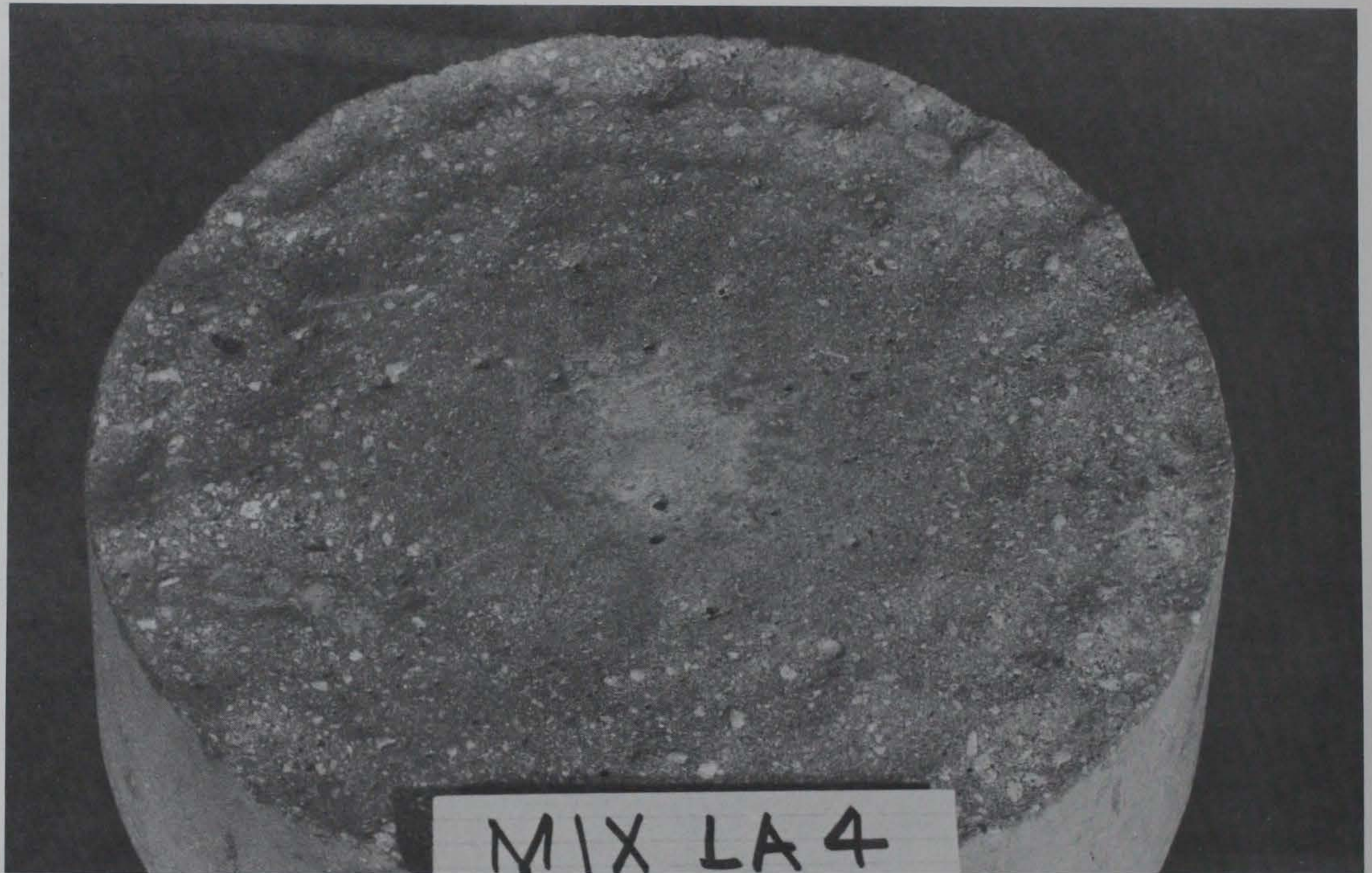
Figure 8. Abrasion-erosion specimen at conclusion of testing, Mixture LA4
