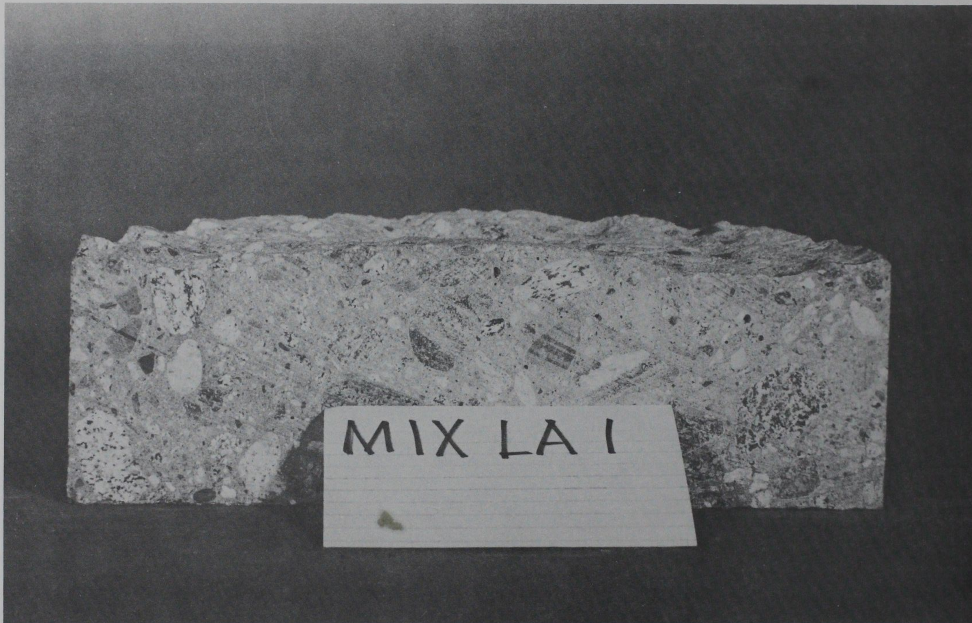
Figure 2. Sawn abrasion-erosion specimen at conclusion of testing, Mixture LA1 (full section view). This specimen is representative of Mixtures LA1, LA5, and LA6
