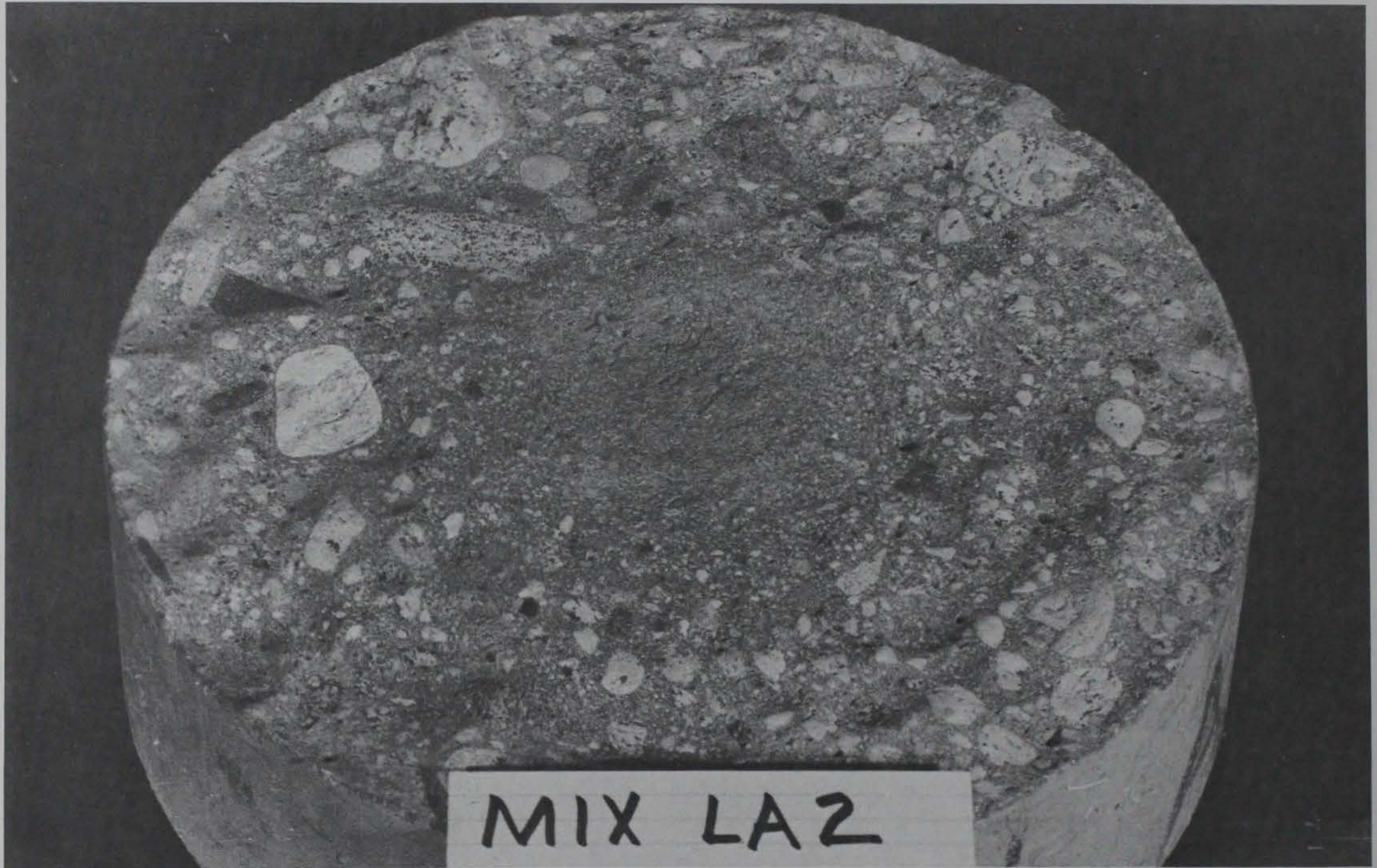
Figure 4. Abrasion-erosion specimen at conclusion of testing, Mixture LA2
