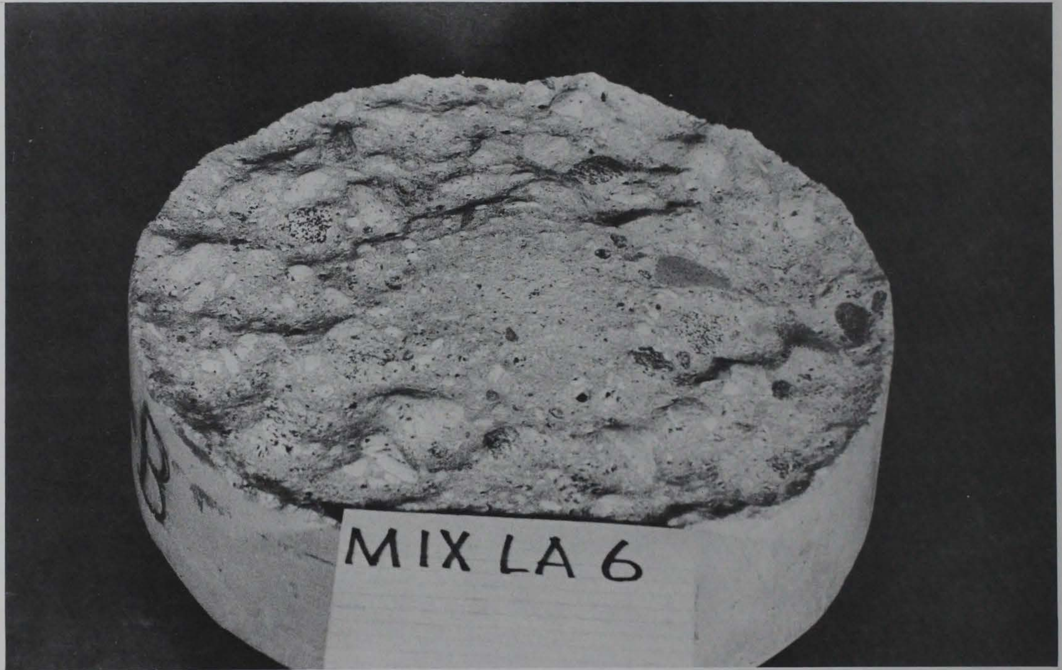
Figure 10. Abrasion-erosion specimen at conclusion of testing, Mixture LA6
