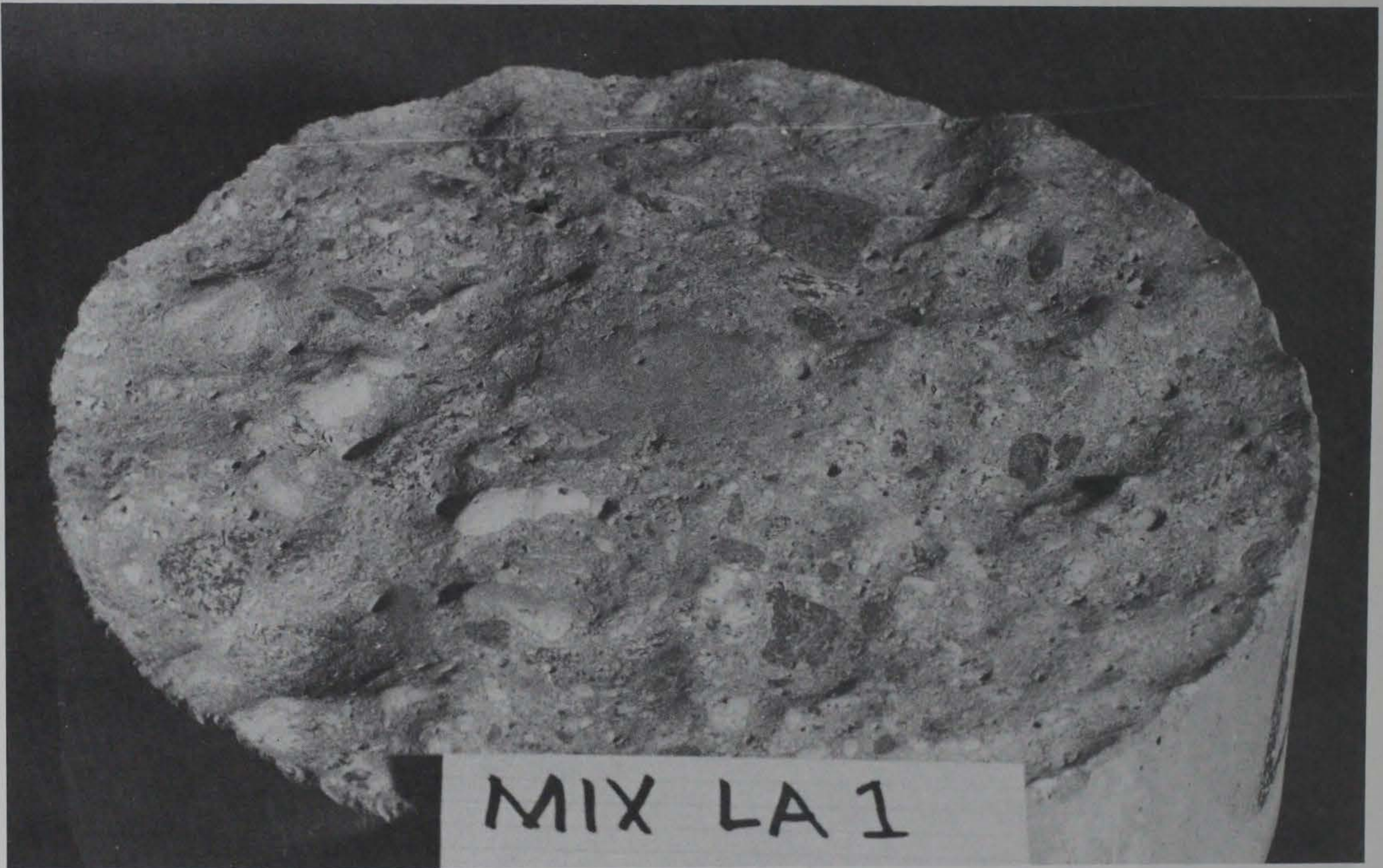
Figure 1. Abrasion-erosion specimen at conclusion of testing, Mixture LA1
