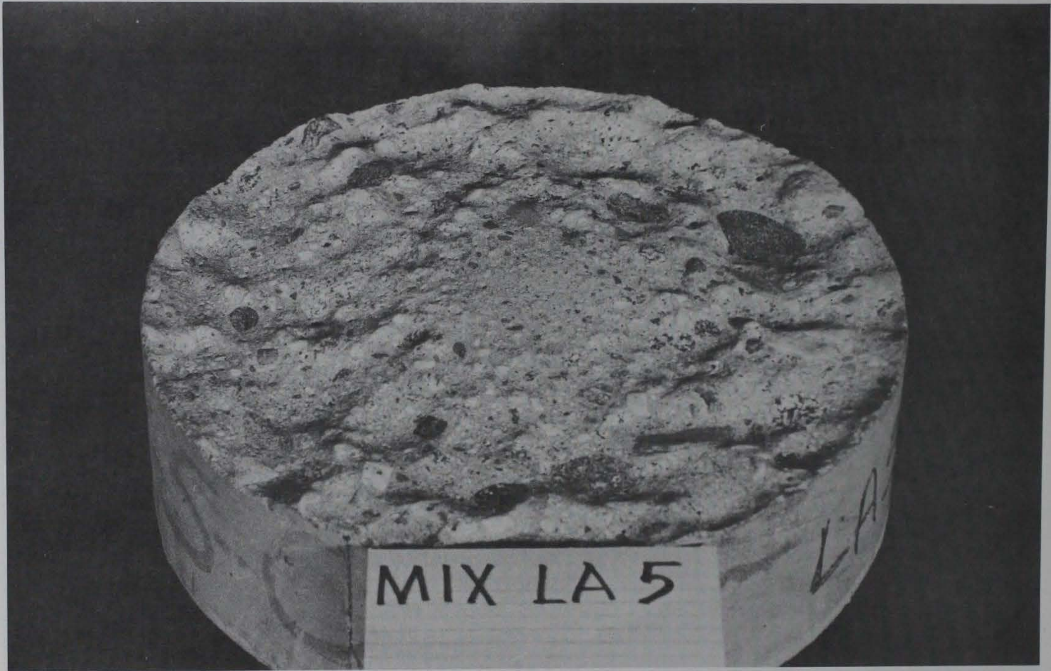
Figure 9. Abrasion-erosion specimen at conclusion of testing, Mixture LA5
