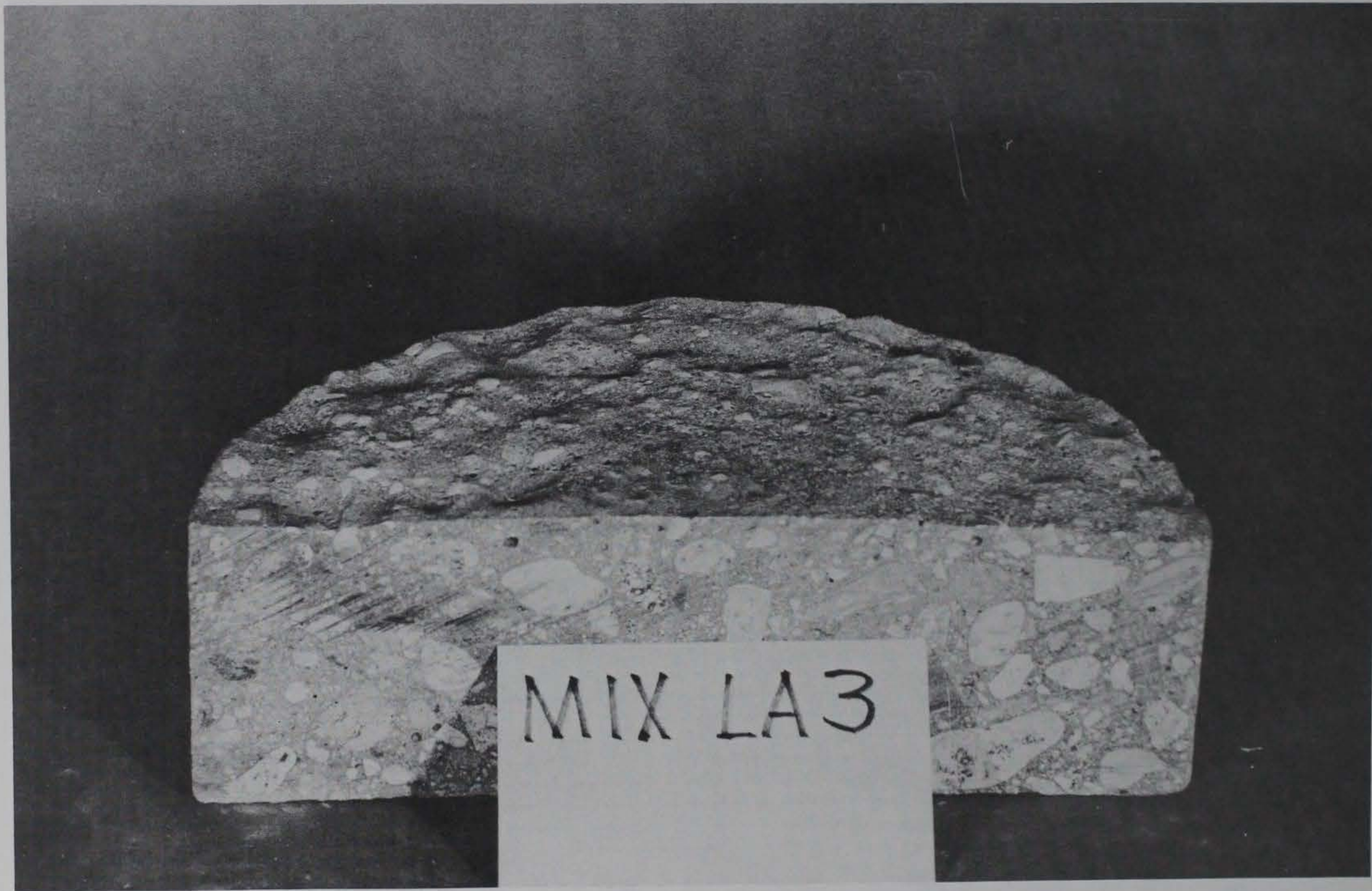
Figure 7. Sawn abrasion-erosion specimen at conclusion of testing, Mixture LA3 (oblique view). This specimen is representative of Mixtures LA2, LA3, and LA4
