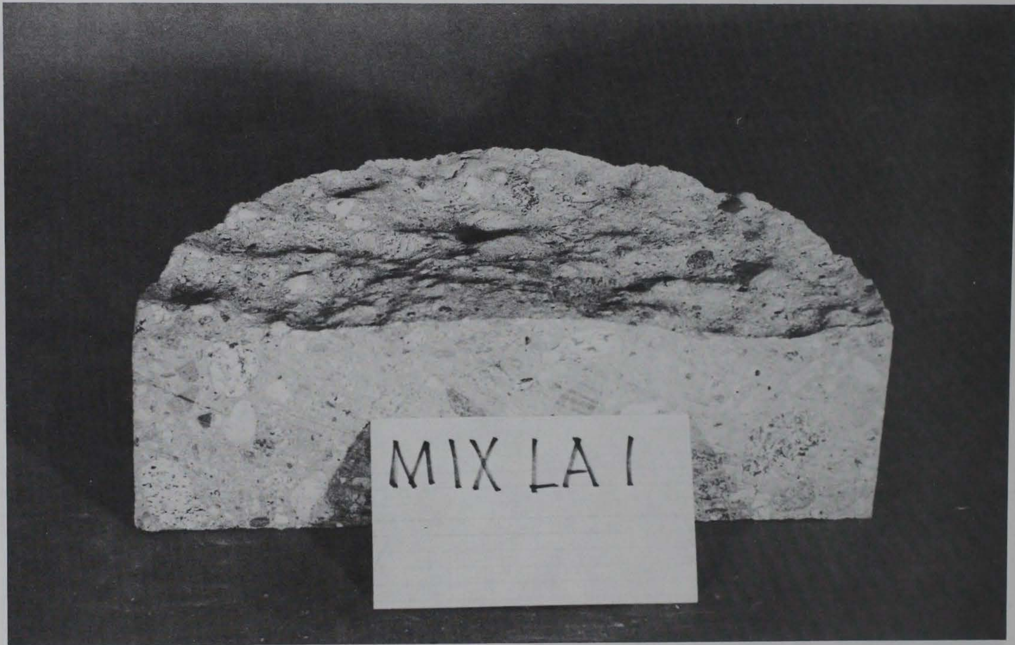
Figure 3. Sawn abrasion-erosion specimen at conclusion of testing, Mixture LA1 (oblique view). This specimen is representative of Mixtures LA1, LA5, and LA6
