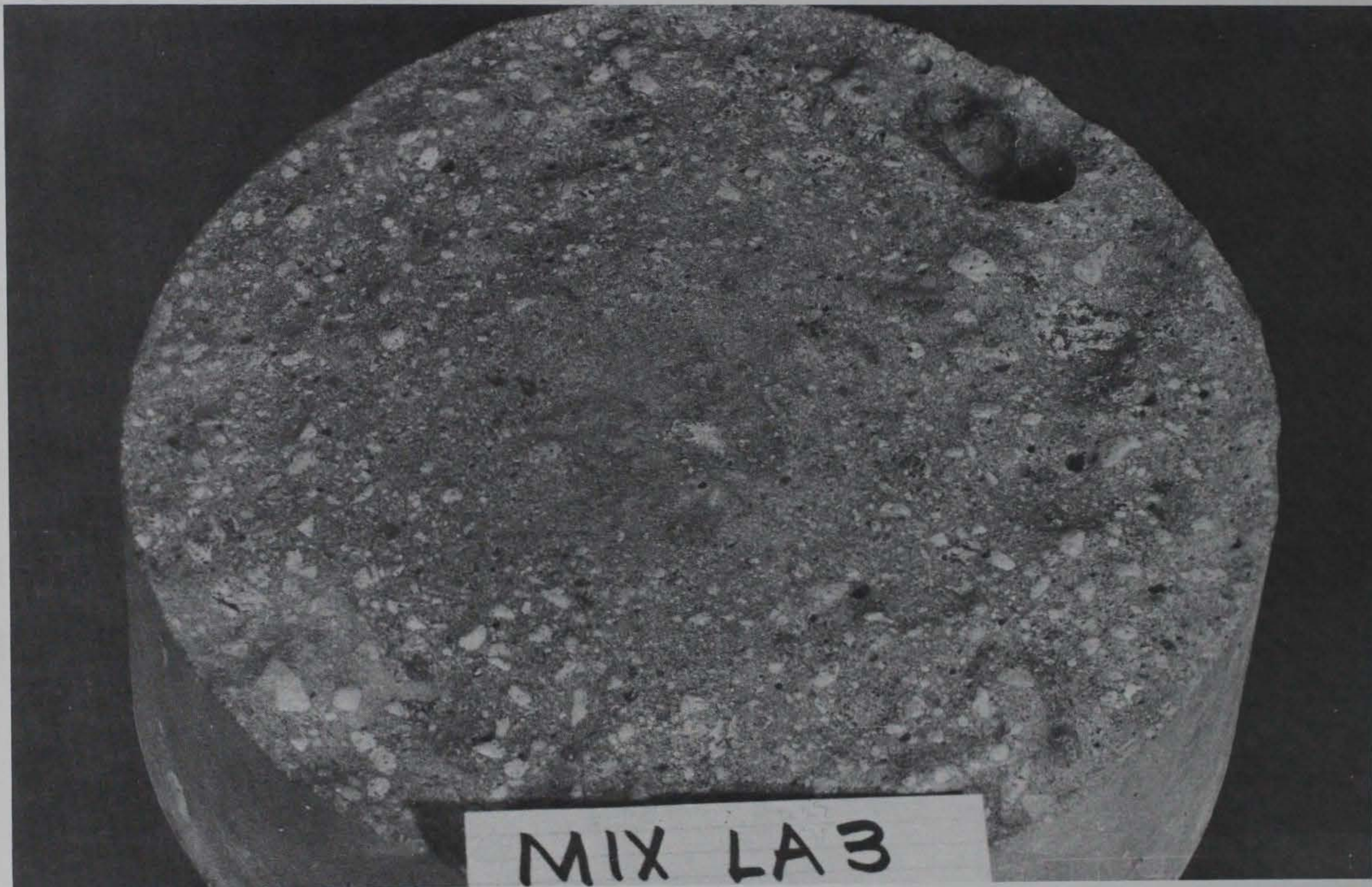
Figure 5. Abrasion-erosion specimen at conclusion of testing, Mixture LA3
