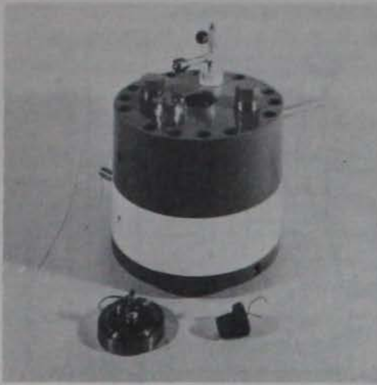
Fig. 3--100 MPa Explosive-loaded Uniaxial Strain Test Device.
