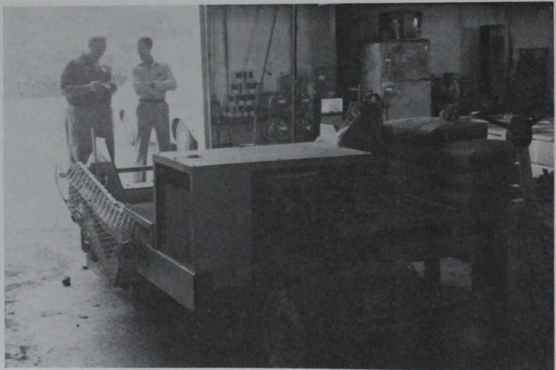
Figure 9. Paving machine used to place pervious concrete
