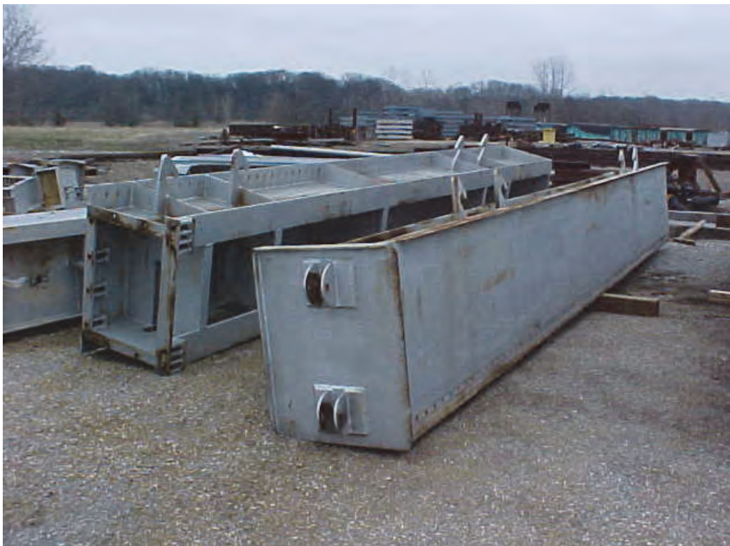
Figure 8. Stop logs used on the Steel Bayou Flood Control Drainage Structure. (Furnished by USAED Vicksburg.)
