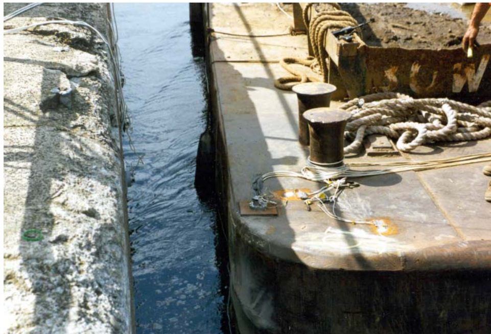
Figure 12. Accelerometer installed on top deck, located on the left side near edge of barge (gages are located at the two rusty spots on the barge deck, to the right of the accelerometer)
