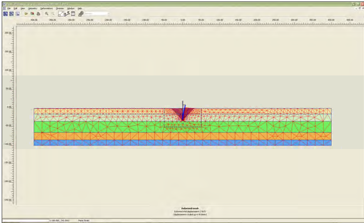
Figure 4.23. Total displacements for a water elevation of 13 ft and a gap tip elevation of 22 ft.
