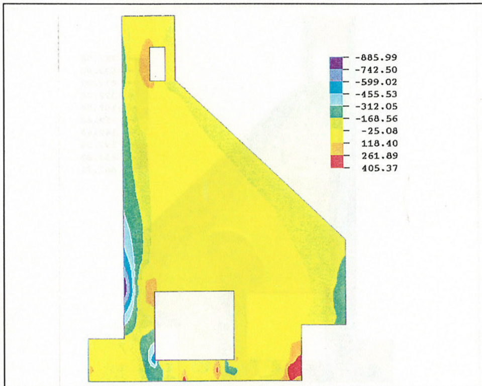
Figure 86. Vertical stress contour at day 615 of the extended analysis
