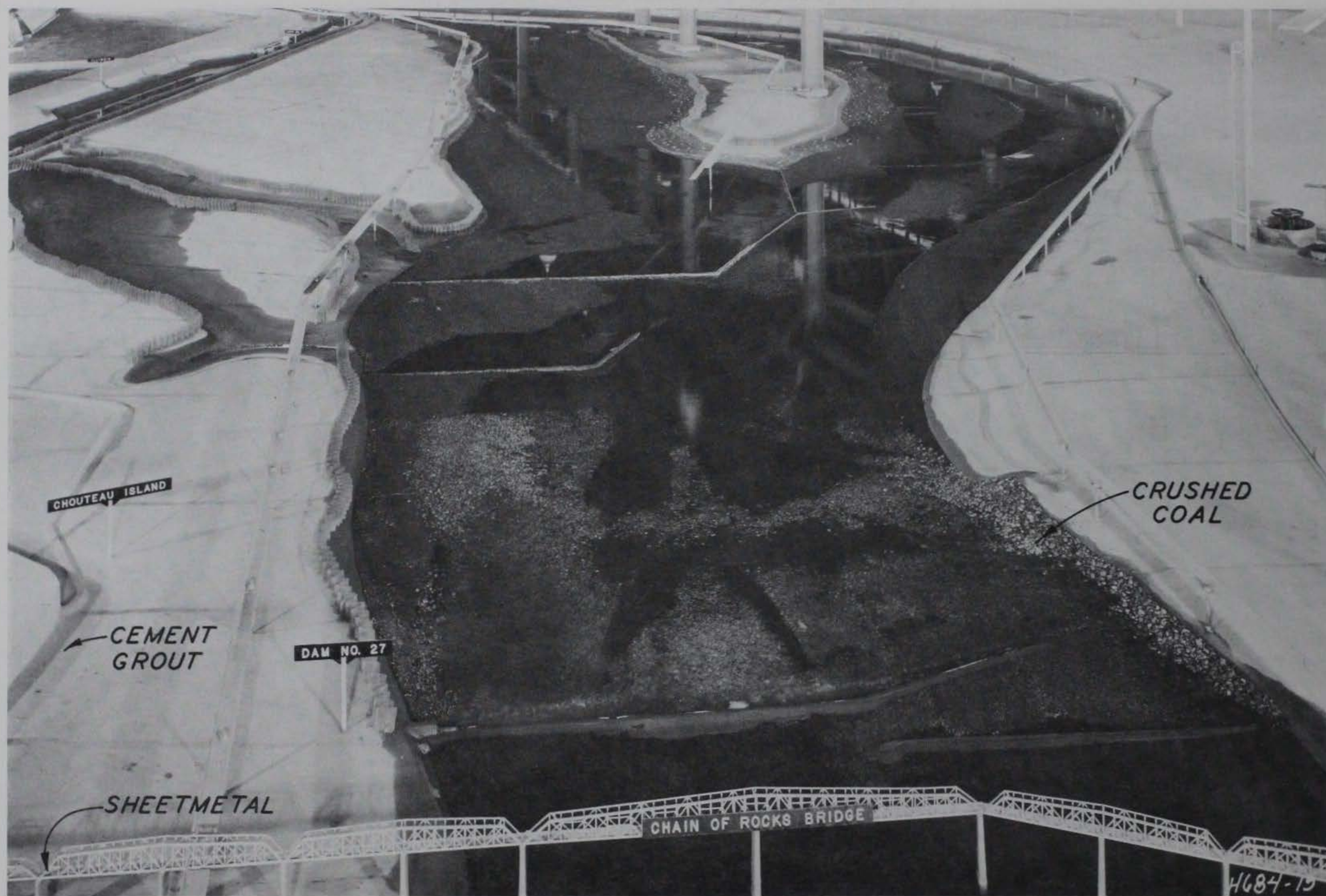
Photo 4. Cement grout with crushed coal, movable-bed navigation model
