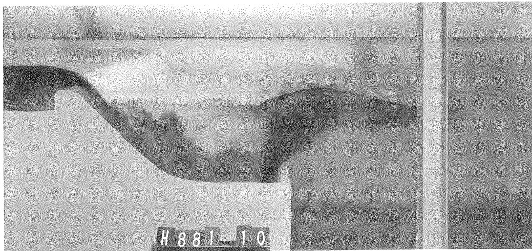
b. Discharge 50,000 cfs, tailwater el 776.5
