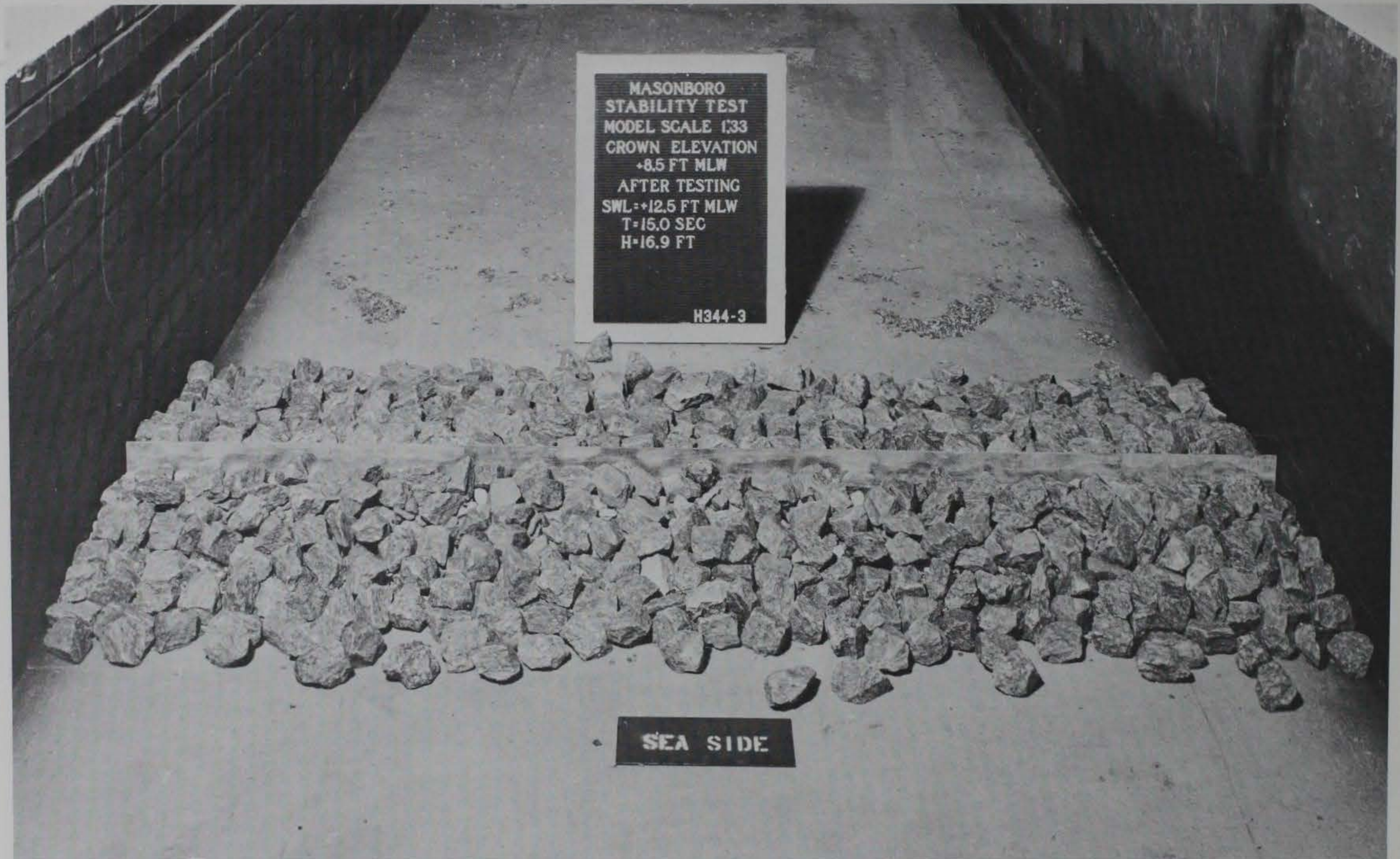
Photo 3. Sea-side view of Plan 1 after attack of 15-sec, 16.9-ft waves at an swl of +12.5 ft mlw for 4 prototype hr
