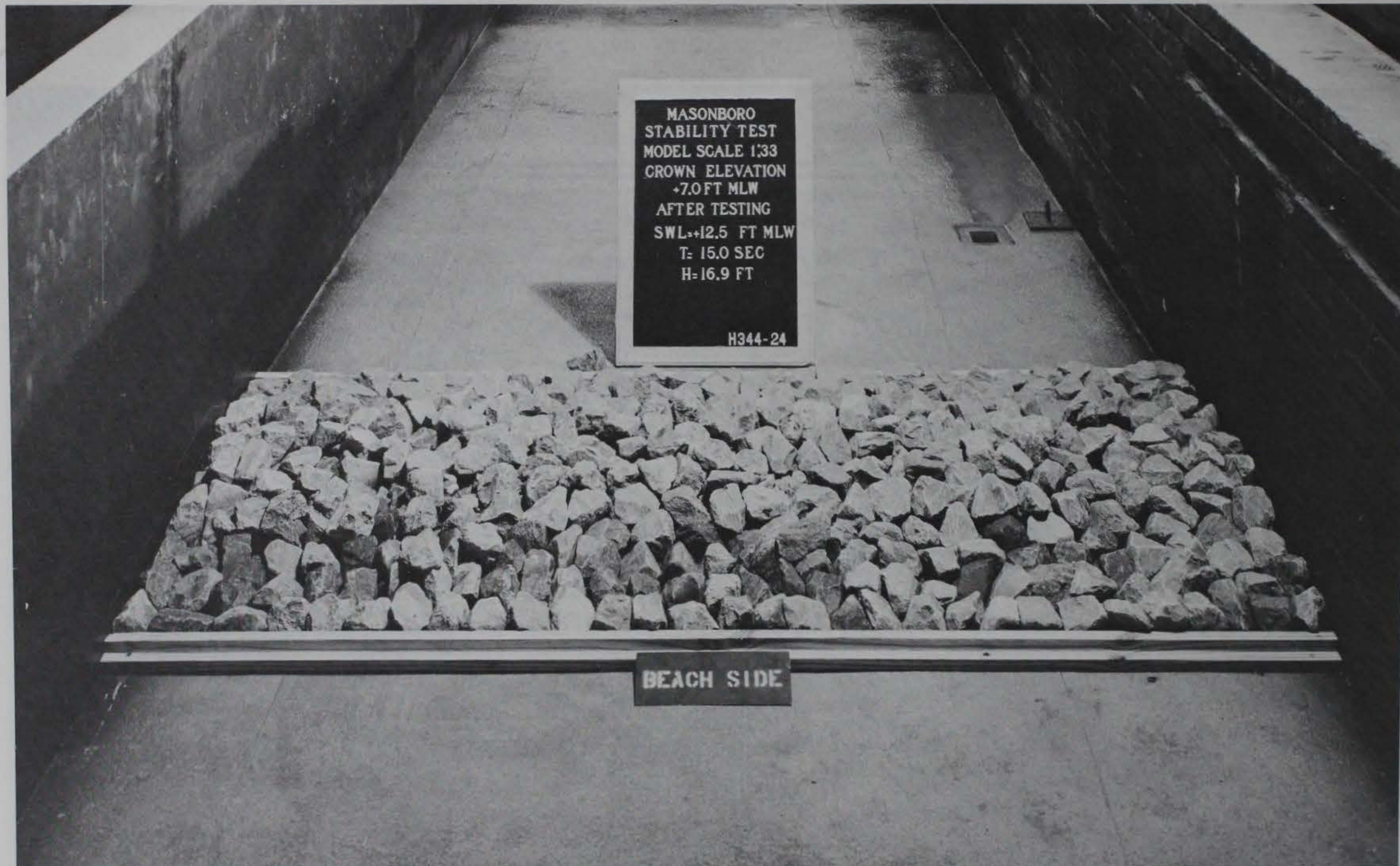
Photo 21. Beach-side view of Plan 3A after attack of 15-sec, 16.9-ft waves at an swl of +12.5 ft mlw for 2 prototype hr
