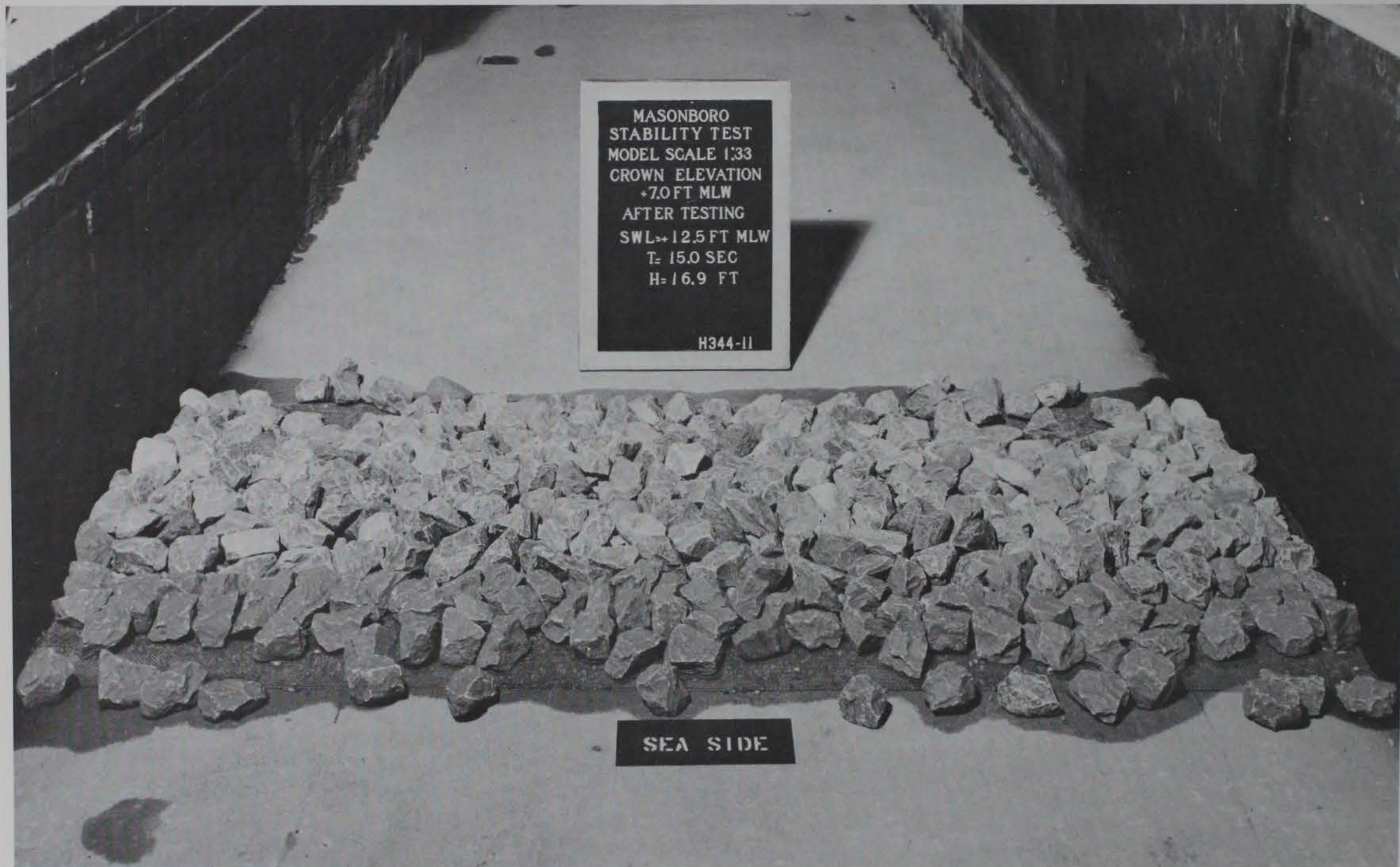
Photo 11. Sea-side view of Plan 3 after attack of 15-sec, 16.9-ft waves at an swl of +12.5 ft mlw for 2 prototype hr
