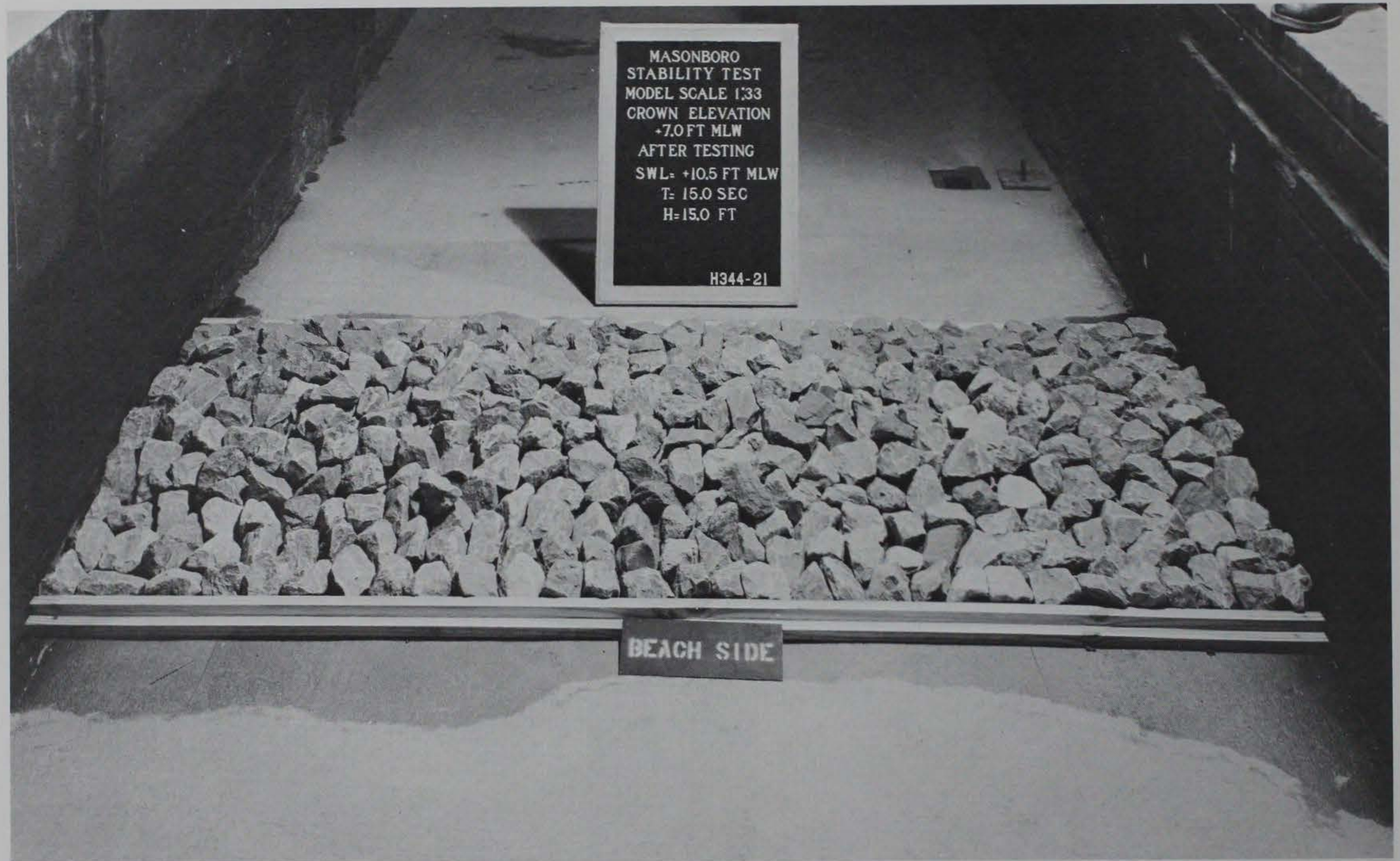
Photo 18. Beach-side view of Plan 3A after attack of 15-sec, 15-ft waves at an swl of +10.5 ft mlw for 2 prototype hr
