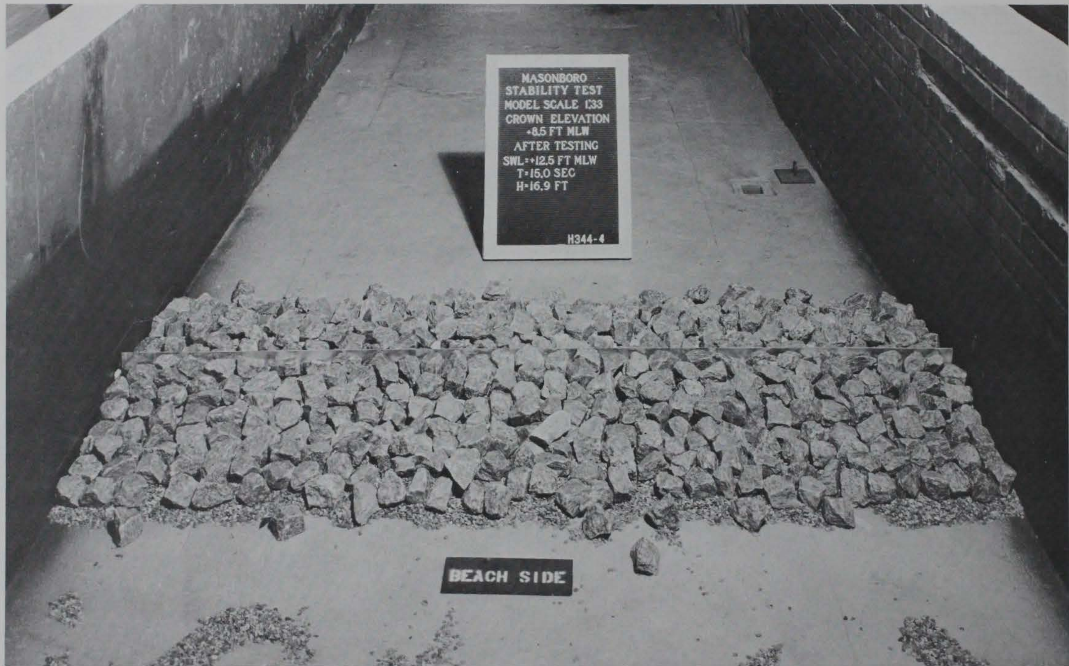
Photo 4. Beach-side view of Plan 1 after attack of 15-sec, 16.9-ft waves at an swl of +12.5 ft mlw for 4 prototype hr
