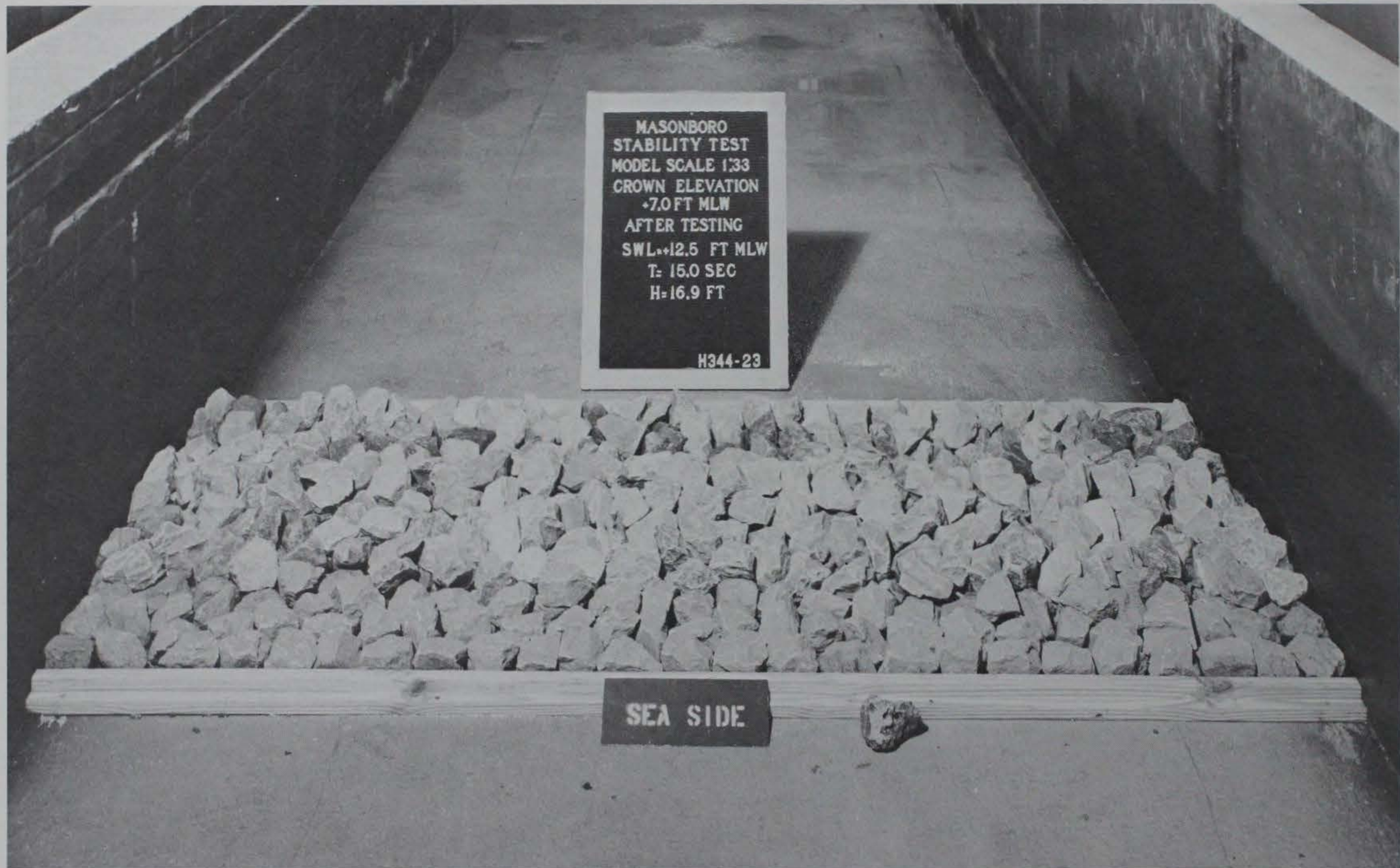
Photo 20. Sea-side view of Plan 3A after attack of 15-sec, 16.9-ft waves at an swl of +12.5 ft mlw for 2 prototype hr
