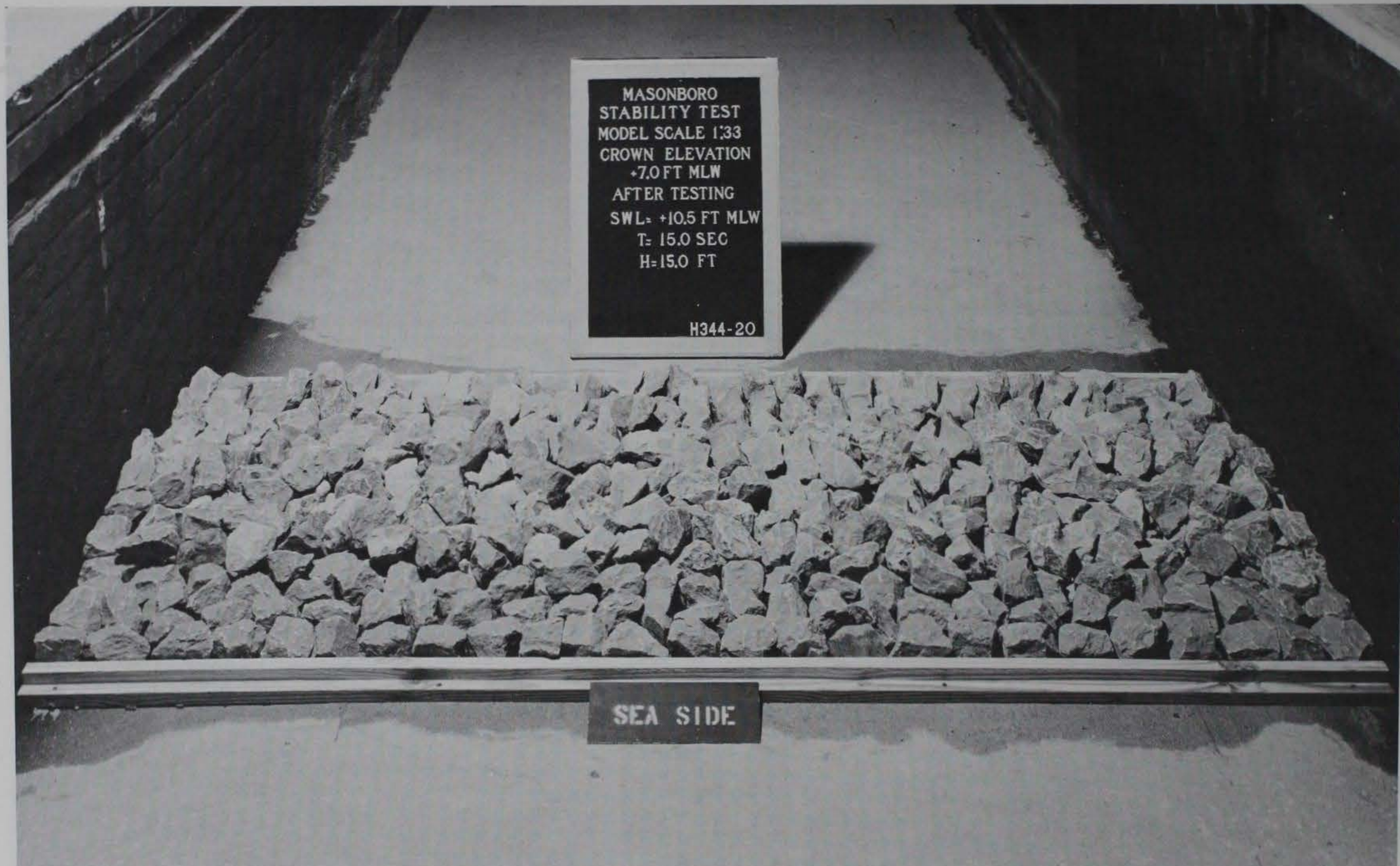
Photo 17. Sea-side view of Plan 3A after attack of 15-sec, 15-ft waves at an swl of +10.5 ft mlw for 2 prototype hr
