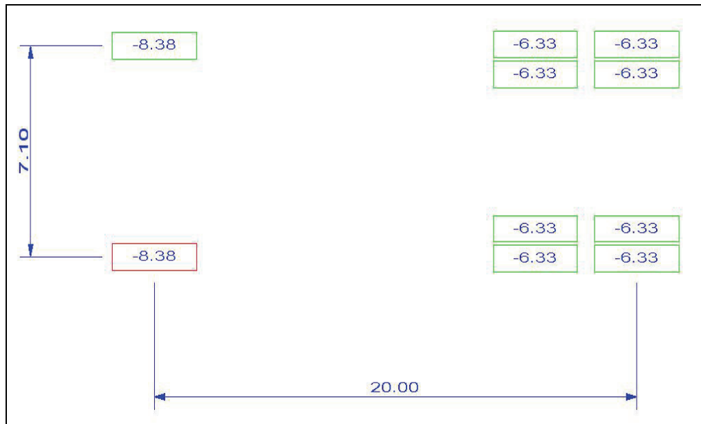
Figure 6. Foster Creek Bridge—preliminary load test truck configuration (ft-kips).
