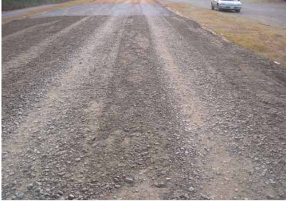
Photo C5. Item 3 (SST), dry lane, maintenance test section, 500 passes with pickup truck
