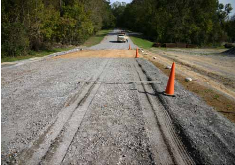
Photo C91. Item 7 (LST), dry lane, new construction test section, 10 passes with dump truck
