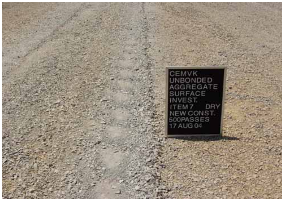
Photo C74. Item 7 (LST), dry lane, new construction test section, 500 passes with pickup truck
