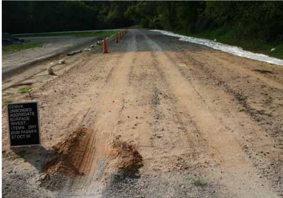
Photo C81. Item 6 (SCG), dry lane, new construction test section, 2500 passes with pickup truck
