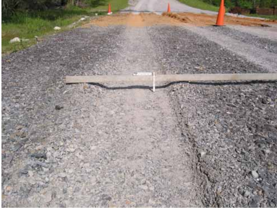
Photo C107. Item 7 (LST), wet lane, new construction test section, 25 passes with CBR truck
