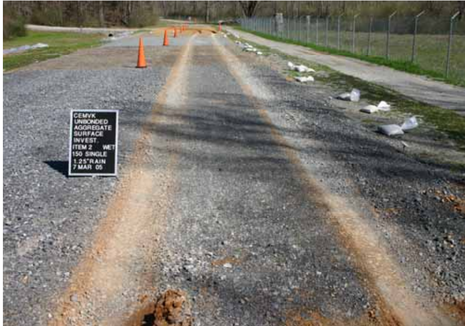
Photo C53. Item 2 (LST), wet lane, maintenance test section, 150 passes with pickup truck
