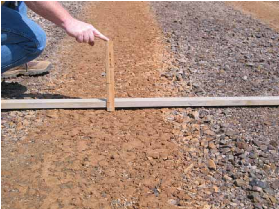
Photo C66. Item 3 (SST), wet lane, maintenance test section, 50 passes with CBR truck
