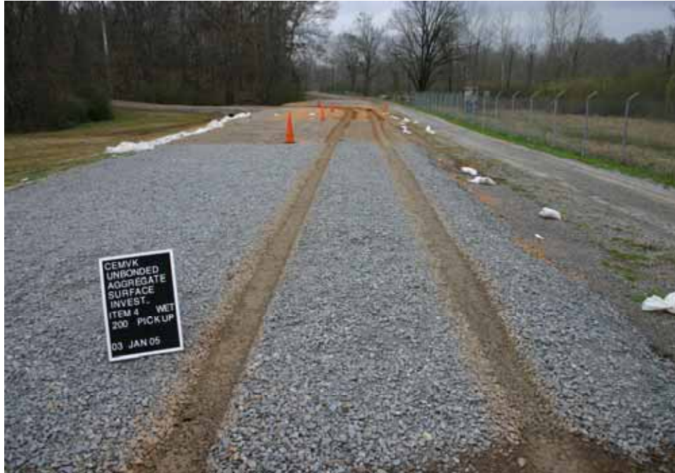
Photo C37. Item 4 (IGN), wet lane, maintenance test section, 200 passes with pickup truck
