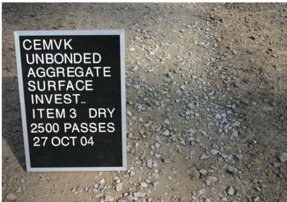
Photo C16. Item 3 (SST), dry lane, maintenance test section, 2500 passes with pickup truck
