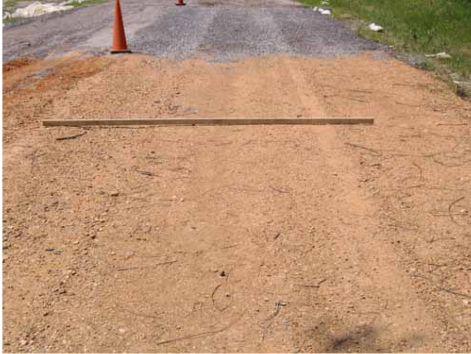
Photo C97. Item 6 (SCG), wet lane, new construction test section, 25 passes with pickup truck
