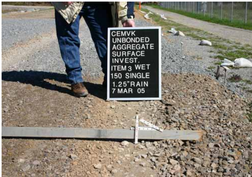
Photo C56. Item 3 (SST), wet lane, maintenance test section, 150 passes with pickup truck
