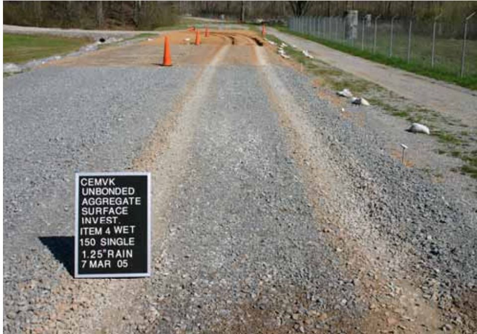
Photo C57. Item 4 (IGN), wet lane, maintenance test section, 150 passes with pickup truck
