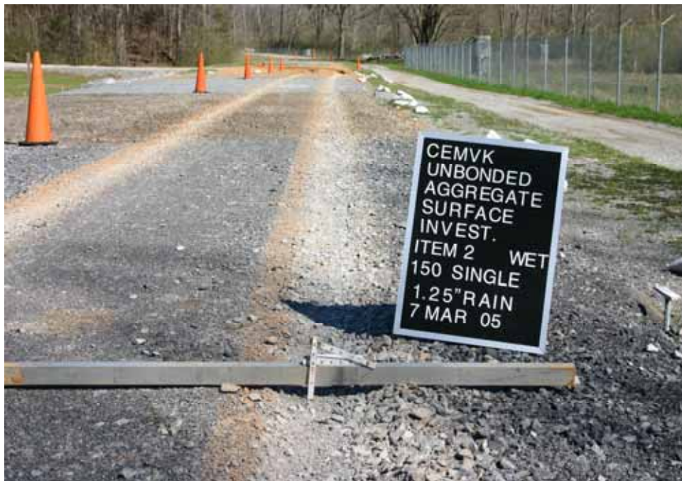
Photo C54. Item 2 (LST), wet lane, maintenance test section, 150 passes with pickup truck
