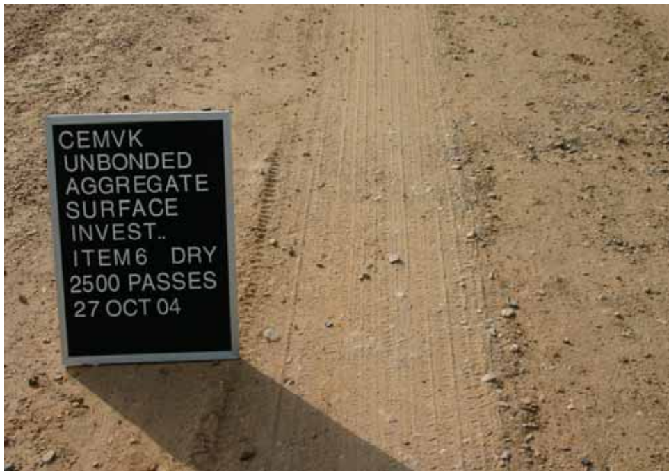
Photo C82. Item 6 (SCG), dry lane, new construction test section, 2500 passes with pickup truck
