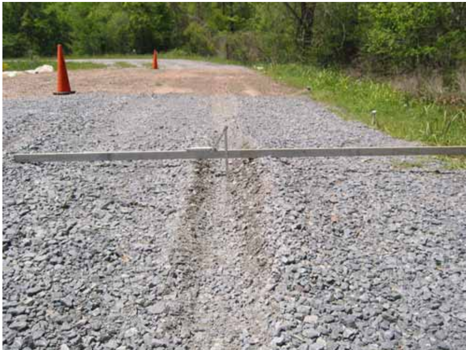
Photo C102. Item 9 (IGN), wet lane, new construction test section, 25 passes with pickup truck
