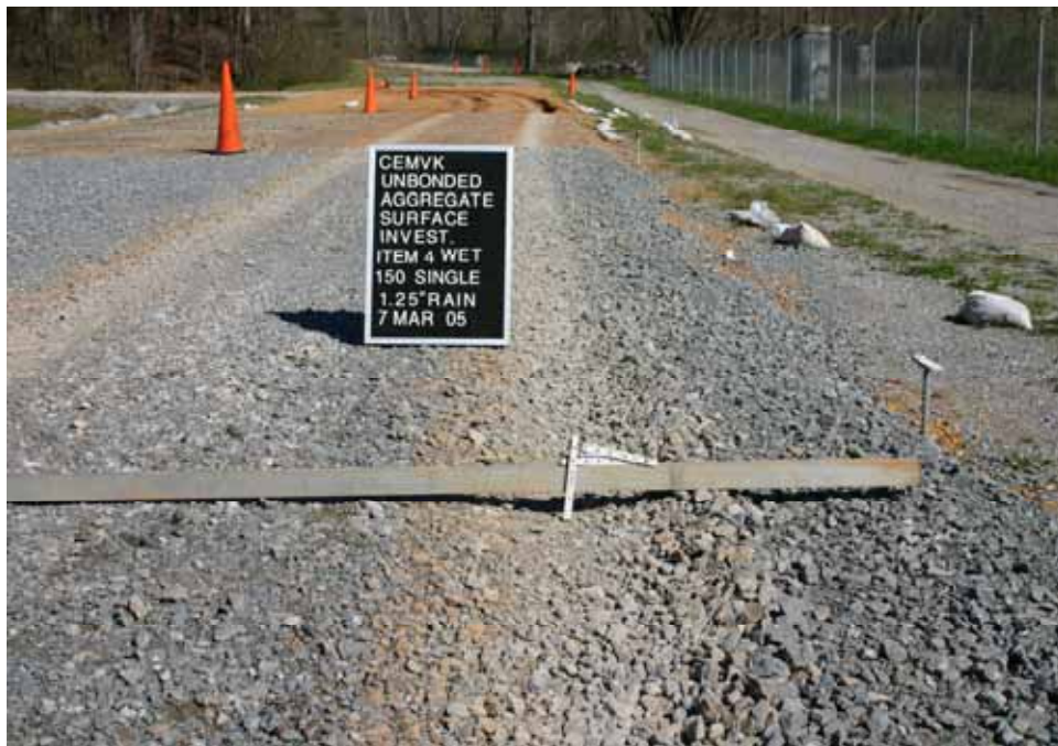
Photo C58. Item 4 (IGN), wet lane, maintenance test section, 150 passes with pickup truck
