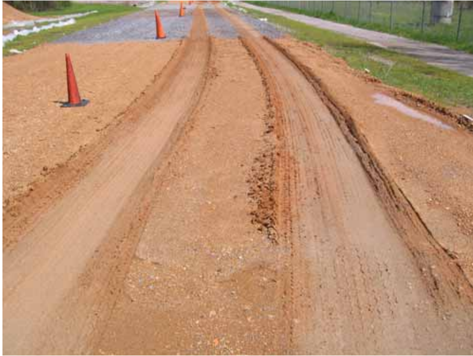
Photo C61. Item 1 (SCG), wet lane, maintenance test section, 50 passes with CBR truck
