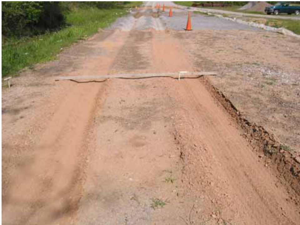
Photo C112. Item 10 (SSB), wet lane, new construction test section, 25 passes with CBR truck
