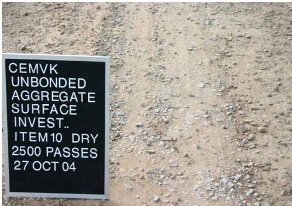
Photo C90. Item 10 (SSB), dry lane, new construction test section, 2500 passes with pickup truck
