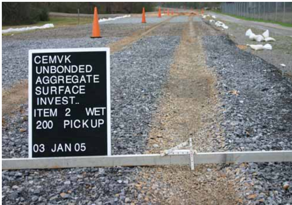
Photo C34. Item 2 (LST), wet lane, maintenance test section, 200 passes with pickup truck
