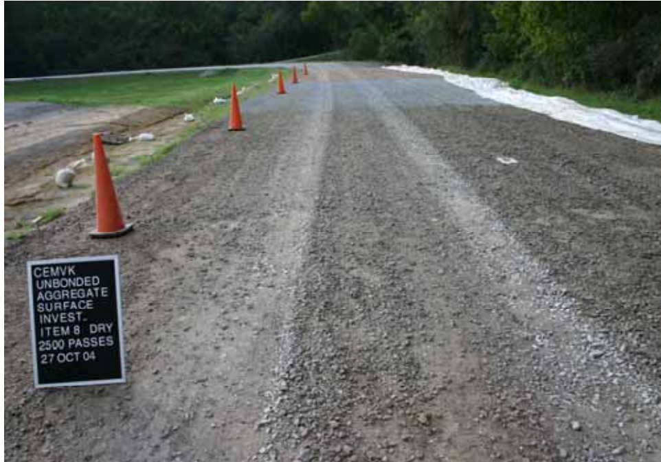
Photo C85. Item 8 (SST), dry lane, new construction test section, 2500 passes with pickup truck
