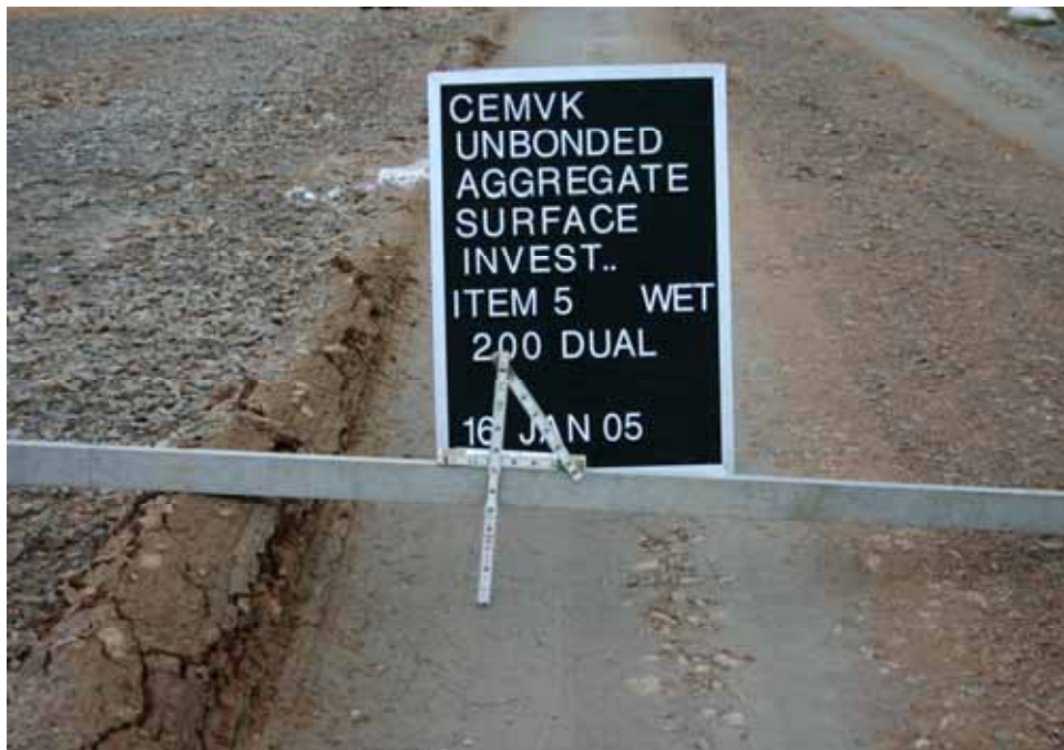
Photo C50. Item 5 (SSB), wet lane, maintenance test section, 200 passes with dump truck
