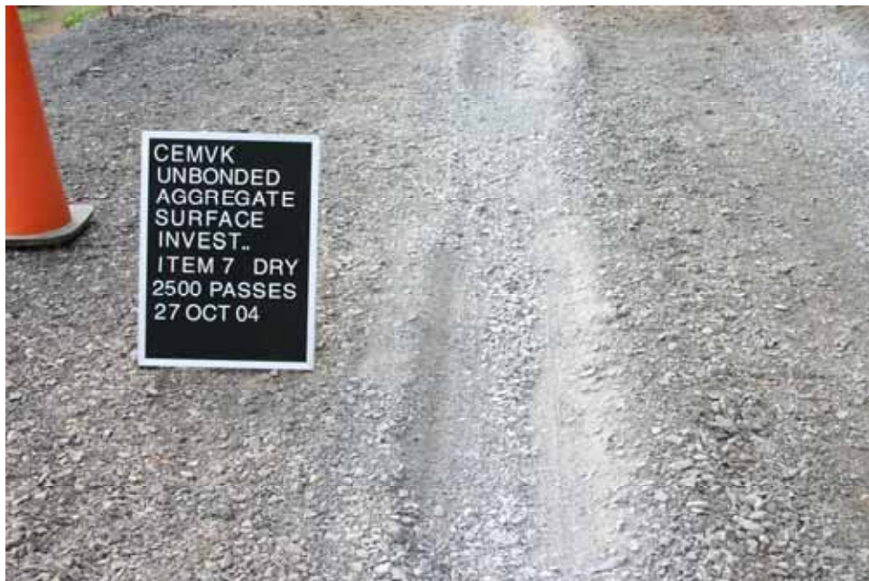
Photo C84. Item 7 (LST), dry lane, new construction test section, 2500 passes with pickup truck
