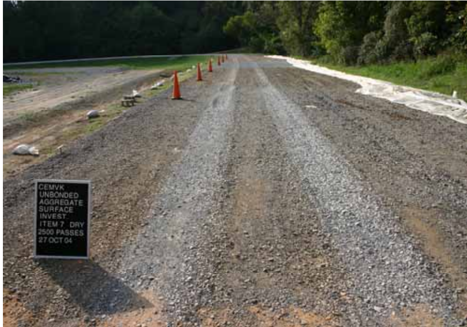
Photo C83. Item 7 (LST), dry lane, new construction test section, 2500 passes with pickup truck
