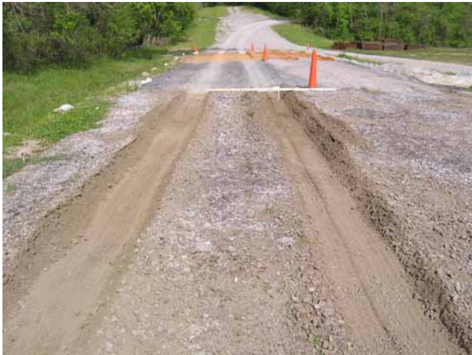
Photo C108. Item 8 (SST), wet lane, new construction test section, 25 passes with CBR truck
