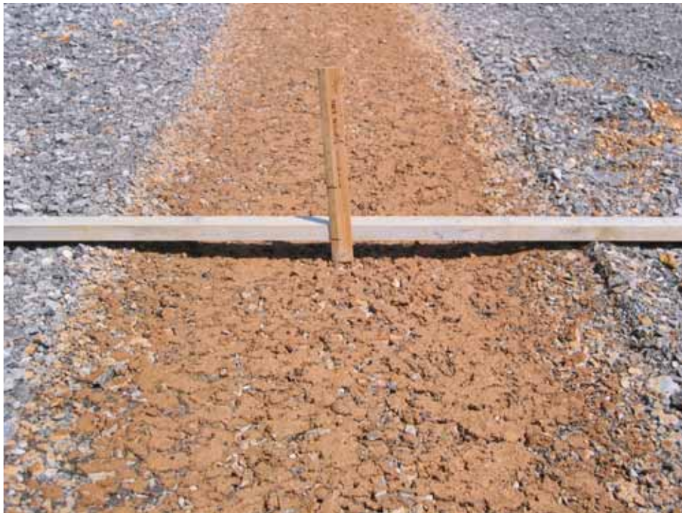
Photo C64. Item 2 (LST), wet lane, maintenance test section, 50 passes with CBR truck
