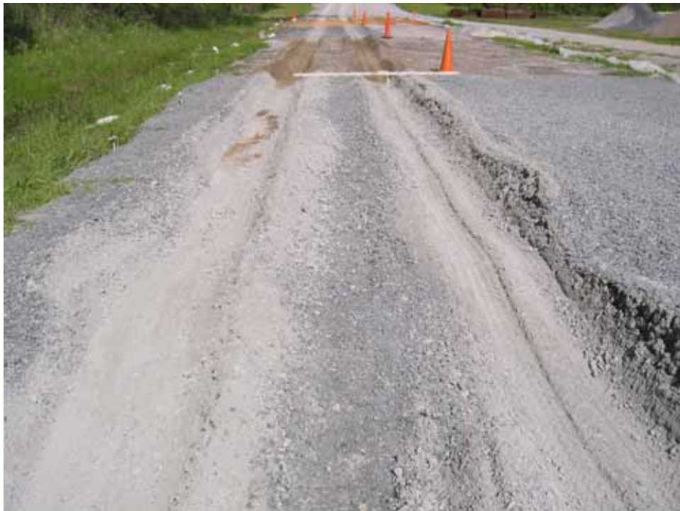
Photo C110. Item 9 (IGN), wet lane, new construction test section, 25 passes with CBR truck
