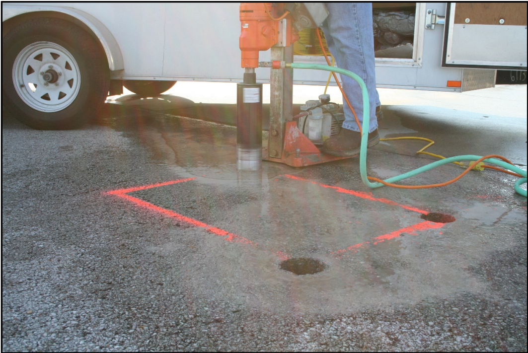
Figure 3. AC core sampling.
