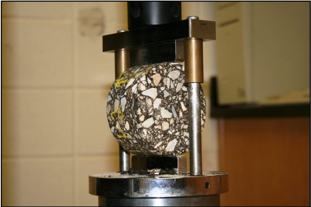
Figure 10. Before an ITS test on the Instron machine.
