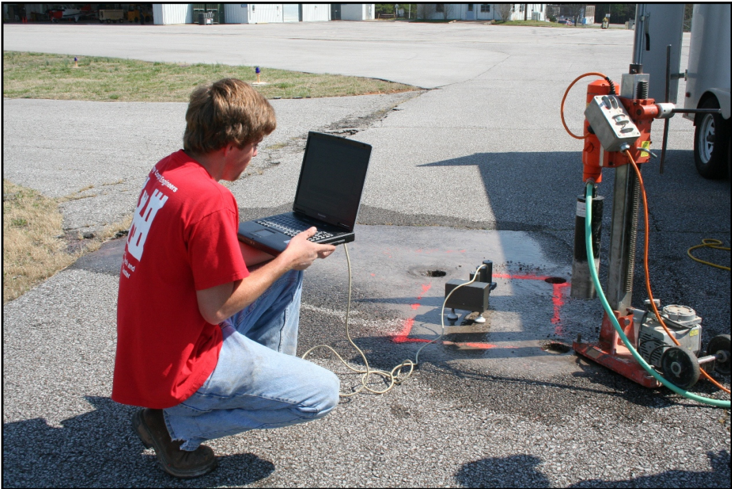
Figure 4. Obtaining the in situ pavement modulus using the PSPA.
