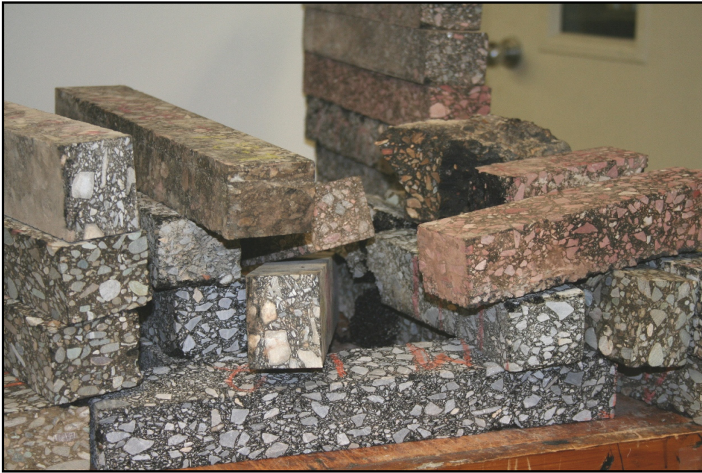
Figure 14. Sawed beams after fatigue testing.
