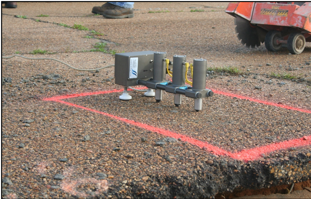
Figure 9. Portable seismic pavement analyzer.
