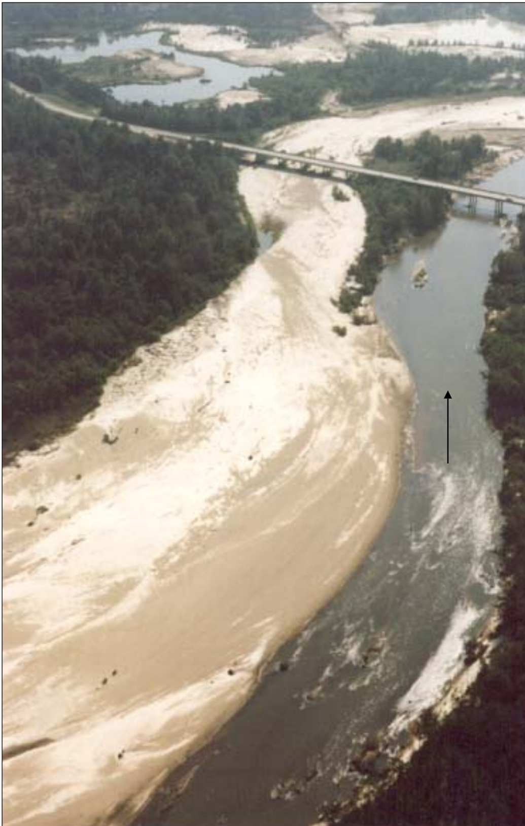
Figure 40. 1995 downstream view of the Amite River at the Louisiana Hwy 37 crossing near Grangeville, LA, showing abandoned riverbed (Meadows and Patrick 1999) (arrow notes flow direction).
