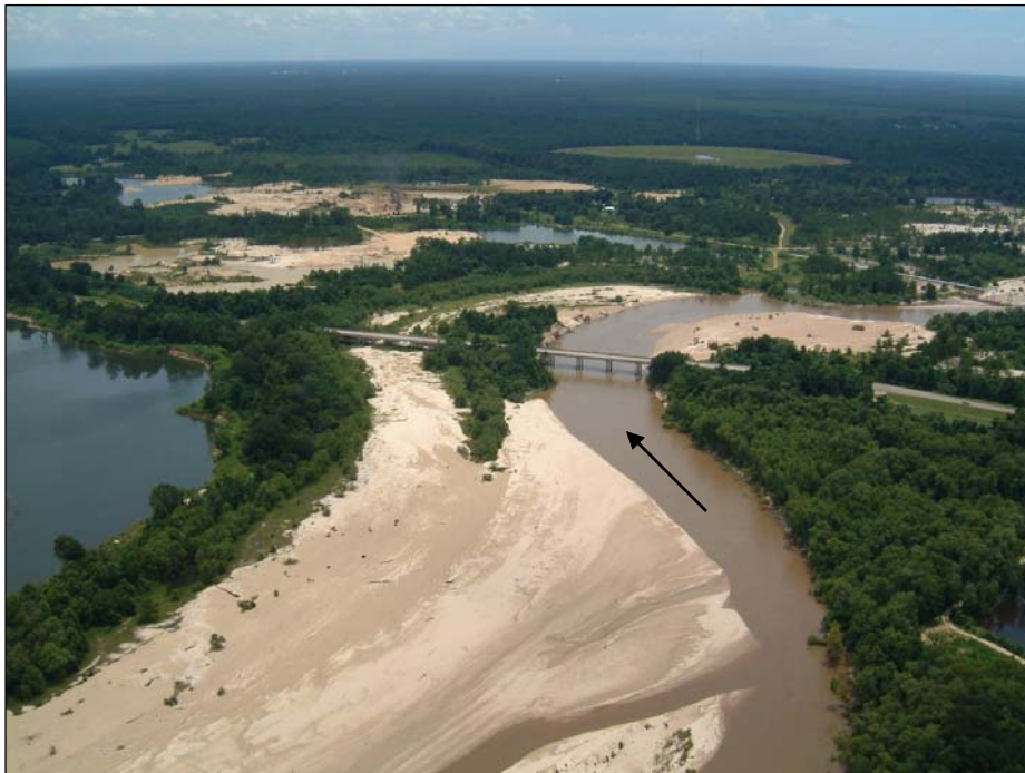
Figure 39. Downstream view of the Amite River at the Louisiana Hwy 37 crossing near Grangeville, LA (note large, dry abandoned channel at left bank—July 2004) (arrow notes flow direction).
