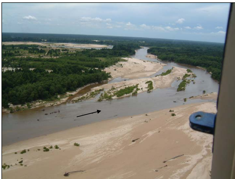
Figure 37. Divided flow conditions of the Amite River just upstream of the Louisiana Hwy 37 crossing near Grangeville, LA (view is downstream—July 2004) (arrow notes flow direction).
