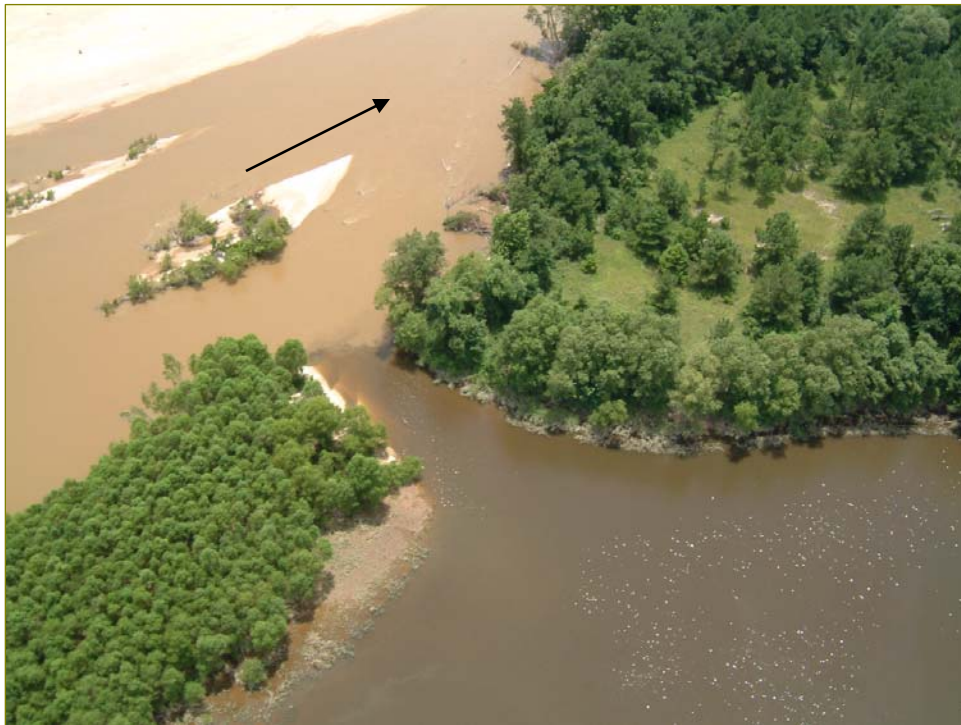
Figure 60. Downstream view of breached right bank of the Amite River near Magnolia, LA (July 2004) (arrow notes flow direction).
