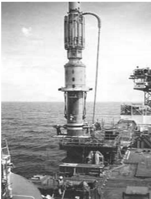
Figure 56. Menck 500T underwater hammer (after Menck 1999)
