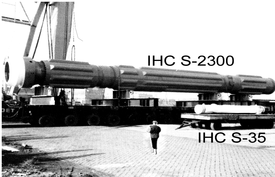
Figure 58. IHC underwater hammers (after IHC 1999)
