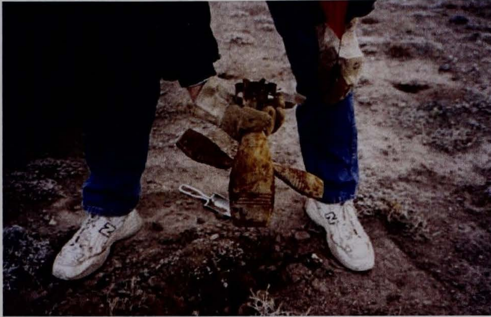
Figure 13: One of the practice 81-mm mortars deformed due to the detonation of the spotting charge.
