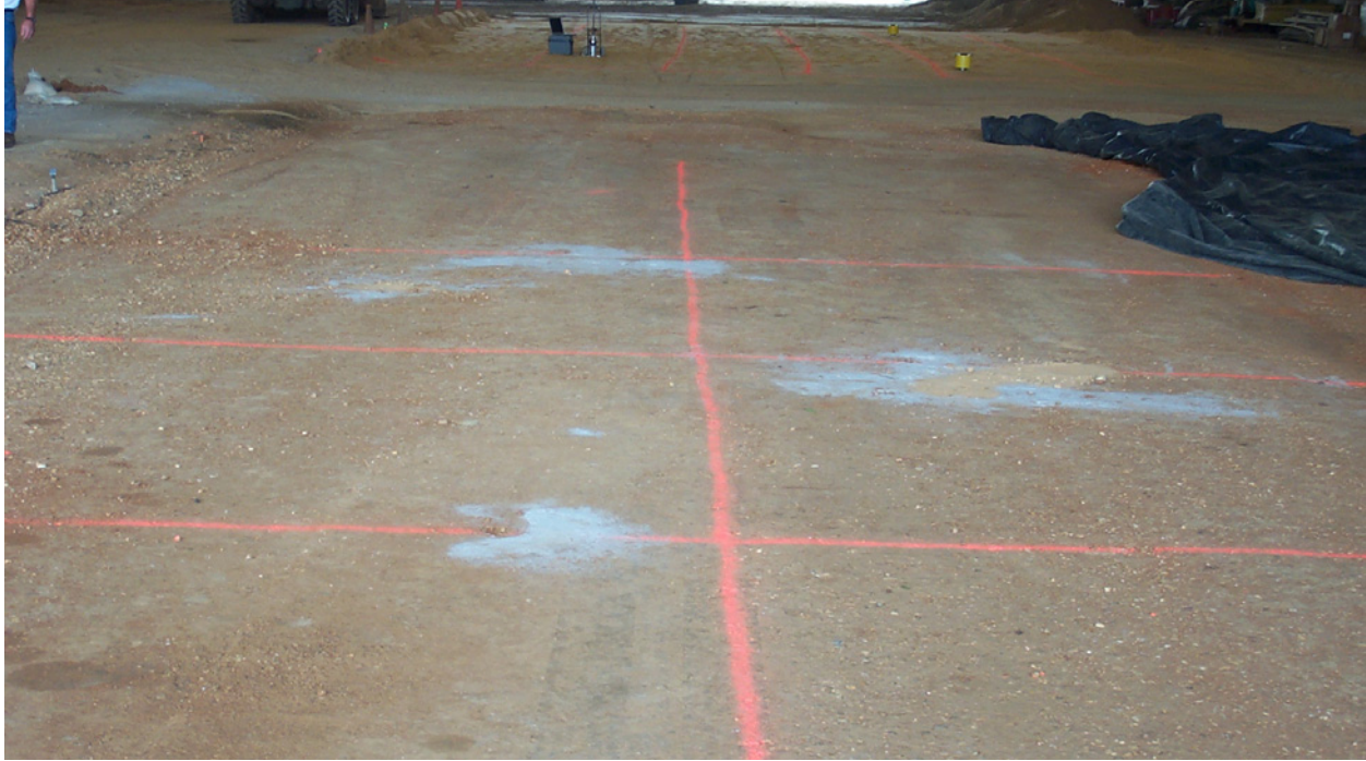
Photo 32. Unsurfaced control test section (high subgrade strength) is complete and awaits traffic
