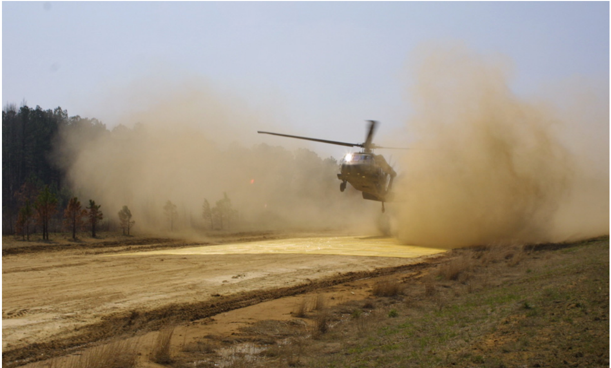
Photo 25. MP Mat helipad diffusing dust cloud as UH-60 Blackhawk approaches helipad
