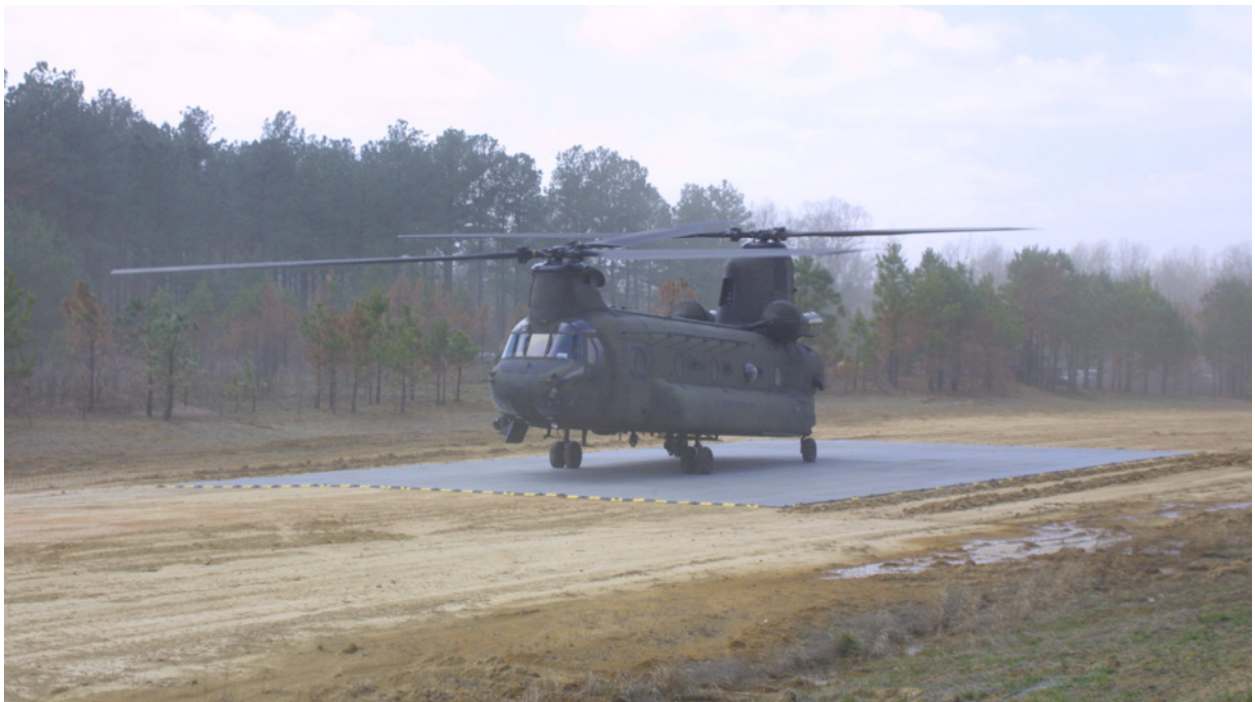
Photo 23. CH-47 Chinook operating on SUPA-TRAC helipad
