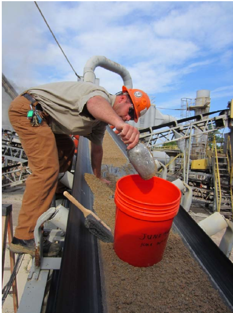
Figure 28. Sampling aggregate from feed belt at asphalt plant.
