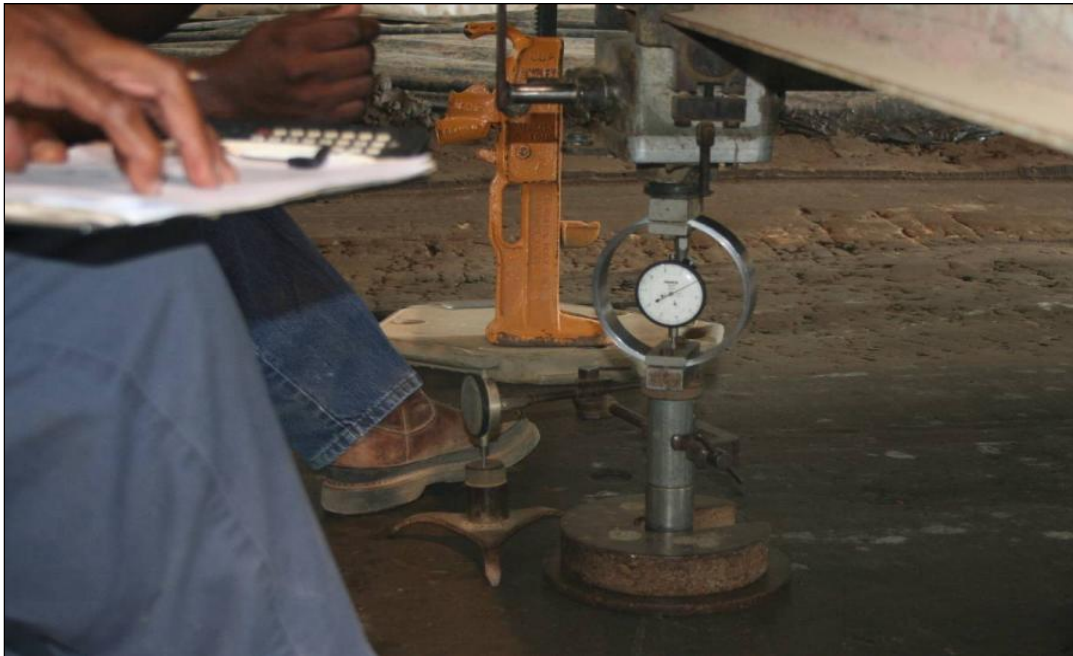
Figure 25. In situ CBR test.
