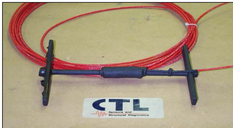
Figure 55. Asphalt strain gauge.
