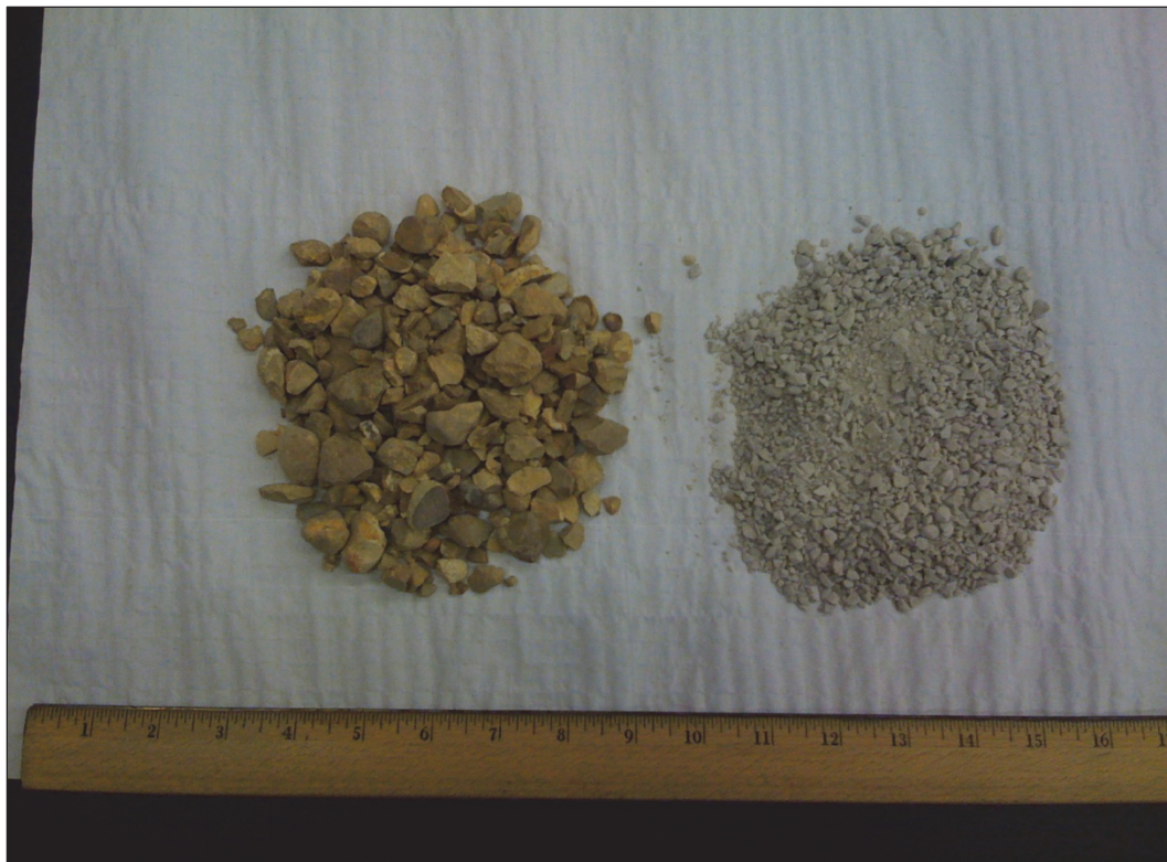
Figure 23. Material included in the subbase blended mix: crushed aggregate (left) and crushed limestone (right).
