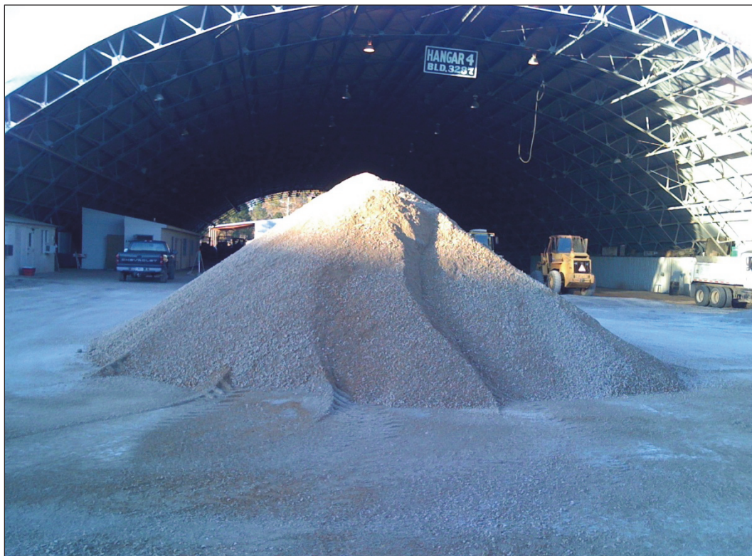
Figure 24. Blended subbase material stockpile.
