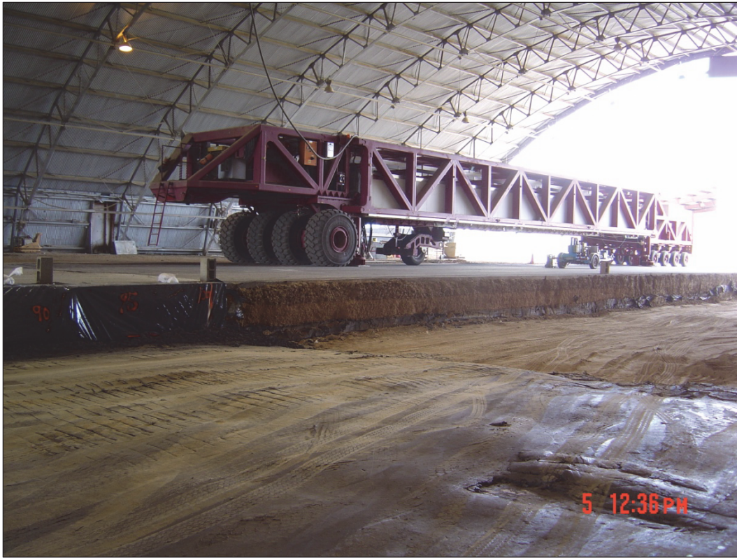
Figure 38. Heavy Vehicle Simulator (HVS-A) used for traffic testing.
