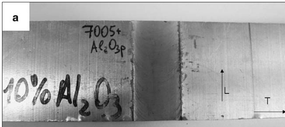
Figure 29. Friction-stir welded 7005 particle reinforced \text{Al}_2\text{O}_3 (Ceschini et al. 2007).
