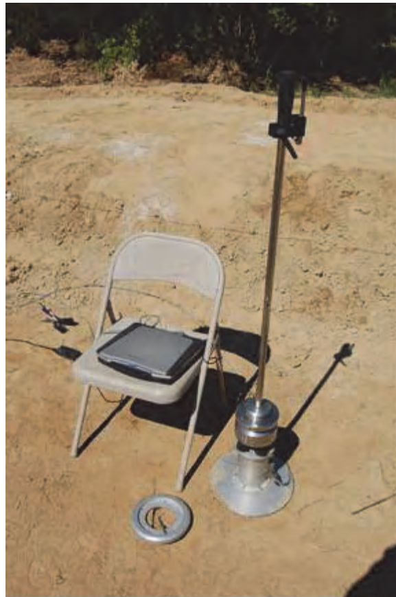
Figure 7. Dynatest Lightweight Deflectometer (D-LWD) requiring laptop and hardwire connection.
