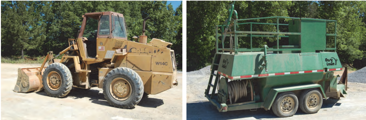
Figure 16. Front-end loader and hydroseeder used in preparing soils for compaction.
