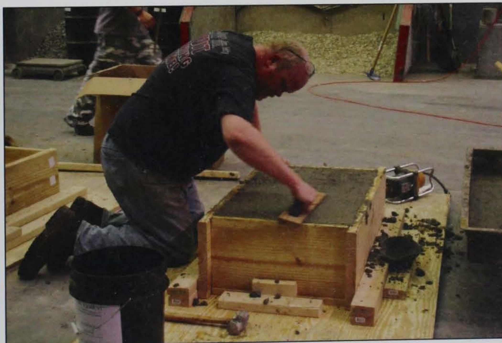
Figure 9. Finishing a laboratory-prepared concrete slab.
