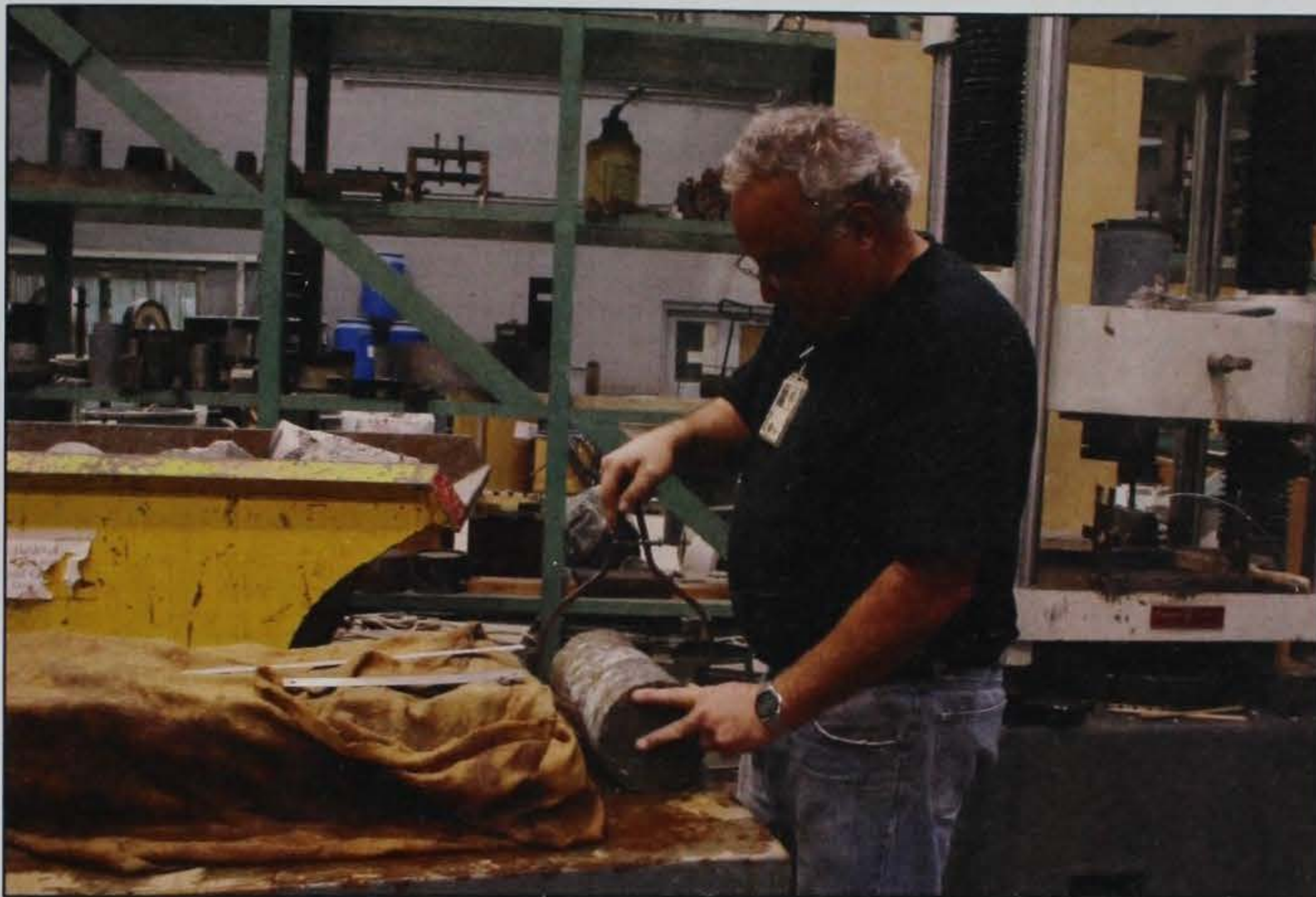
Figure 16. Measuring a core sample before splitting tensile strength testing.
