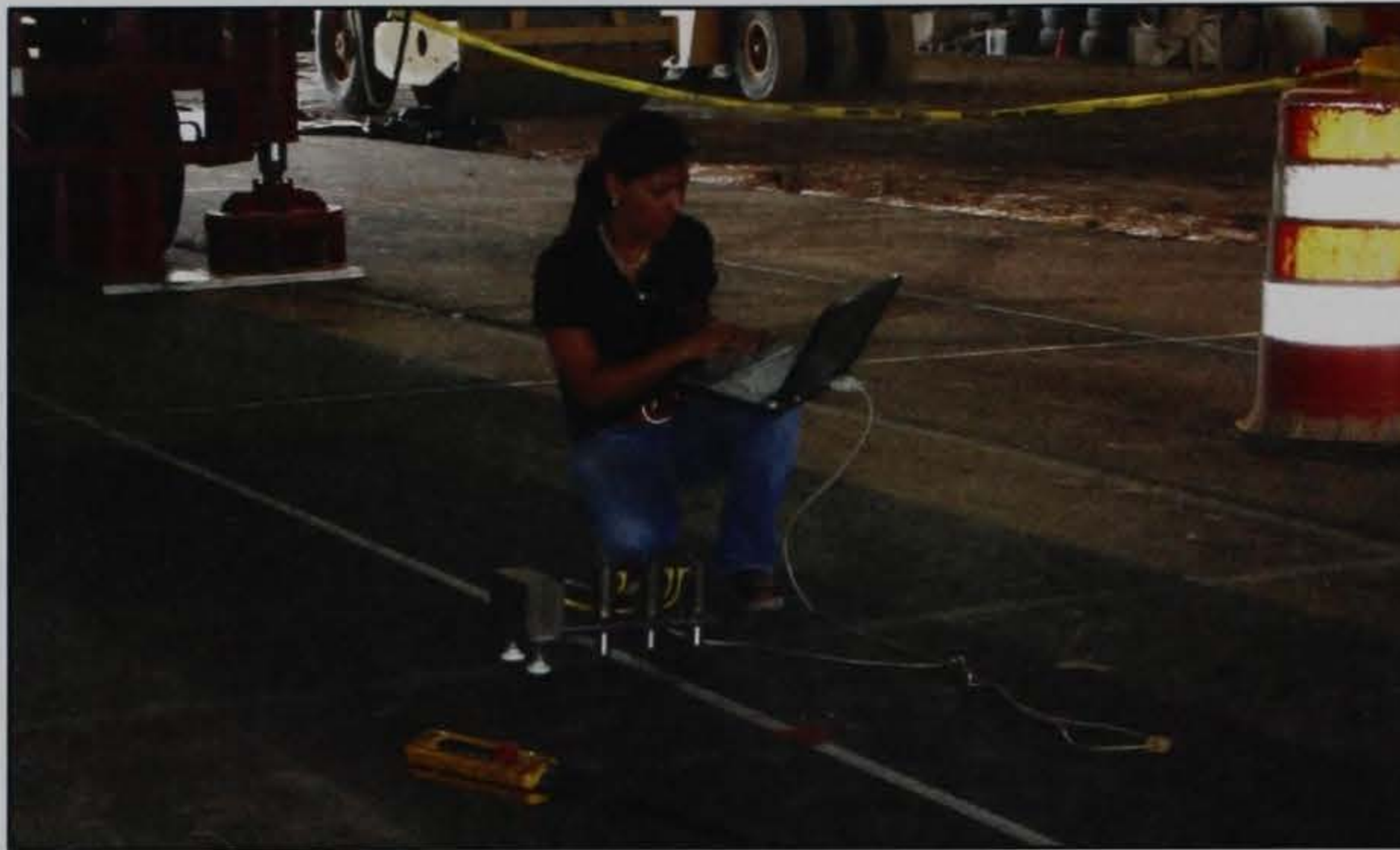
Figure 1. Operating the PSPA on an asphalt concrete test section.
