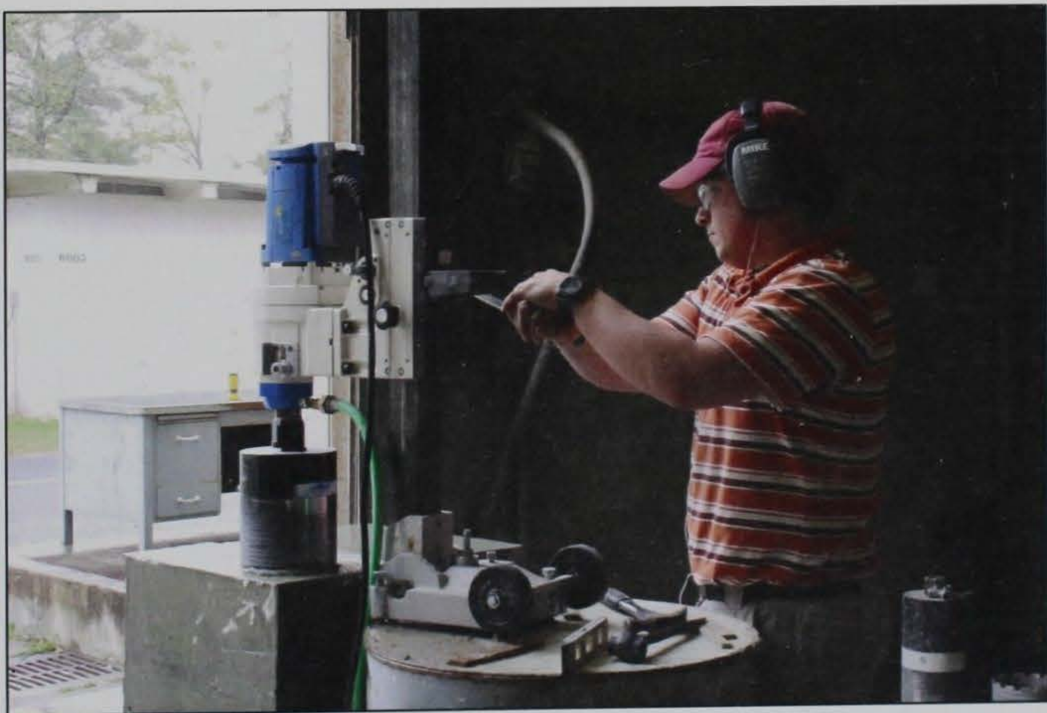
Figure 13. Sawing cylindrical specimens for splitting tensile strength testing.
