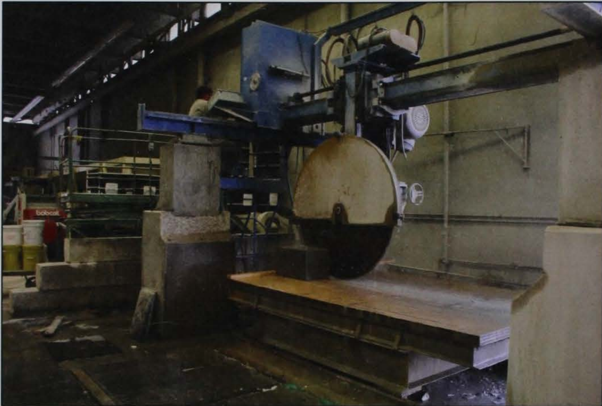
Figure 14. Sawing beam specimens for flexural strength testing.
