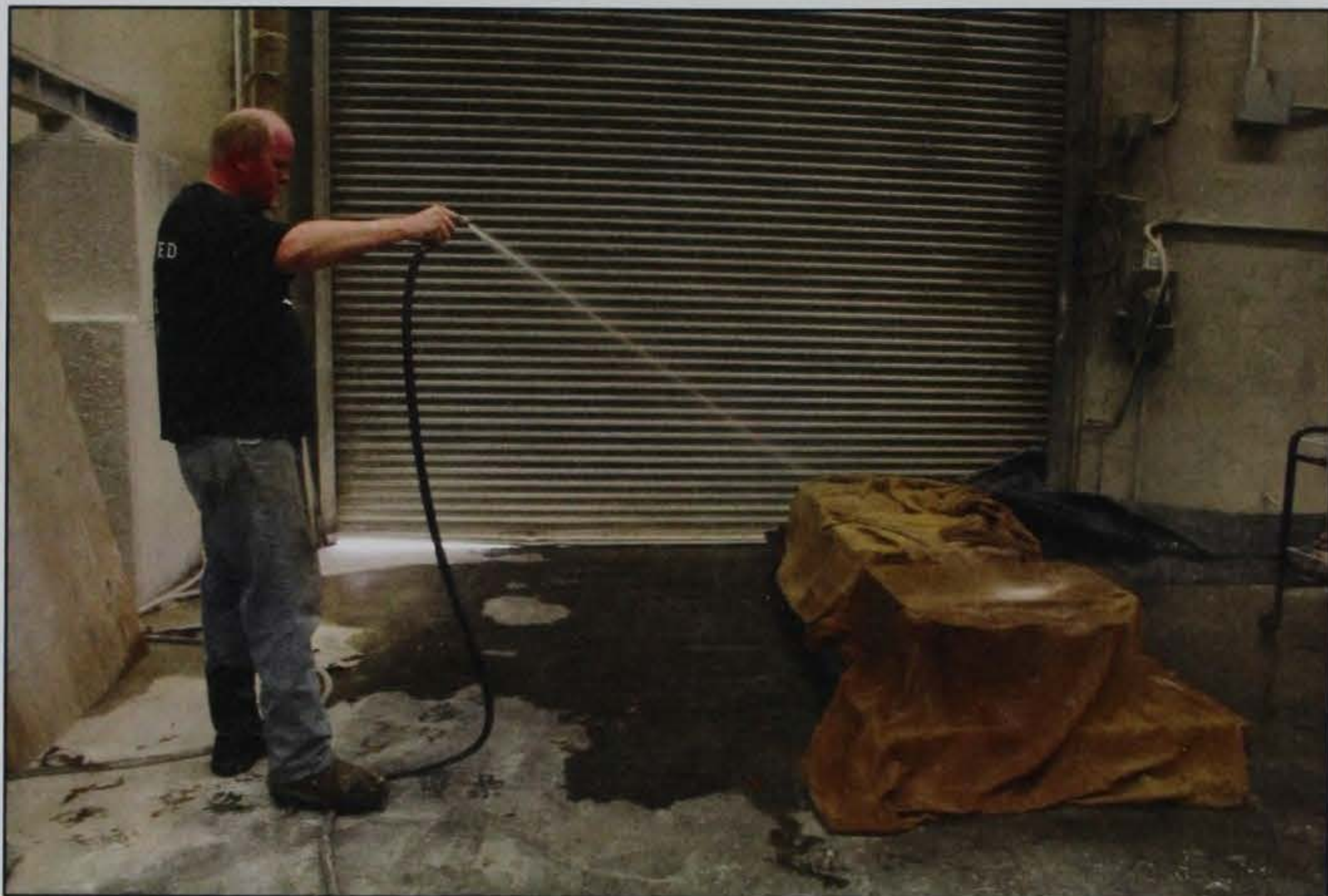
Figure 10. Keeping slabs moist before transporting to the fog room.
