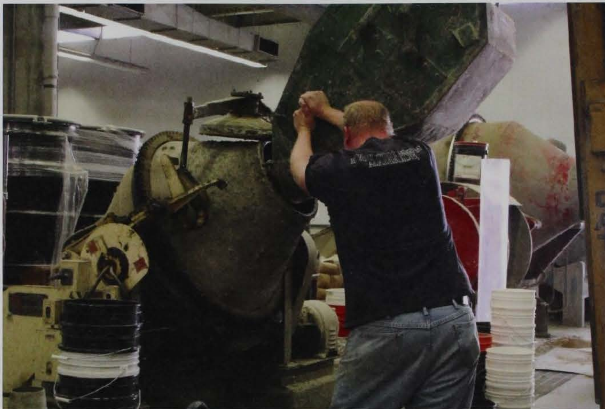
Figure 6. Pouring aggregate into the mixing barrel.
