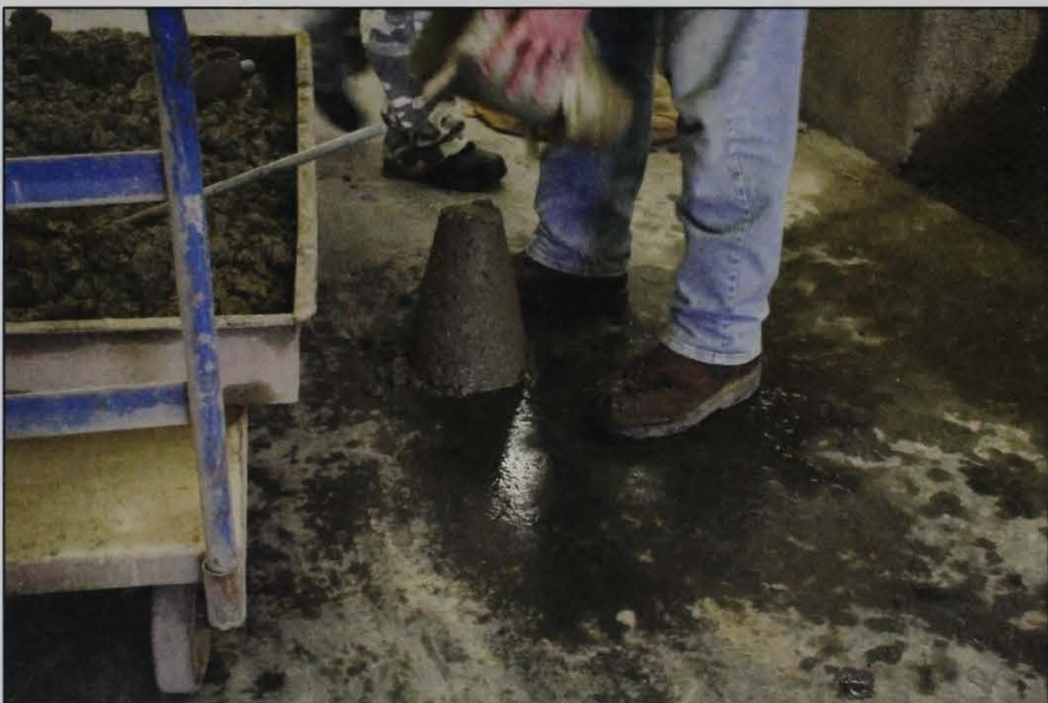
Figure 7. Performing a slump test on a concrete mixture.
