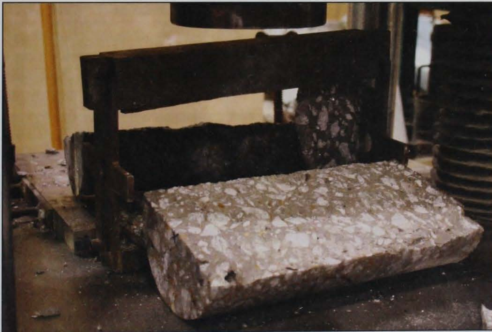
Figure 17. Core sample after splitting tensile strength testing.
