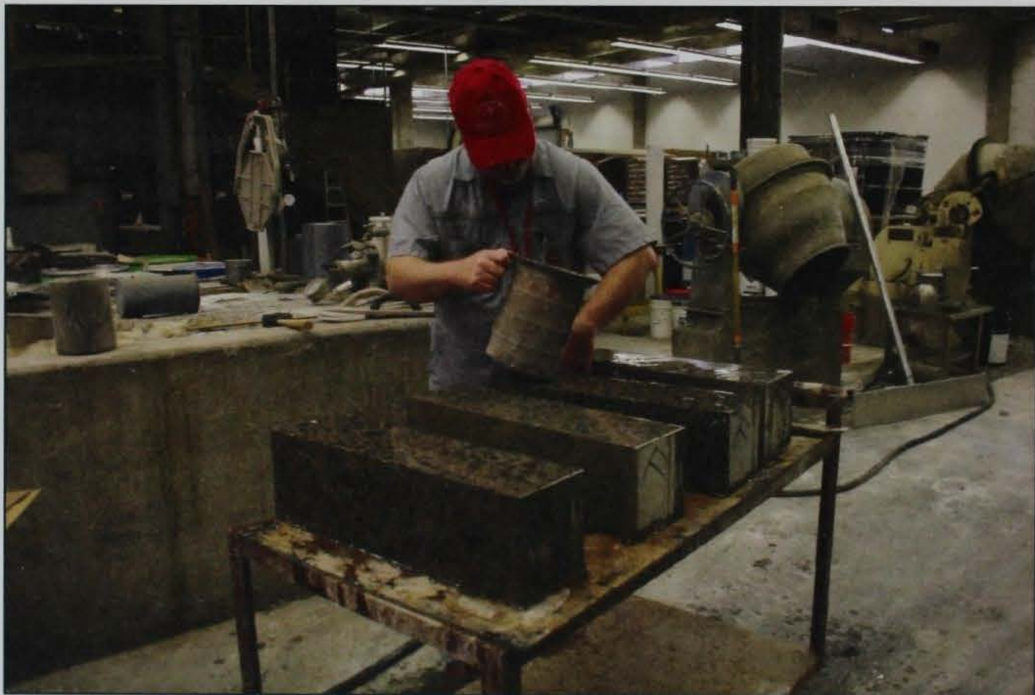
Figure 15. Keeping beam specimens moist before flexural strength testing.
