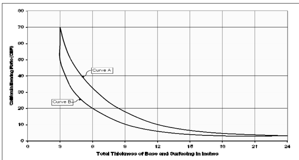
Figure 1. Total thickness of base and surfacing in relation to CBR values (after Porter).
