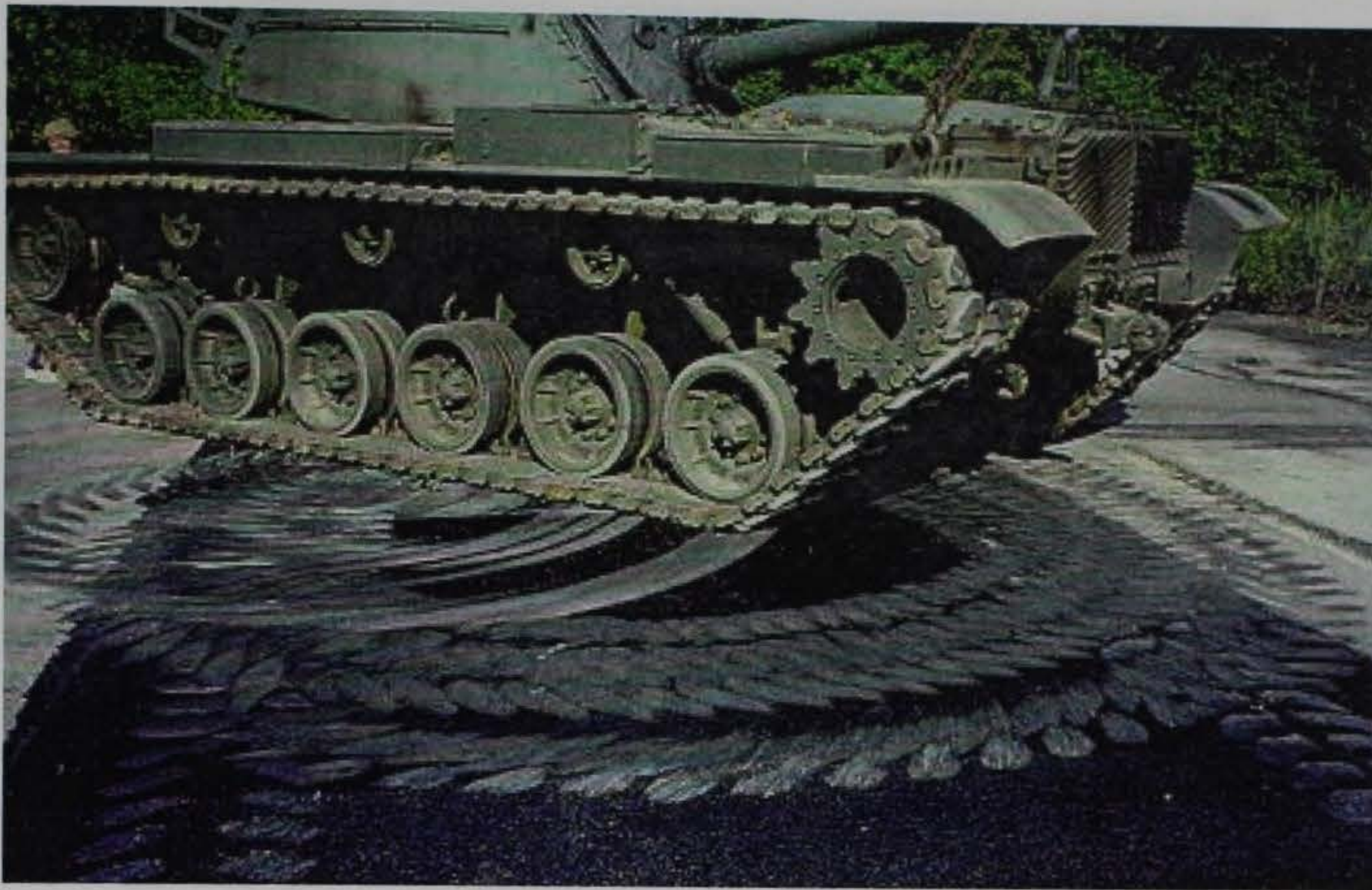
Figure 3. 106,000-lb M-60 tank conducting pivot steers on E-Krete surface at ERDC
