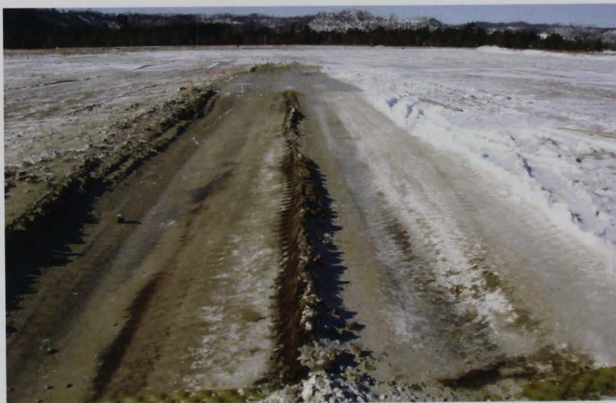
Figure 56. SC-2 control after 2,000 passes.
