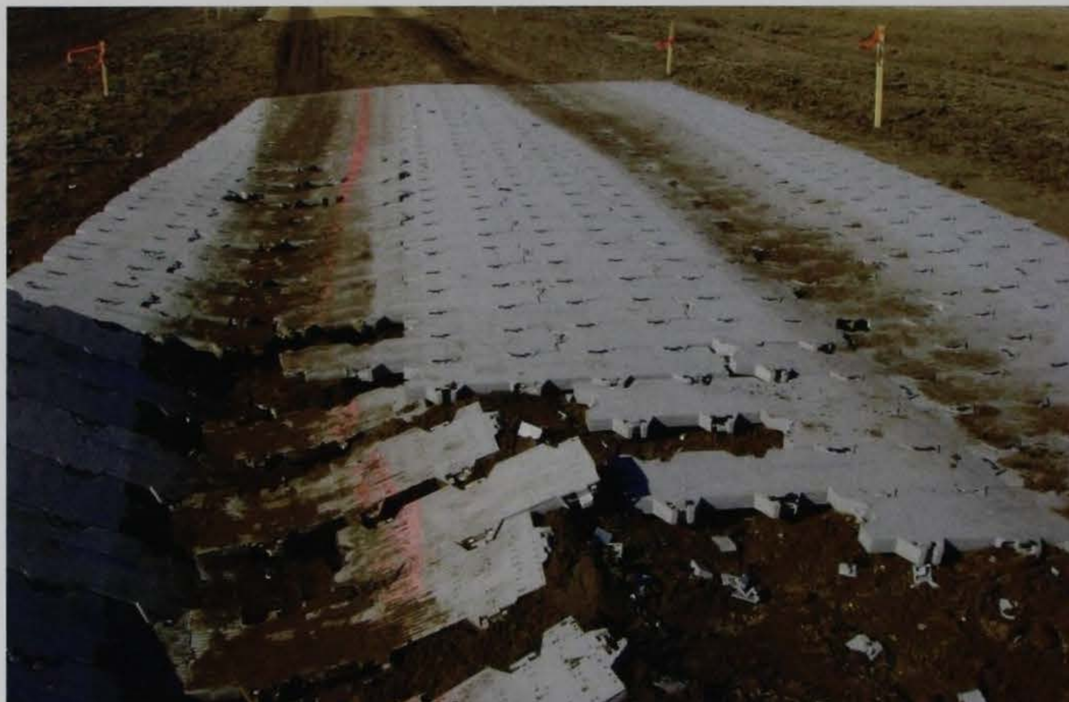
Figure 66. SC-1 test section after 146 passes
