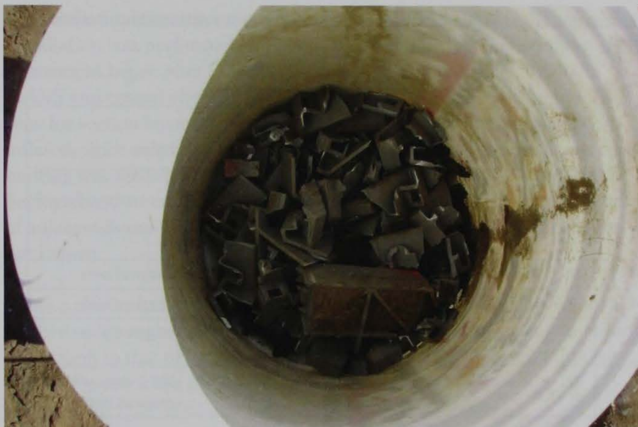
Figure 69. Bucket full of broken pieces of Supa-Trac collected after removal.
