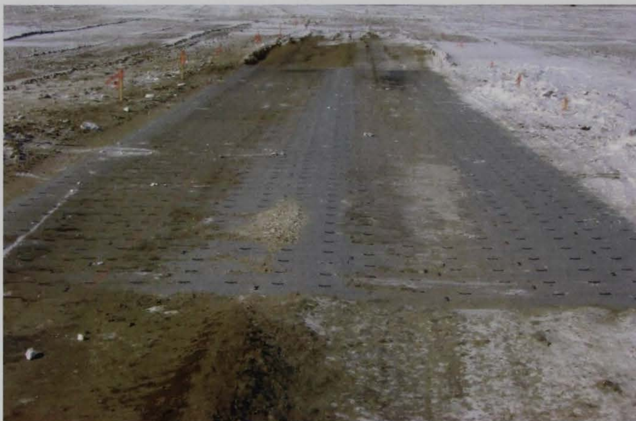
Figure 67. SC-2 test section after 2,000 passes.
