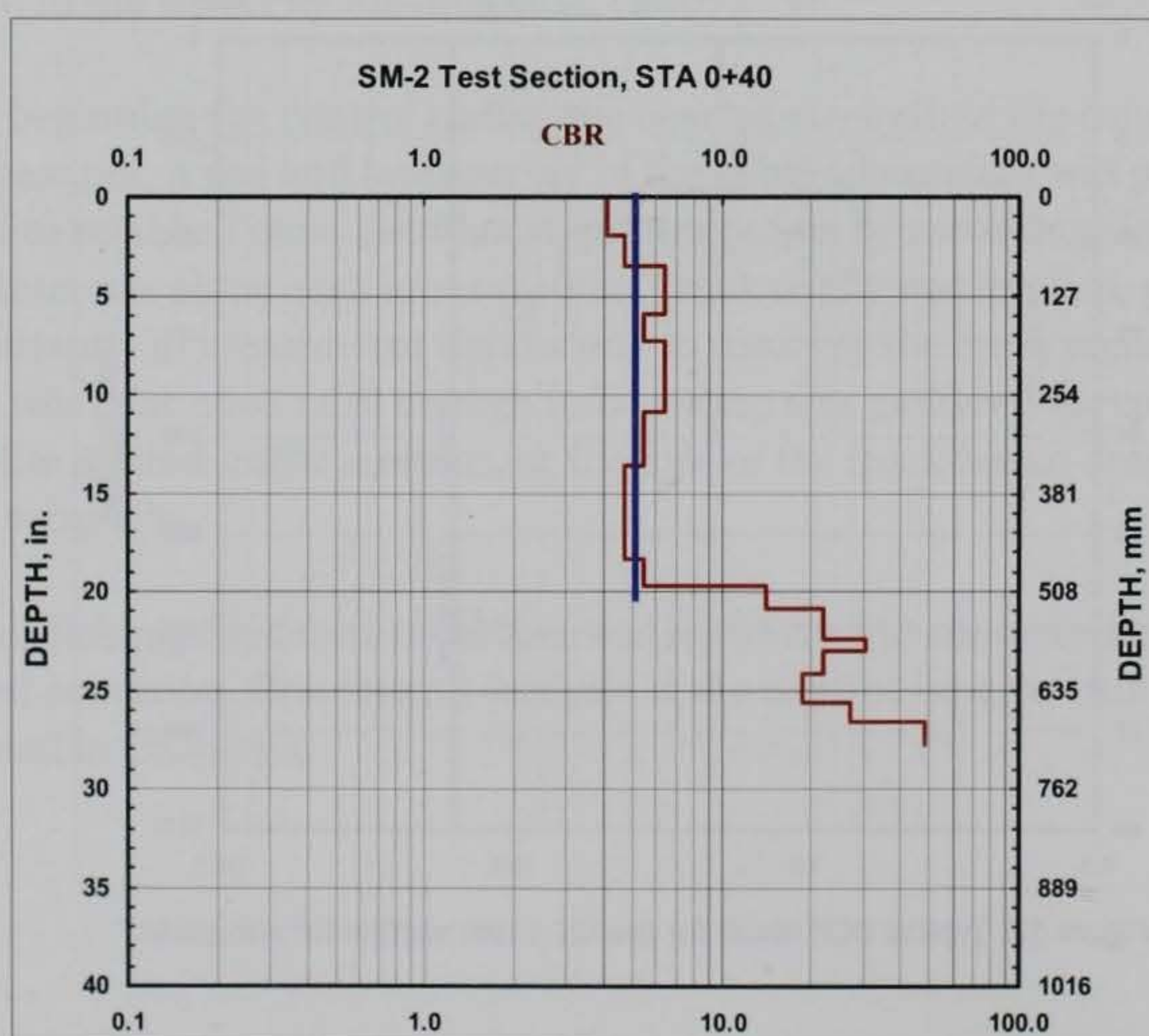
Figure 20. Typical DCP result for the SM-2 test section ML-CL subgrade.
