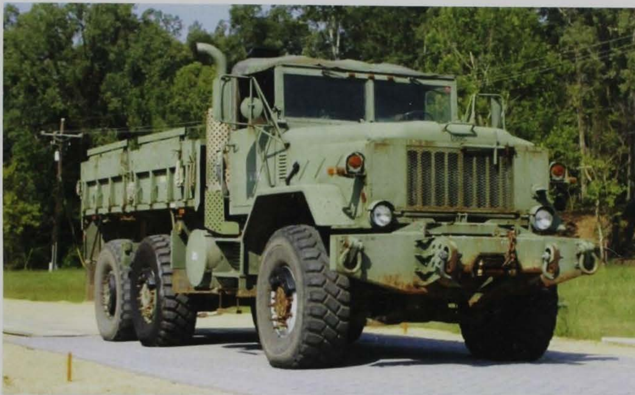
Figure 16. Seven-ton military transport truck used to traffic the mat test sections.
