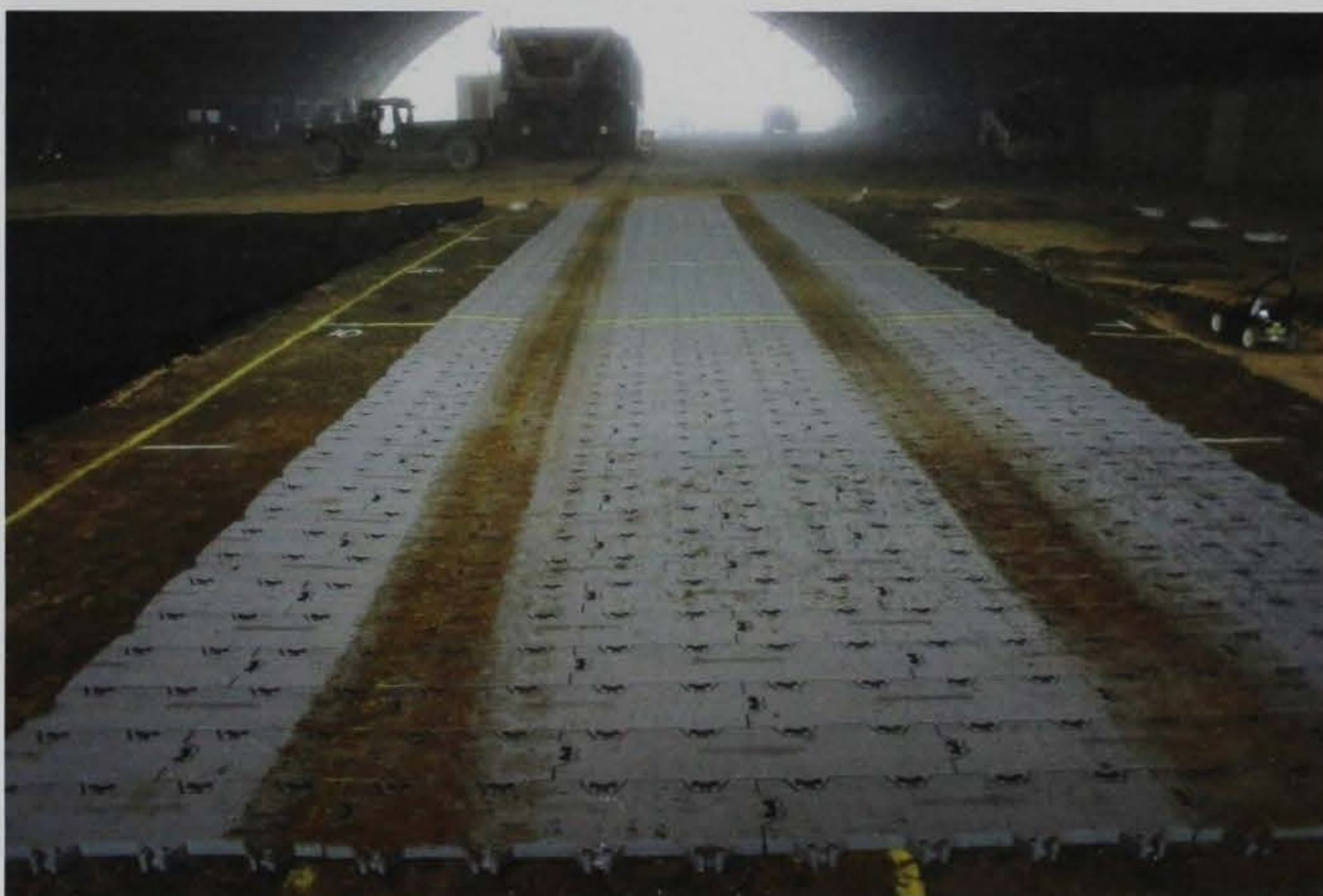
Figure 63. SM-4 test section after 2,000 passes.
