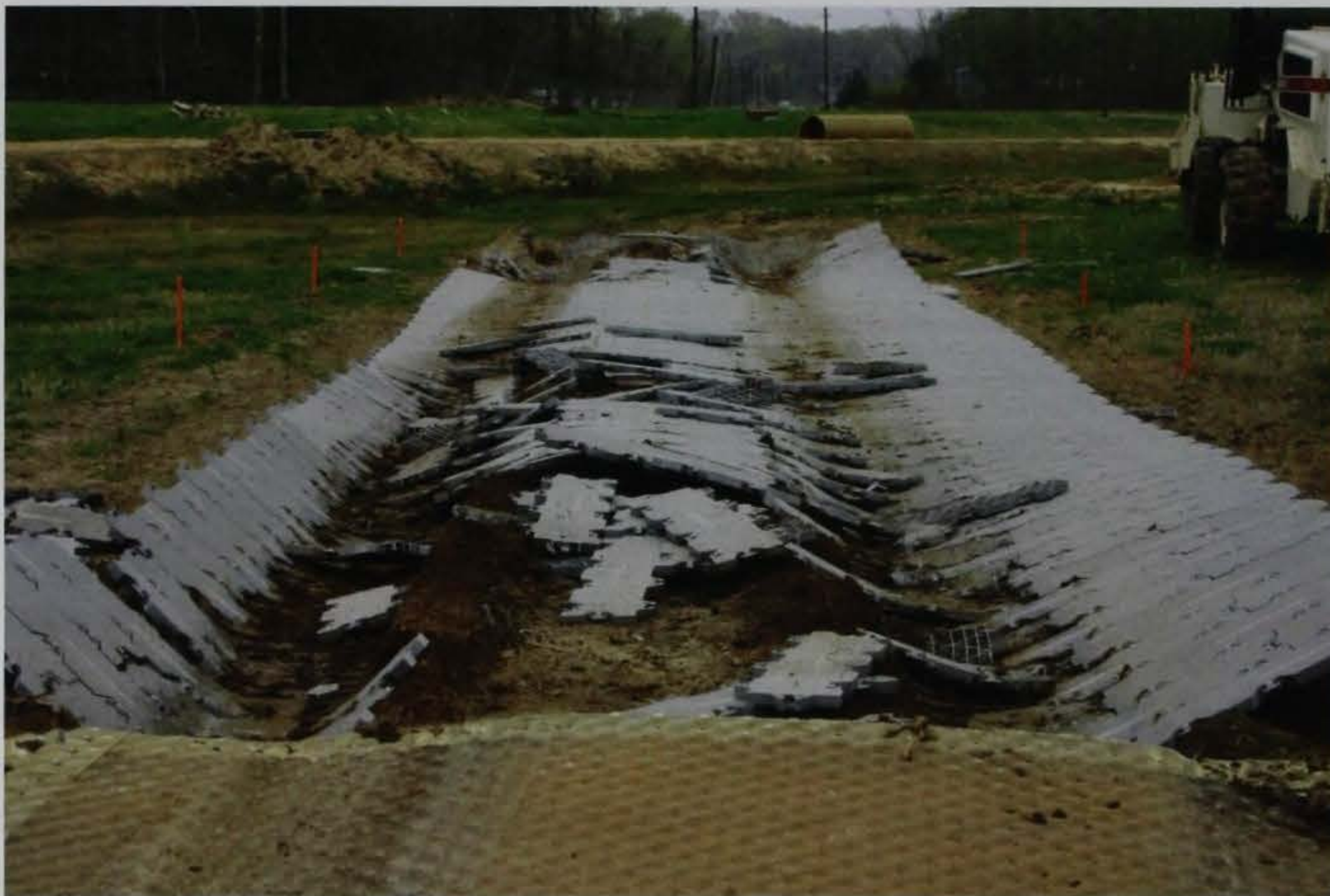
Figure 62. SM-3 test section after 140 passes.
