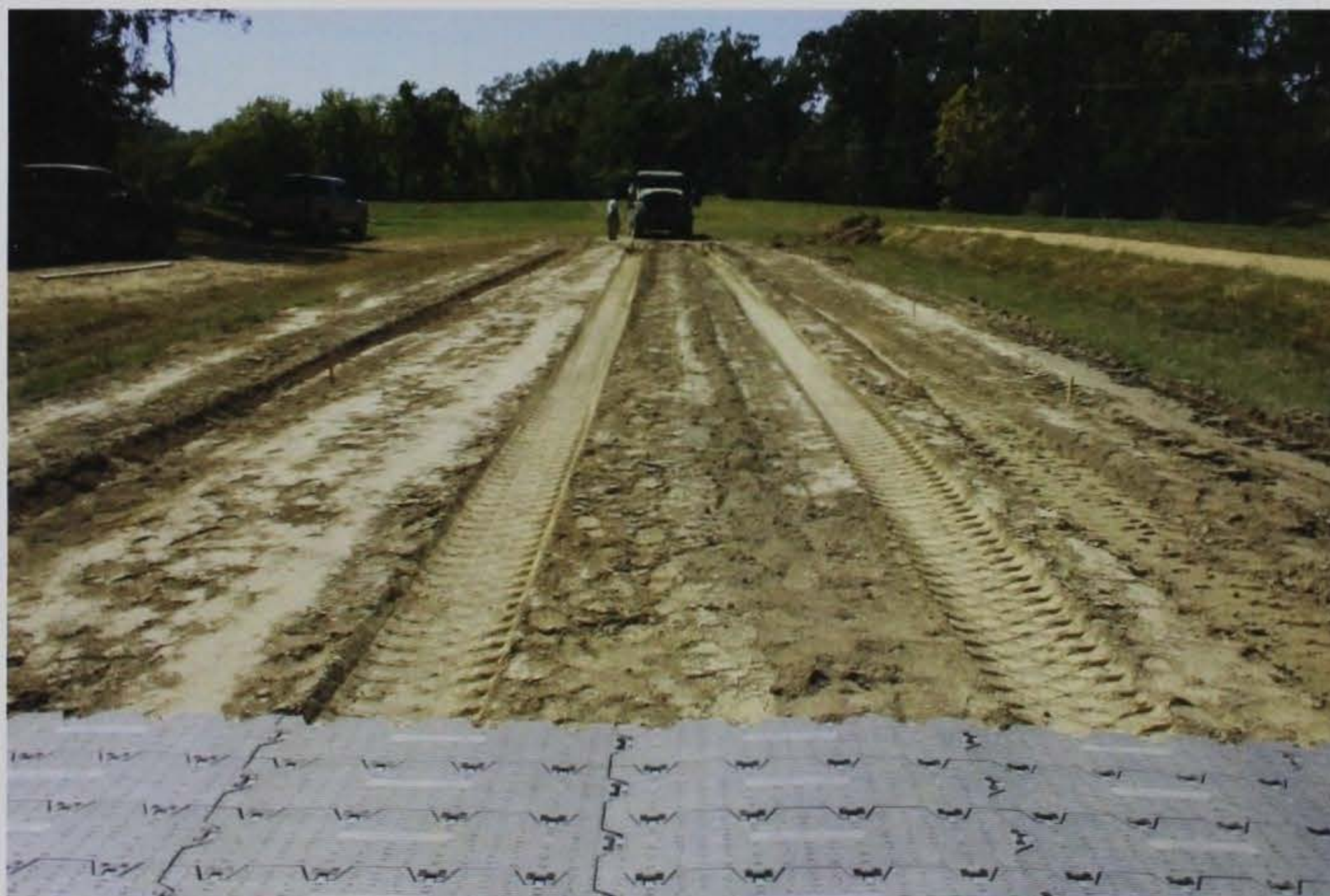
Figure 54. SM-2 control after 6 passes.
