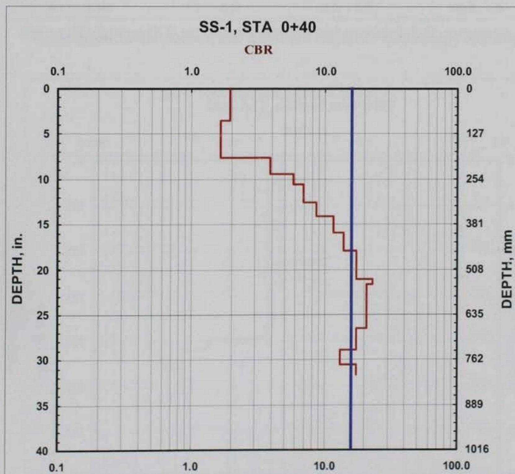
Figure 18. Typical DCP result for the SS-1 test section SP subgrade.
