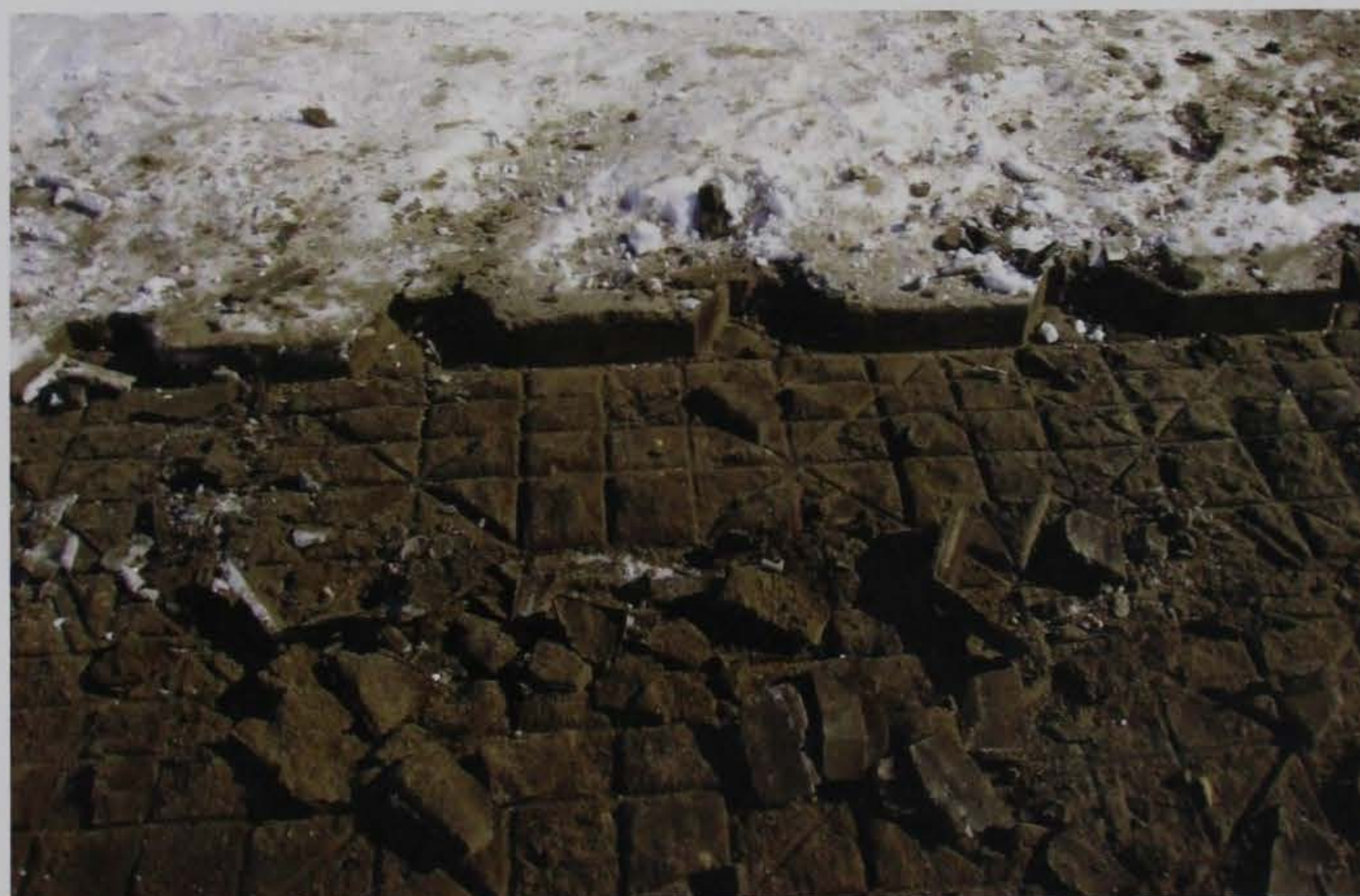
Figure 70. Frozen subgrade after removal of matting from SC-2.
