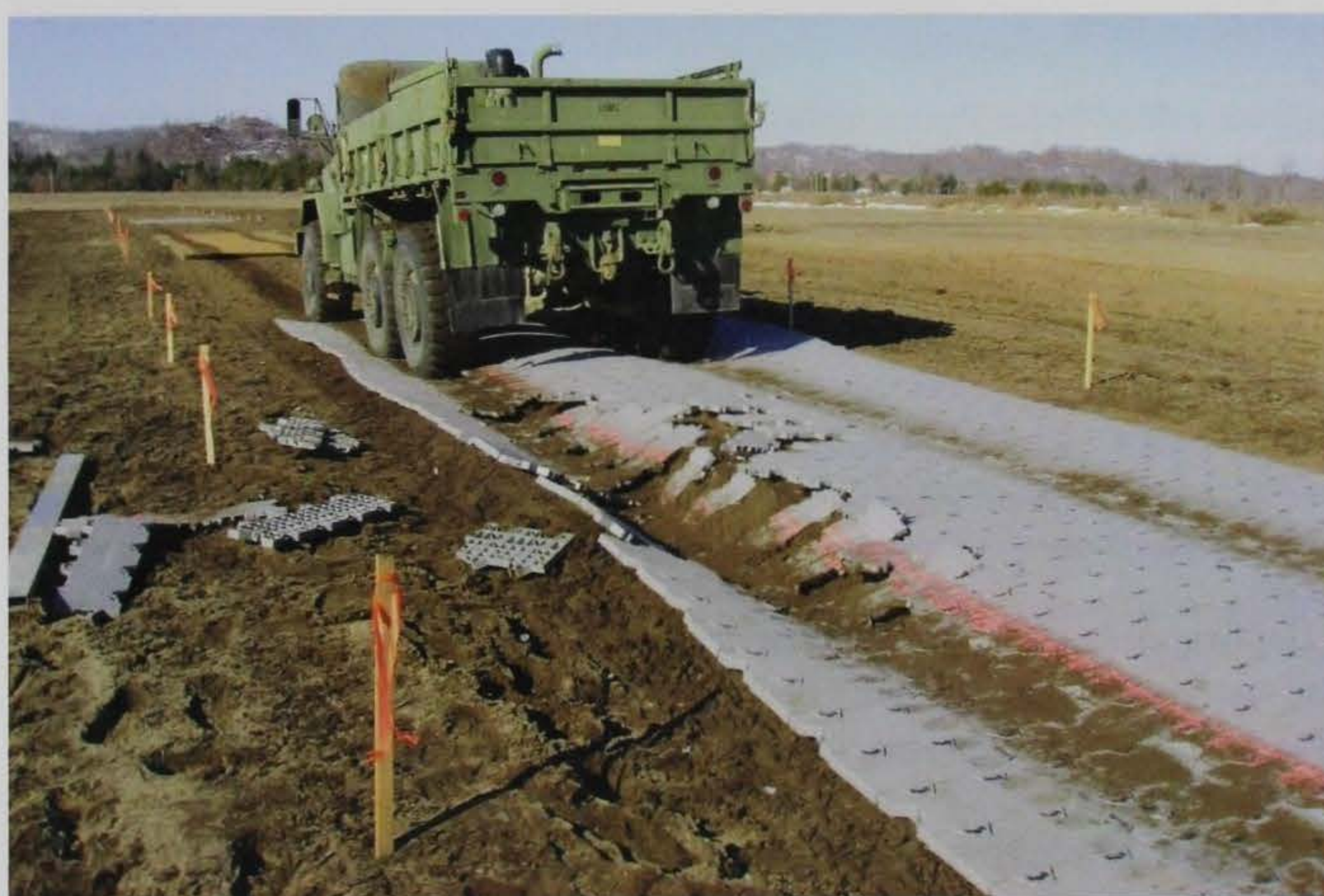
Figure 65. SC-1 test section after 120 passes.
