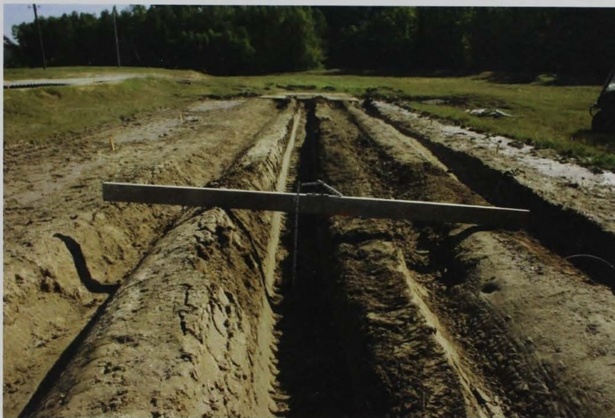
Figure 53. SM-1 control rut depth after 4 passes.
