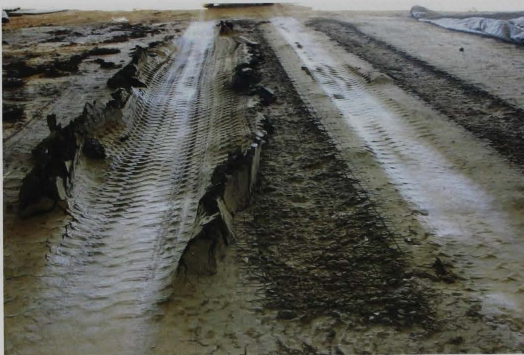
Figure 55. SM-4 control after 1,000 passes.
