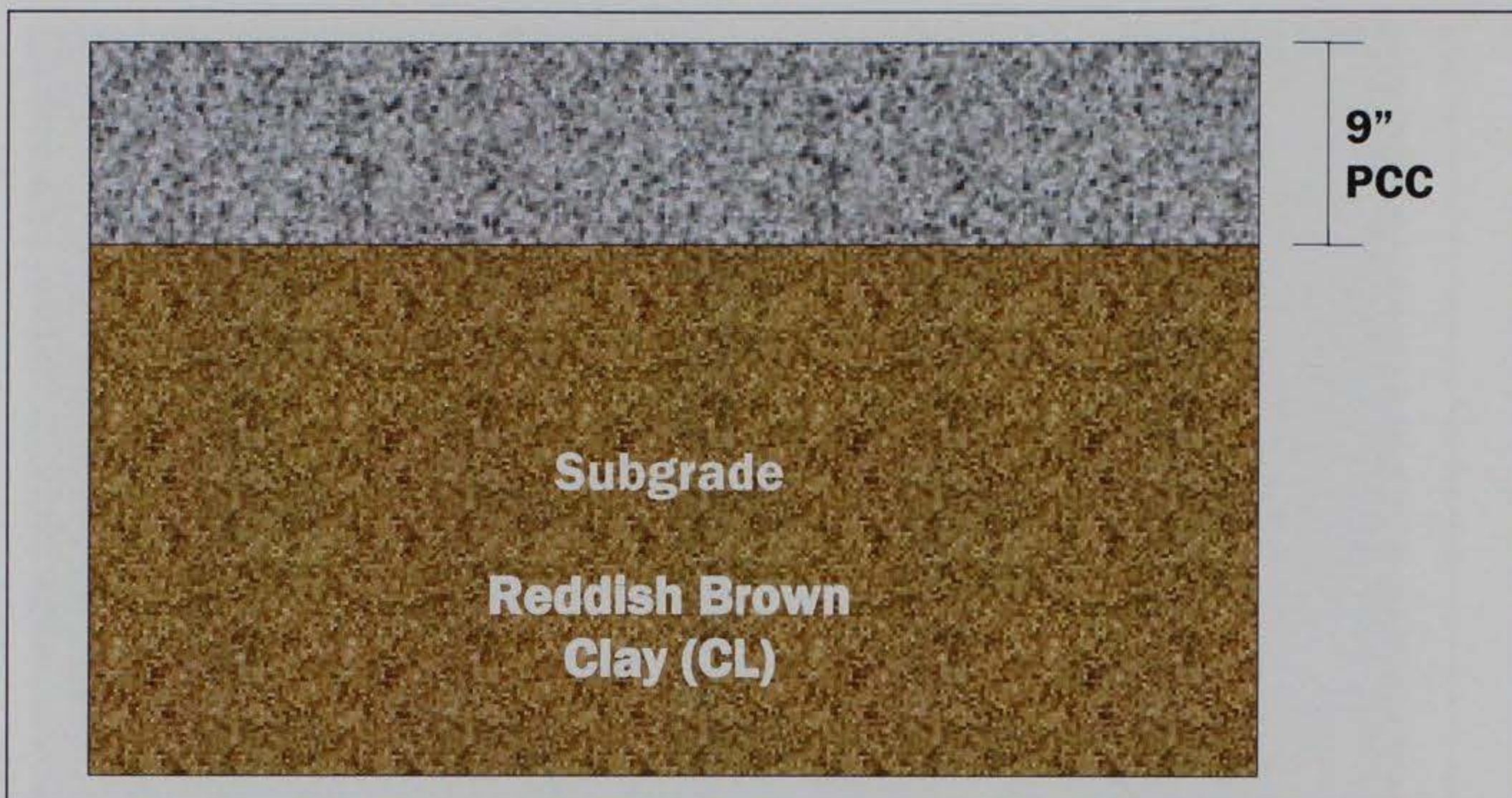
Figure 28. Pavement structure at the ALC Ramp, Tinker AFB, OK.
