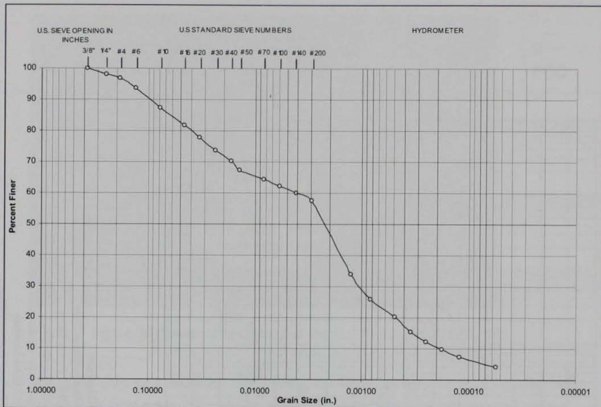
Figure 30. Gradation curve of subgrade material at Tinker AFB, OK.
