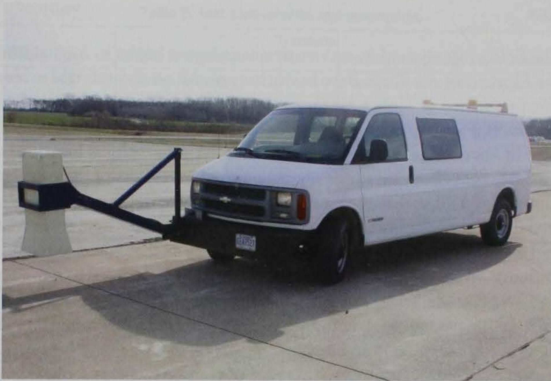
Figure 8. Ground penetrating radar van.
