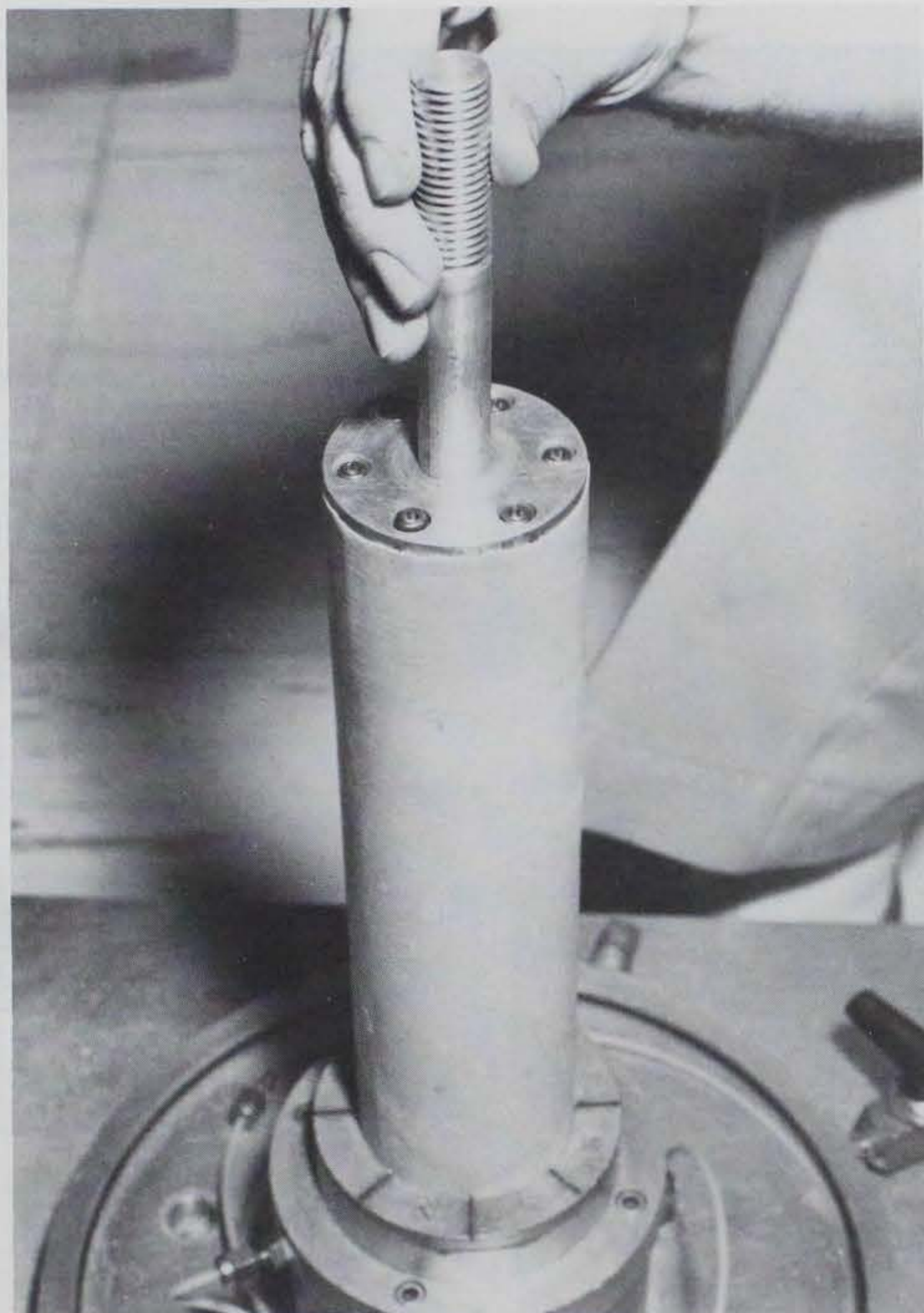
Figure 14. Fastening the lateral support rod to the chamber base
