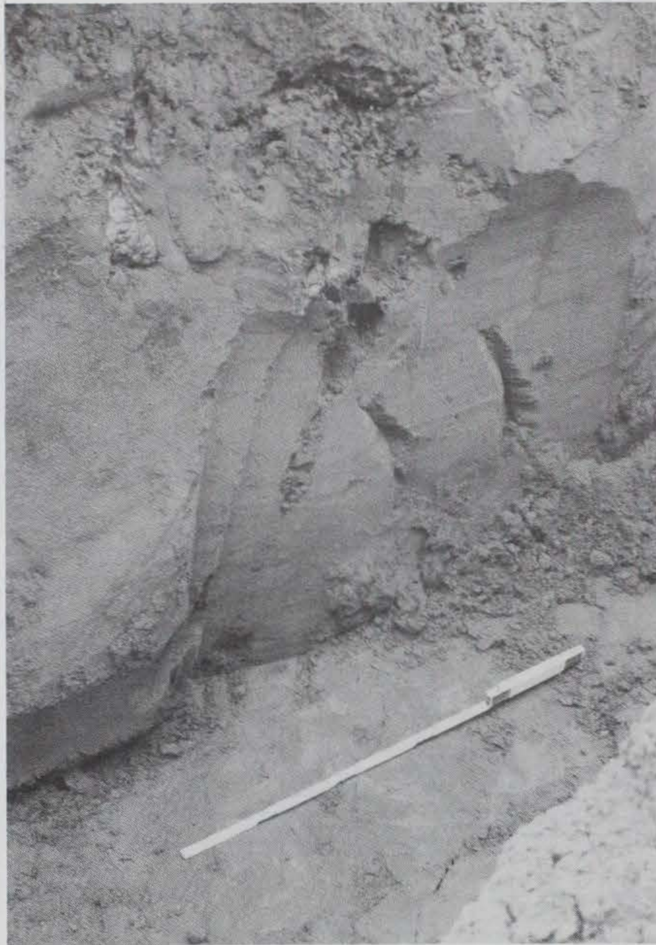
Figure 17. Top of excavated crack
