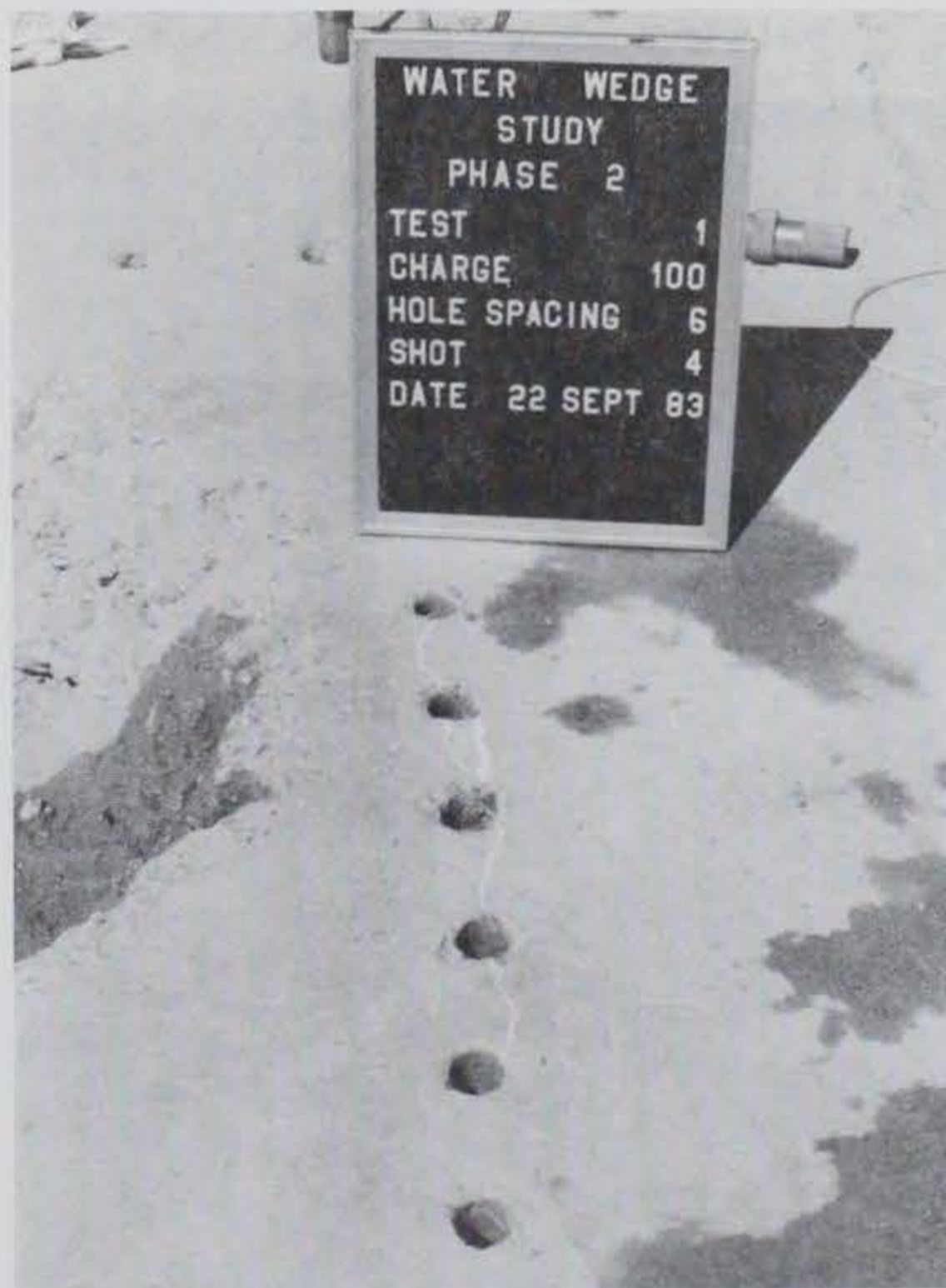
Photo 15. Extent of cracking after test 1, shot 4
