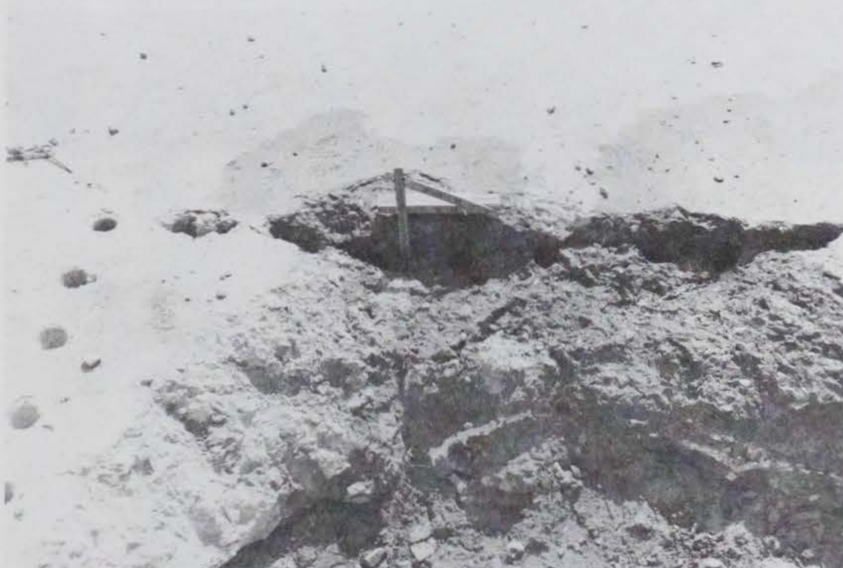
Photo 31. Extent of spalling after shot 29, test 4
