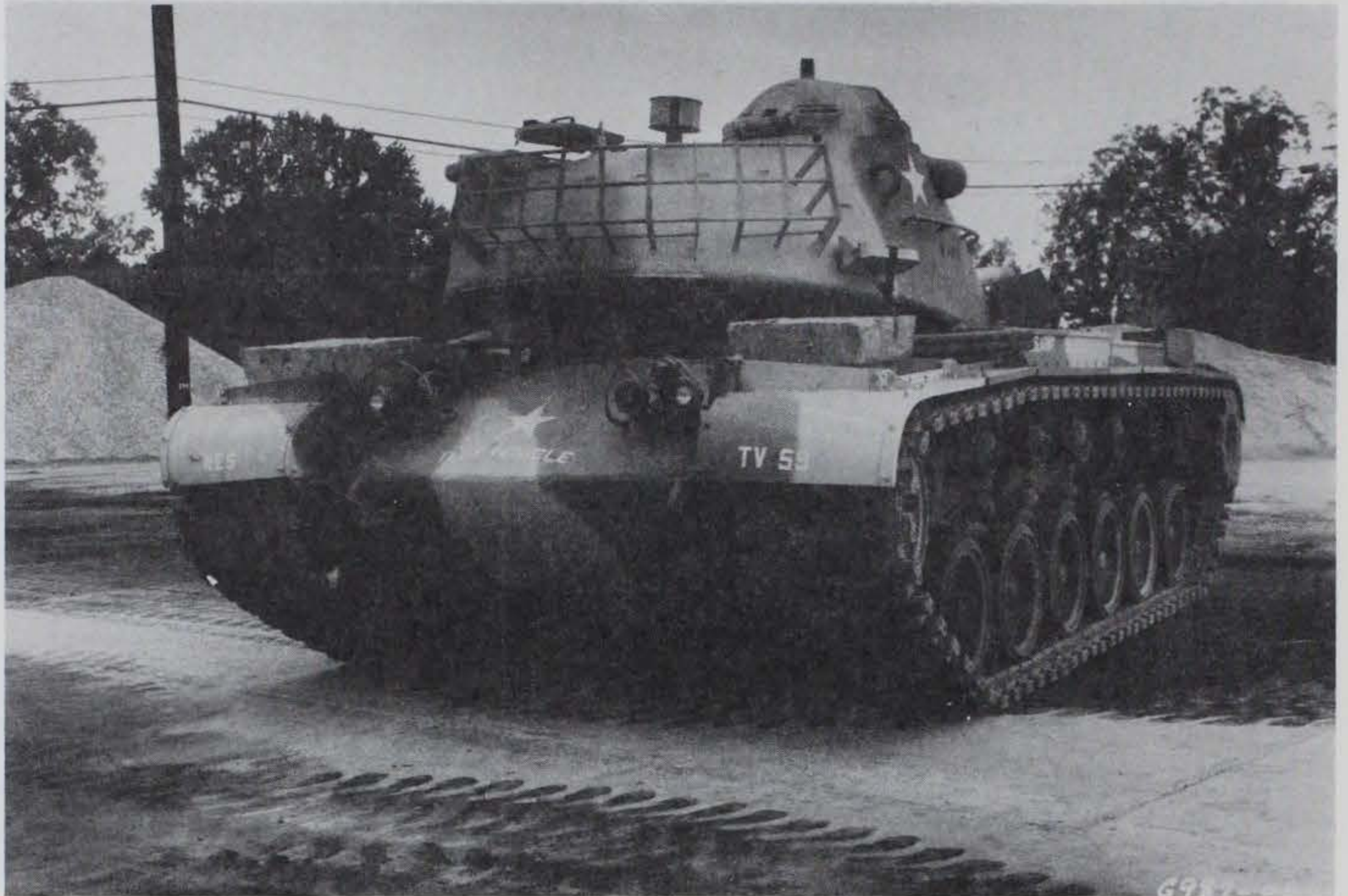
Photo 23. View of M-48 tank loaded with blocks to simulate combat weight
