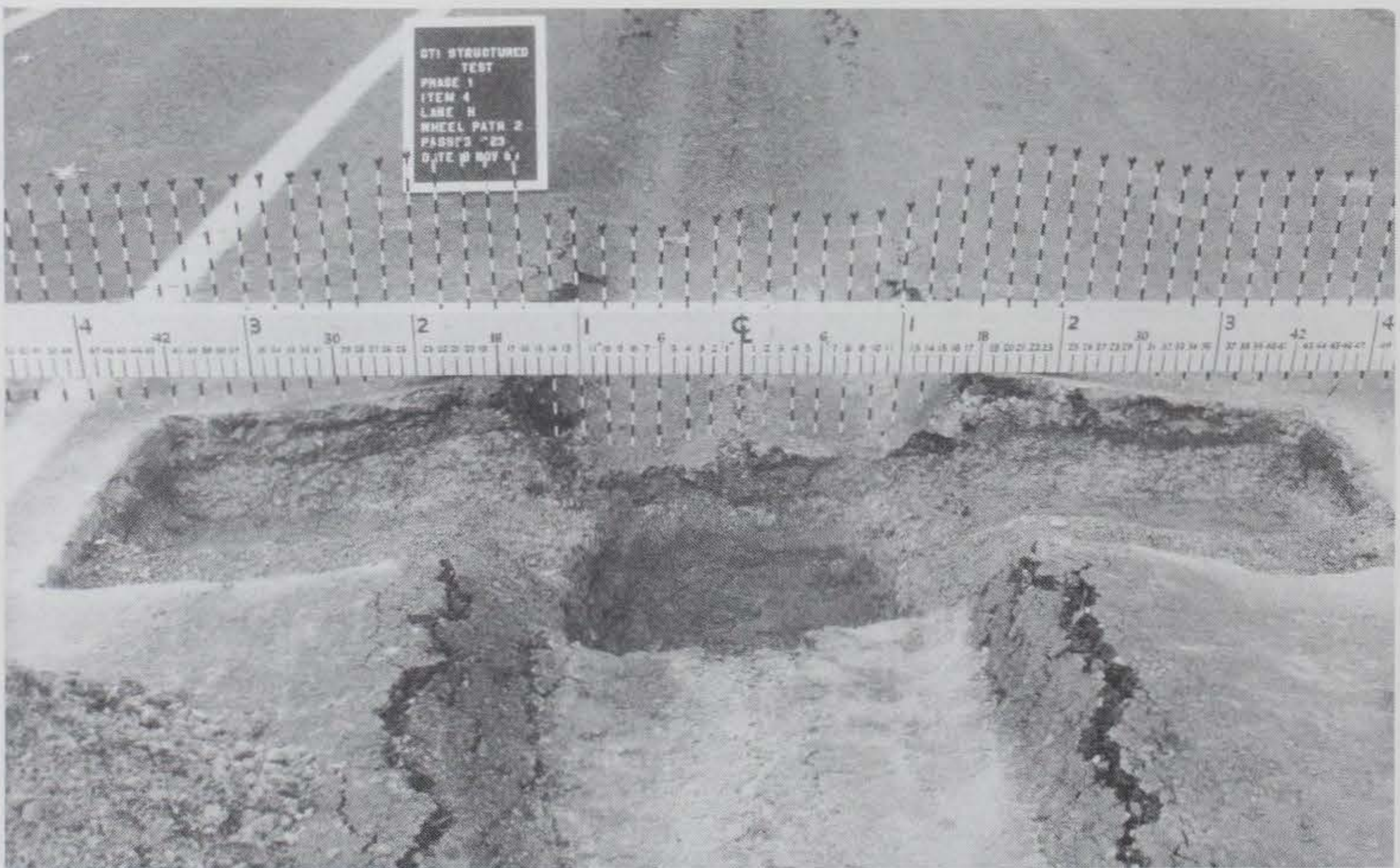
Figure 11. High-tire-pressure lane, section 4, test trench after 323 passes
