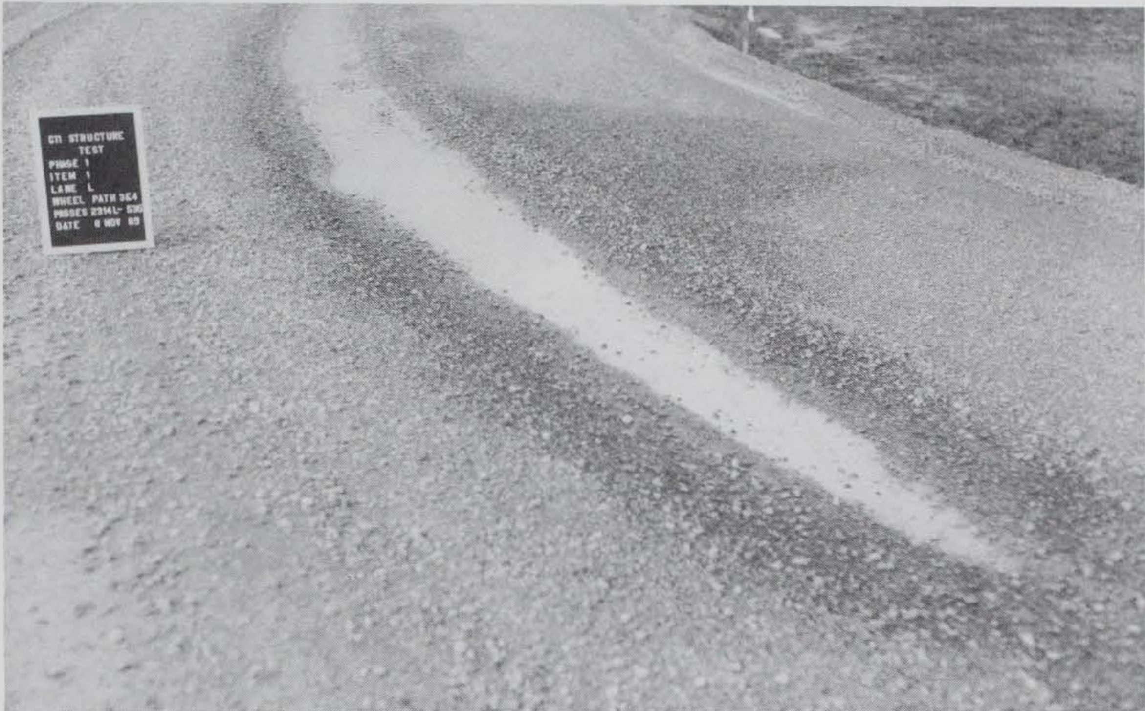
Figure 21. Low-tire-pressure lane, section 1, low-severity rutting
