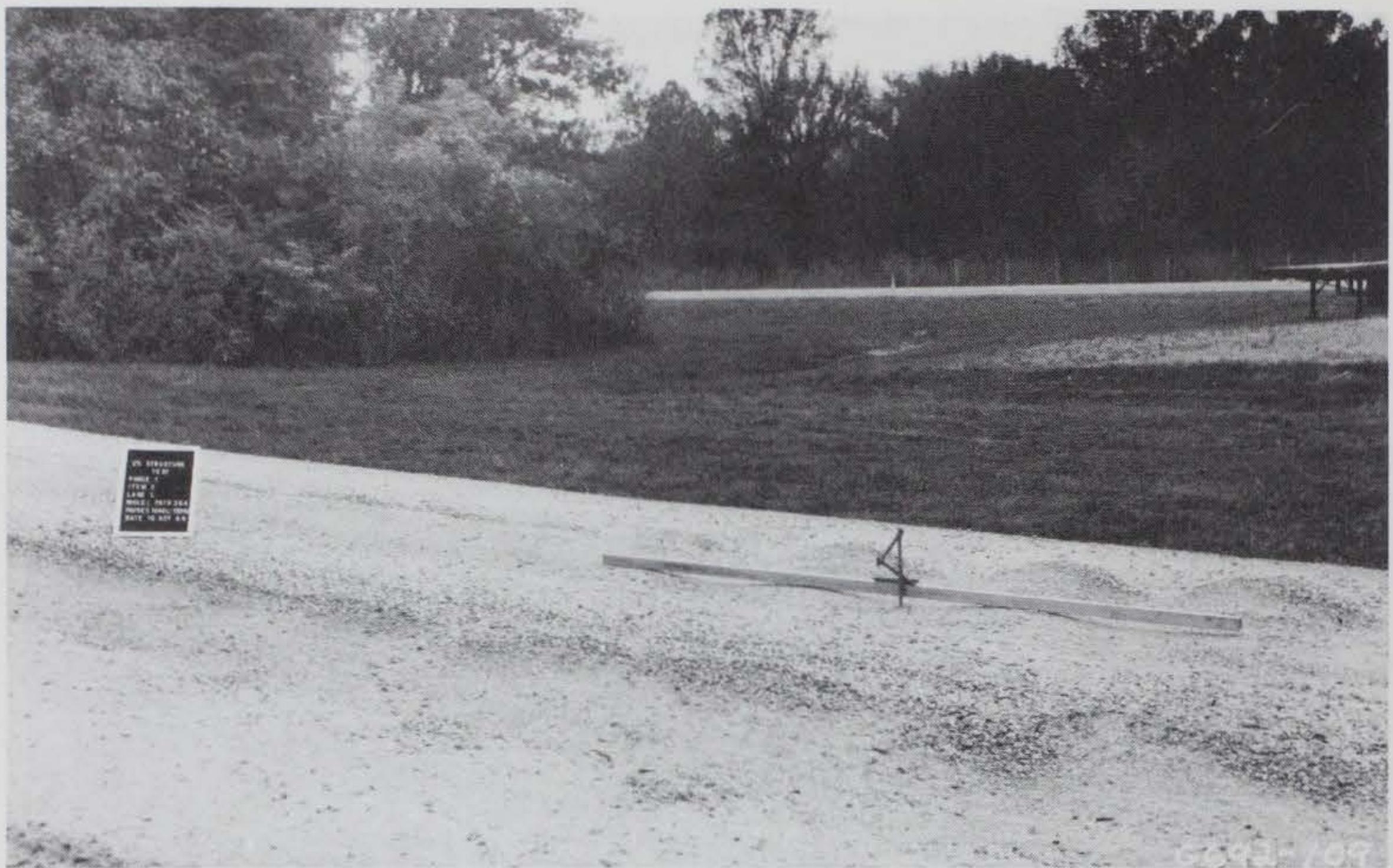
Figure 19. Low-tire-pressure lane, section 2, long intervals between corrugations
